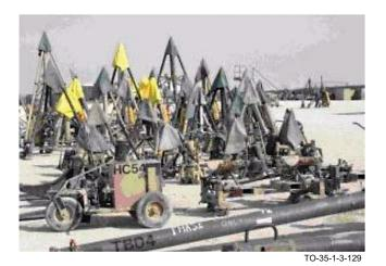
Figure 7-4. Locally Manufactured Permeable Covers
