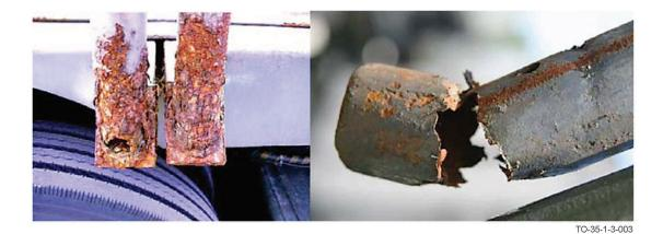
Figure 1-3. Corrosion Accelerated by Condensed Moisture
