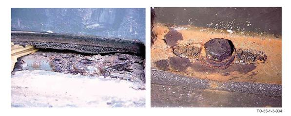
Figure 1-4. Open Cell Foam and Resulting Corrosion
