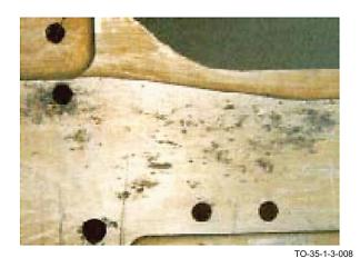
Figure 1-8. Example of Pitting Corrosion
