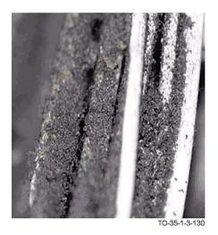
Figure 7-5. Wire Bundle Sand/Dust Accumulation
