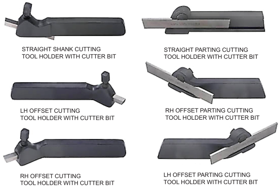
Figure 4-15. Different Types of Cutting Tool Holders
