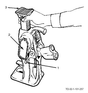
a. The operator should familiarize himself with the jack, its capabilities and its operations. The reversing lever (1) is located below the lifting mechanism cover (2) on the left side of jack when viewed from the lifting lever. When preparing to lift a load, the head (3) can be pulled up by hand to meet the load.
