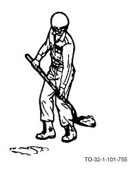
d. Slide one hand near enough to the shovel blade to raise the weight of the blade and dirt, holding the handle down with the other hand.
