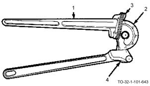
The hand tube bender consists of the following components: a handle (1), a radius block (mandrel) (2), a clip (3), and a slide bar (4). The radius block is graduated from 0 to 180 degrees, and the slide bar has a scribe mark which indicates the degree of bend. These benders are available in 3/16, 1/4, 5/16, 3/8, and 1/2 inch sizes. The hand tube bender is used to bend copper, brass, or aluminum tubing to specific angles.
