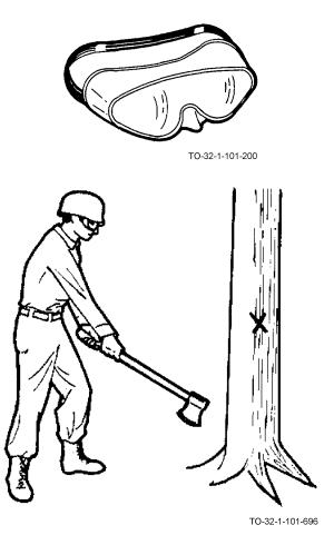
a. First clear the work area of material that might deflect the ax blade. The user's body weight should be evenly distributed, with knees set, but not tense. The feet should be spread at a comfortable distance to retain balance, while the body should be relaxed and free to swing and bend at the waist.
