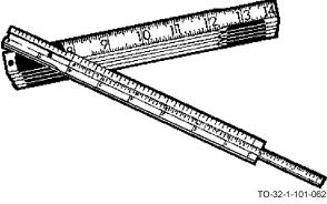
These folding rules are usually from two to six feet long. The folding rules cannot be relied on for extremely accurate measurements because a certain amount of play develops at the joints after continued use.
