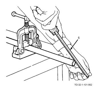
h. Remove the shoulder (the rough edge left by cutting) from the outside of the pipe with a file (5).
