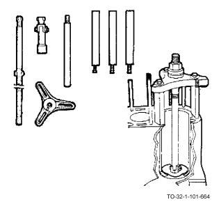
The universal cylinder sleeve is used to pull cylinder sleeves from engine blocks. It is adjustable to provide clearance regardless of the position of the cylinder studs and to simplify centering the tool over the bore. This puller is used in conjunction with four adapter plates supplied with the puller. The combination is capable of pulling cylinder sleeves 4-1/4, 4-1/2, 4-3/4, and 5-3/4 inches in diameter.
