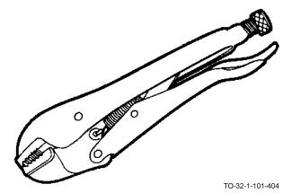
The clamp pliers are generally used more as a wrench than as a pair of pliers. It has a fixed jaw and handle which contains an adjustment screw for the movable jaw. The other handle is in two sections, one section to apply pressure and to lock the pliers, and the other section, when pulled, to release the grip. Clamp pliers are used to hold or clamp nuts and bolts which have been rounded off by using the wrong size wrench.
