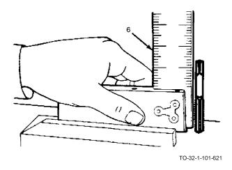
e. Remove tap wrench and, using a square (6), check tap for squareness. Check at least two different positions on the tap.
