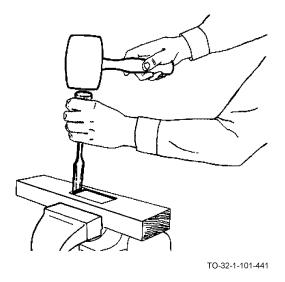
f. Remove the last 1/8 inch using chisel and mallet to complete the job.
