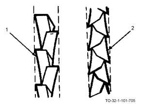
The handsaw consists of a thin flat blade with teeth and a wooden or plastic handle, called the heel, fastened to the end of the blade by screws. There are two categories of handsaws: the ripsaw (1) and the crosscut (2). The ripsaw is designed to cut with the grain of wood, and the crosscut saw is designed to cut against the grain. The handsaw is used in carpentry, roughout work, and for "finish" hand sawing. Sizes of handsaws vary depending on design and nature of the task.
