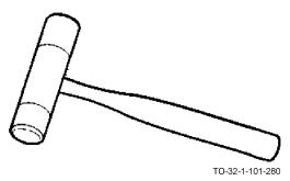
Soft-faced hammers are capable of delivering heavy blows to machined, highly polished or soft surfaces without damaging the surface. 21.2.12 Lead or Copper Hammer.
