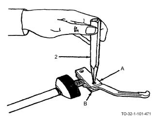
b. Insert tip of punch (2) through hole in part A using only hand pressure, and move punch and part A until you can get the tip of the punch into part B.
