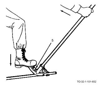
d. Place one foot on the foot rest (5) and push down with your foot while pulling back on the handle. Apply steady pressure throughout the entire bending process.
