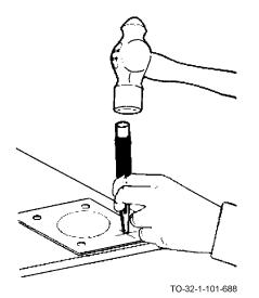
Cutting small holes in gasket with a hollow punch.
