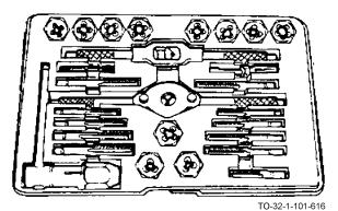
The thread cutter set is made up of a combination of taps, dies, diestocks, tap wrenches, guides, and screwdrivers and wrenches for making adjustments. Thread cutter sets are used for cutting internal and external threads.
