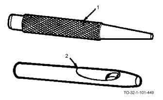
27.2.1 <u>Center Punches</u>. There are two types of center punches, both used for starting drill holes.
