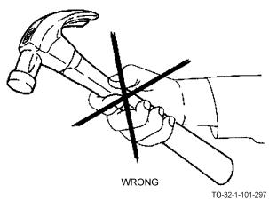
The wrist and arm motion depends on the power of the impact required. Small nails require light blows almost entirely from a wrist motion. Heavy blows, needed to drive a large nail or other similar task, come from the wrist, forearm and shoulder.
