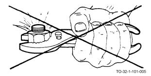
2.2.4 <u>Use Each Tool Only on the Job for Which it was Designed</u>. If you use the wrong tool to make an adjustment, the result will probably be unsatisfactory. For example, if you use a socket wrench that is too big, you will round off the corners of the wrench or nut. If this rounded wrench or nut is not replaced immediately, the safety of your equipment may be endangered in an emergency.
