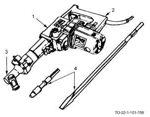
The portable electric hammer consists of a metal housing (1) with a spade or pistol-grip handle (2). A strong spring inside the housing moves a steel piston back and forth in a pounding motion. The housing muzzle (3) is designed to hold a variety of bits (4) which give the electric hammer great versatility. Examples of possible uses for this tool are beveling, caulking, pounding, digging, and breaking operations.
