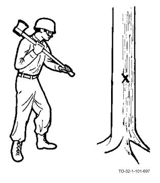
c. To start the swing, bring the ax back over the right shoulder, bending the elbow as the right hand slides up the handle toward the ax head.
