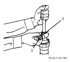
b. Insert attachment into bit retainer (2) and secure in place with locking collar (3).
