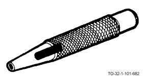
The hollow gasket cutter is also known as a hollow punch. It is extremely serviceable for cutting soft materials. It comes in a set with a mandrel. The sizes are 1/4, 5/16, 3/8, 7/16, 1/2, 9/16, and 5/8 inch. The set will withstand unlimited use if a hardwood block is used under the gasket material when cutting gaskets. They are not designed for cutting metal or cutting against a hard surface. Other individual hollow gasket cutters are also available.
