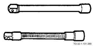
Extensions are either rigid or flexible. They range from 2 to 17 inches in length. Extensions may be used with any socket handle combination to gain clearance above nut or bolt.
