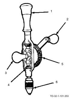
The hand drill is made up of the following parts: handle (1), drive handle (2), side handle (3), pinion (4), gear wheel (5) and chuck (6). The handle provides a storage area for drill bits. The side handle may be used to steady the drill when drilling in soft wood. The pinion turns the chuck and drill. Through mechanical linkage, the gear wheel transfers the driving force from the drive handle to the chuck. Hand drills are used to drill holes in wood and sheet metal.
