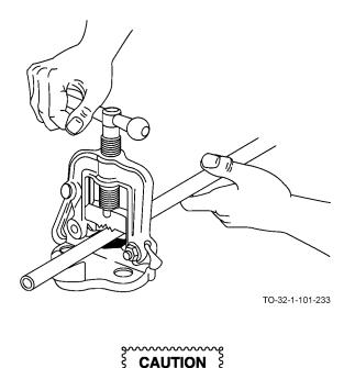
• Do not apply too much pressure to copper or aluminum pipe. Failure to comply could result in damage to, or destruction of, equipment or loss of mission effectiveness.
