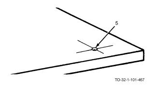
d. Remove the punch and check your mark (5). If it is not in the center of the "X" or not deep enough, you will have to repeat the procedure.
