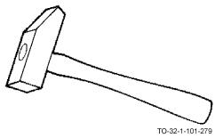
The setting hammer has a square flat face on one end of the head and a sloping beveled edge on the other end. It is used in sheet metal work for leveling and bending edges and for setting double seams.
