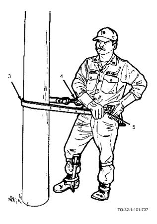
c. Snap the safety strap (3) to one D-ring (4) on the belt, pass the strap around the pole to be climbed, and snap the other end of the safety strap to the other D-ring (5).
