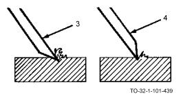
c. Rough cuts are made with bevel side down (3), while smooth finishing cuts (4) are made with bevel side up.
