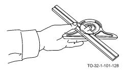
d. Remove and read measured angle on protractor scale.
