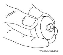
b. With the stud in the hole, check the piece for taper and out-of-roundness by sensing any wobble.
