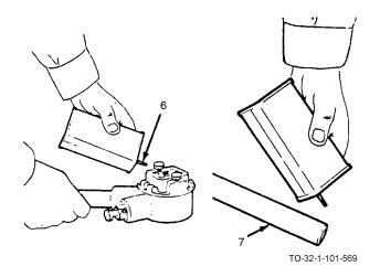
h. Apply cutting oil (6) to die and to end of pipe (7) to prevent overheating of dies and damaging of threaded surface.
