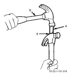
d. Drive wooden wedge (4) in handle face (5) with hammer (6).
