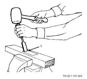
d. Start your cut about 1/8 inch from the guide line (1). Using a chisel and mallet, make your cut toward the center (the waste area) to protect the edge.
