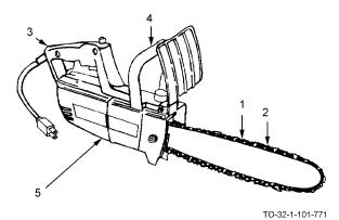
The electrically driven chain saw is a portable power saw with the teeth (1) arranged on a flexible steel chain-like belt (2). It has a pistol-like grip (3) and bar frame (4) above the motor housing (5) for holding and guiding. Unlike the gaso-line-powered chain saw, the electric chain saw is designed for lighter work such as tree trimming and cutting small logs and timber.
