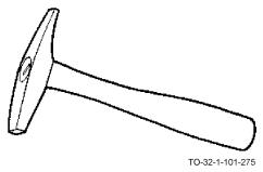
The mason's hammer has a flat striking face on one end of the head and a tapered chisel on the other end. It is used for setting and cutting bricks and flat stones.
