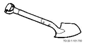
The D-handled shovel resembles the long-handled shovel except that. it has a shorter handle with a D-shaped handgrip at the end. The D-handled shovel is used for fight work or for digging in cramped, tight places.
