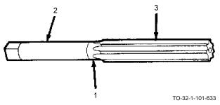
Reamers are used to enlarge and true a hole. They are also used to remove burrs from the inside diameters of pipes and drilled holes. The reamer consists of three parts, the body (1), the shank (2), and the blades (3). The shank has a square tang to allow the reamer to be held with a wrench for turning.
