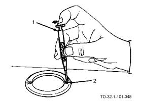
a. Hold screwdriver as shown, with forefinger on rotating head (1).
