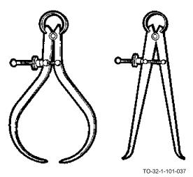
The spring-joint calipers have the same type of legs, but are joined by a strong spring hinge, screw, and adjustment nut.
