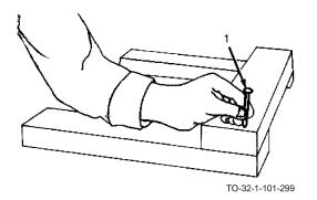
b. Support a common nail (1) between thumb and first finger about halfway up the nail.
