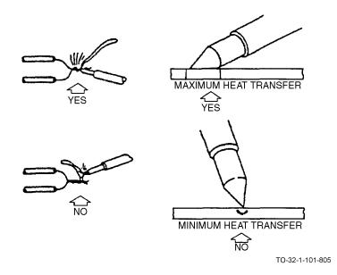
Figure 53-2. Using the Soldering Iron
