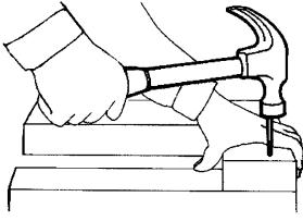
d. Remove fingers and drive nail flush. Make sure the hand supporting the work is not in direct line with the hammer blows.
