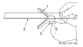
a. Slide center head (1) on rule (2) and fasten by tightening setscrew (3).
