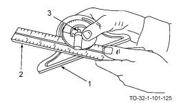
a. Slide protractor head (1) on rule (2) and fasten by tightening setscrew (3).
