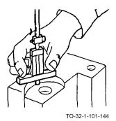
Measuring hole depth of die from a given surface.
