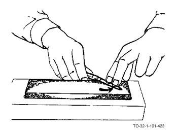
d. After several strokes, reverse the blade and stroke the other side in a similar manner. Use light, even pressure.
