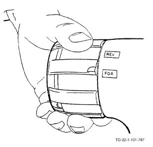
i. Set the ratchet switch in desired position for anvil rotation required. Reconnect impact wrench to power source.
