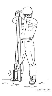
a. Drive the posthole digger into the spot where the hole is to be dug.
