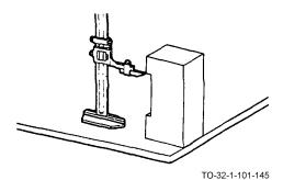
Measuring vertical distance from a plane surface.
