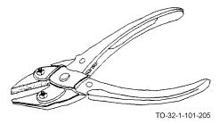
The parallel jaw pliers are constructed so that the jaws remain parallel to each other throughout the entire distance of travel. It has two jaws, a pivot pin, curved handles, and tension springs. The tension springs are contained within the curved handles and will open the jaws when the handles are released. These pliers are used to grip objects which have flat surfaces.
