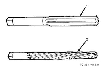
Solid taper-pin reamers are used to finish tapered holes for the insertion of tapered pins or other tapered parts. They are made with a standard taper of 1/4 inch per foot. Solid taper-pin reamers come with straight (1) or spiral flutes (2). Sizes range from 5/0 to 14, with the diameter at the large end ranging from 0.0984 to 1.5412 inches. They also come in sets of 10, sizes 3/0 to 7, and a set of 11, sizes 0 to 10. They are also included in mixed sets of straight and taper-pin reamers.
