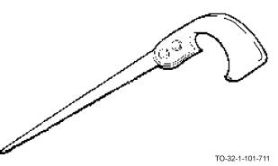
The compass saw is slightly larger than the keyhole saw. The teeth are so arranged that the blade can easily be turned for cutting curves or holes. As with the keyhole saw, the compass saw will vary in size depending on the design and purpose.
