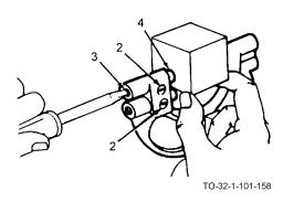
b. Loosen the locking screw (2) and turn the adjusting screws (3) until the dimensions (4) is set.
