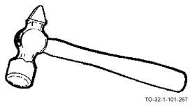
A cross peen hammer is used as a chisel for removing rivet heads and for stretching or bending metal.
