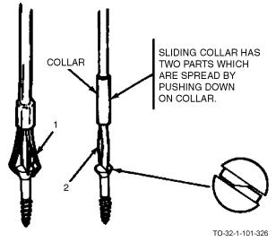
Some common screwdrivers have a screw-holding feature. These are used for working in close quarters, overhead, and hard to reach places. The two most common types are the clip (1) and sliding collar (2). After the screw has been firmly started, switch to a conventional screwdriver to complete the job.
