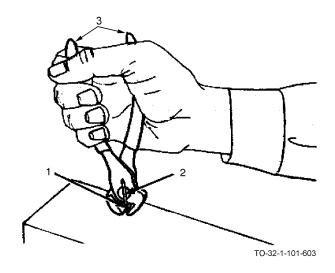
a. Place the cutting edge (1) of the nippers over the nail, wire, rivet, or bolt (2) that is to be cut flush with the surface.
