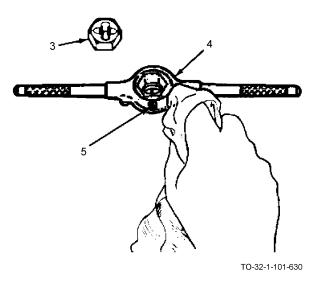
k. Disassemble die (3) and diestock (4) by loosening setscrew (5). Wipe clean with a rag.
