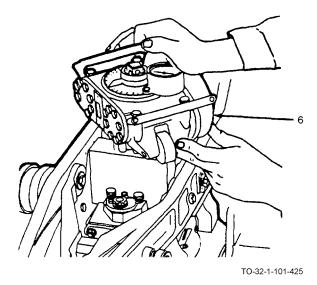
e. Install power wrench (6) onto square drive bar and reaction torque adapter. Rotate power wrench until the reaction torque adapter engages a fixed point.
