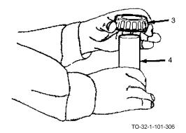
i. Unwrap bearing (3) and center over shaft (4).
