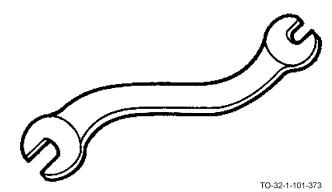
The S-Shape wrench has a 22-1/2 degree offset. It is used to reach around obstructing objects.
