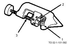
Tube cutters have a cutting blade (1), guide rollers (2), and an adjusting screw (3). Some cutters have a reaming blade
