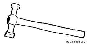
A bumping body hammer is used to straighten and form metal.
