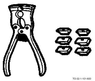
Cutting nippers are available with integral or detachable cutters. They are used to cut wire, light metal bars, bolts, nails, and to cut protruding metal flush with a surface. Some nippers have adjusting screw stops in the handle and adjustable jaws. Others have detachable jaws with compound leverage and come with three extra pairs of jaws. Cutting nippers range in size from 5-1/2 to 15 inches long and up to 1-3/4 inches in jaw widths.
