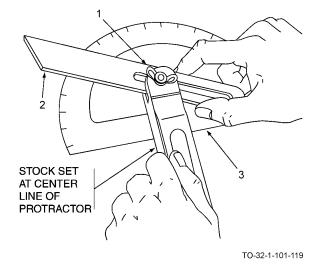
a. Loosen locking nut (1) and adjust blade (2) to measure a desired angle using protractor (3). Tighten locking nut (1).
