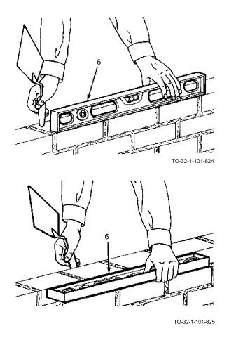
j. Lay enough bricks to cover the mortar bed and tap into line using a builder's level (6).
