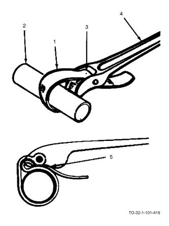
a. Loop the strap (1) around the pipe (2) in the opposite direction to that in which the pipe is to be rotated.
