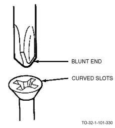
The tip of a cross-tip screwdriver is shaped like a cross so that it fits into cross-tip screws. Cross-tip screws have two slots which cross at the center. These screwdrivers are made with four different sized tips. Cross-tip screwdrivers also have different length blades ranging from 1 inch to 8 inches.
