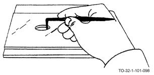
The bent point is used to scribe through holes or other hard to reach places.
