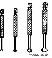
Small hole gages are adjustable, having a rounded measuring member. A knurled screw in the end of the handle is turned
