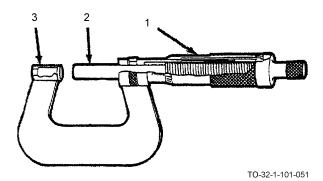
Reading a micrometer is only a matter of reading the micrometer scale or counting the revolutions of the thimble and adding to this any fraction of a revolution. The micrometer screw has 40 threads per inch. This means that one complete and exact revolution of the micrometer screw (1) moves the spindle (2) away from or toward the anvil (3) exactly 1/40 or 0.025 inch.
