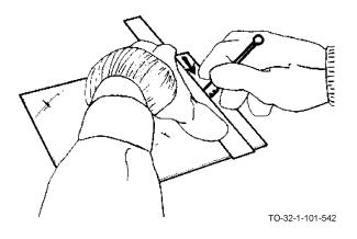
f. Start your cut at the far end of the pane of glass drawing the cutter toward you. It is important that you maintain proper pressure throughout the cut. Correct pressure is indicated by a scratching sound. Too much pressure or a dull wheel will produce a crunching sound. Make a continuous mark from one edge to the other edge.
