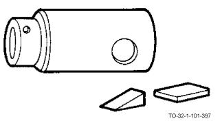
Wedge-type stud removers are made of a socket housing and two metal wedges. The socket is placed over the stud to be removed and the wedges are driven into the socket to hold the stud. The socket housing is now turned with a handle to remove the stud.
