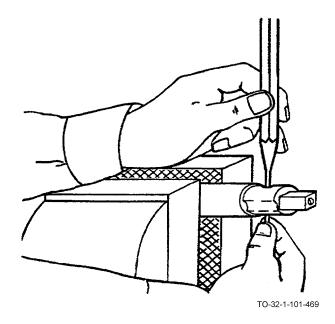
c. Catch the pin before it falls out of the shaft. When the pin is about half way out of the shaft, you can let go of the punch.
