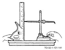
Setting gage for transfer of 4 inch vertical measurement.
