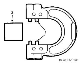
a. Position gage so that the pins or buttons (1) are square with the flat surfaces on the part (2).
