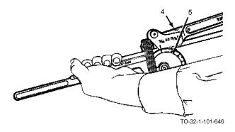
c. Lower slide bar. The zero mark (4) on the slide bar should match up with the zero mark on the block (5).
