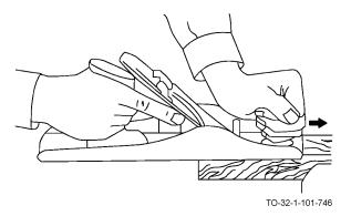
d. Check to insure the plane is placed on the work so that the wood grain points in the direction the plane will go.
