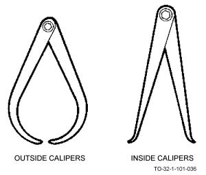
The simple outside calipers are bowlegged. Those used for inside diameters have straight legs with feet turned outward. Calipers are adjusted by pulling or pushing the legs to open or close them.
