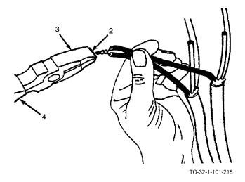
b. Grasp the ends of the wires (2) firmly on the serrated jaws (3) and twist the pliers (4).
