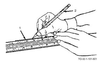
a. Place the wire (1) on the table. Measure the section to be cut off. Mark it with pencil, chalk, soapstone or other suitable marking piece (2).
