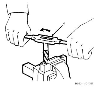
c. Remove the broken screw by turning the extractor counterclockwise. The extractor may be turned using a tap wrench or open end wrench (4).
