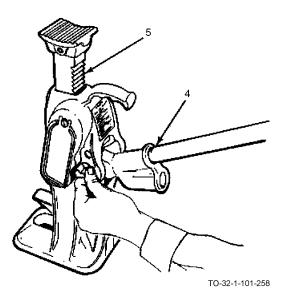
b. To raise a load, pull reversing lever up and toward the operator and operate the lever (4). The jack will raise the load one notch for each lever downstroke. The rack (5) cannot be ratcheted out of the base, as it is designed to stop when raised to its top limit.
