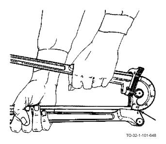
e. Stop bending the tubing when the zero mark on the slide bar matches the desired angle (6) on the block.
