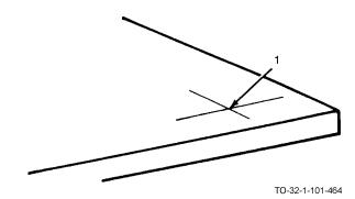
a. Mark the material to be punched with an "X" (1).
