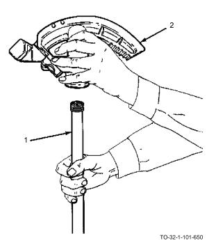
a. Install handle (1) on bender (2). A section of threaded pipe may be used as a handle.
