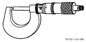
Outside micrometers are used to measure an outside distance or diameter to an accuracy of 0.001 of an inch.
