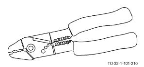
Wire strippers are used to strip insulation from electrical cord. When closed around wire, only the insulation is cut. The wire core remains undamaged.
