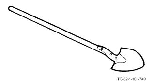
The long-handled shovel consists of a curved, shaped steel blade attached to a long wooden handle. The lower metal edge of the blade is tapered to help it cut into the ground. The longhandled shovel is used for heavy digging, especially when it is necessary to throw or move dirt a substantial distance.
