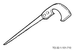
The keyhole saw is the smallest type of nested saw. Its blade has a very narrow point small enough to enter a 1/4 inch hole. It is used for close-quarter work, such as cutting, shaping, or enlarging holes in a board.
