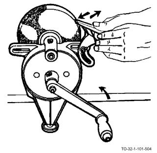
f. Rotate the handcrank and move the tool forward until it makes contact with the wheel.
