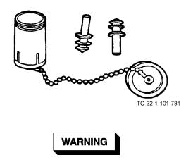
The electric hammer produces hazardous noise levels when in operation. Always wear proper protection to avoid possible hearing loss.
