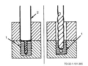
a. Drill a hole in the broken screw (1). Use a drill size guide (2) if available. If one is not available, drill the hole slightly smaller than the diameter of the extractor. (When drilling larger screws it may be necessary to drill a small pilot hole first, then a larger hole).
