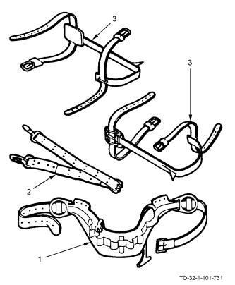
Climbing tools consist of safety belts (1), safety straps (2), and leg irons with spurs (3). Climbing tools are used for scaling poles and trees, erecting power lines, and for support when clearing and topping trees.
