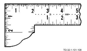
The octagon or eight square scale is used for cutting an octagon from a square piece of material. The back side contains
