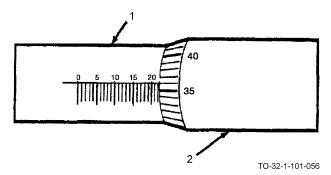
The barrel (1) is graduated in millimeters from 0 to 25. It takes two revolutions of the spindle to move the barrel 1 mm. The thimble (2) is graduated in 56 divisions with every fifth line being numbered. Rotating the thimble from one graduation to the next moves the spindle 1/50 of 0.5 mm, or 1/100 mm. Two graduations equal 2/100 mm, and so forth.
