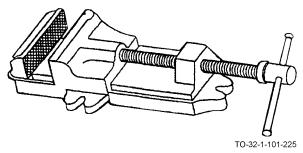
The machine table vise is a special purpose vise which may be bolted to a drill press, lathe, or table. It is available in two sizes, one having a 3-1/2 inch jaw width and a 3 inch jaw opening, and the other having a 6 inch jaw width and a 6 inch jaw opening. Machine table vises are used to hold small pieces of wood or metal for machining or drilling operations.
