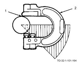
a. Locate the gage on the part with the solid anvil (1) on top. Rock the gage (2) as indicated by the shaded segment above, where the GO dimension is checked.
