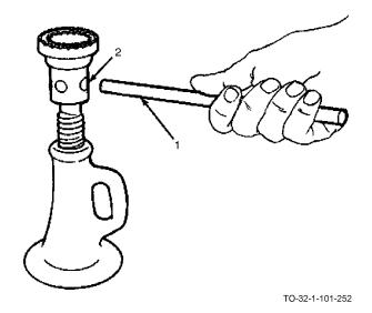
a. Insert the handle or bar (1) in the hole in the top housing or head (2).
