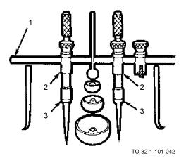
The trammel measures distances beyond the range of calipers. The instrument consists of a rod or beam (1) to which trams (2) are clamped. The trams (2) carry chucks (3). The trammel can also be used as a divider by changing the points.
