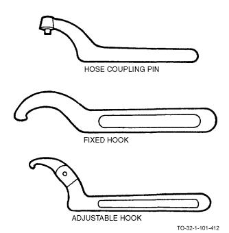
Three kinds of hook-type wrenches include the hose coupling pin, for tightening and loosening hose couplings, the fixed hook, for tightening or loosening couplings with protruding rims or edges, and the adjustable hook-type. The adjustable hook-type is similar to the fixed hook-type. However, it may be adjusted around objects and fastened before use.
