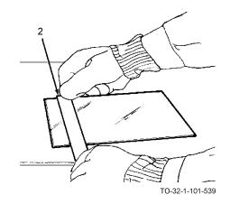
c. Place a straight edge (2) along line to be cut. A wooden yardstick should be used when available, since wood will not slip easily on glass. The cutter will cut 1/16 inch from your mark, so adjust your guide before cutting.
