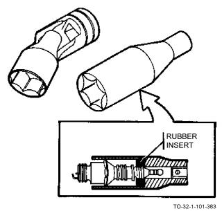
A universal joint socket and spark plug socket are examples of specially designed sockets. The universal joint socket is used When it is necessary to reach around an object. The spark plug socket has a rubber insert. This insert protects the ceramic insulator when removing and/or installing the spark plug. All sockets must be used with some type of handle.
