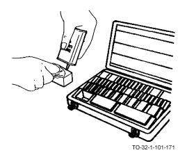
a. Observe particular care when using gage blocks to measure hardened work. The danger of scratching is increased when the work is as hard as the block, or harder.
