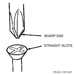
Cross-point screwdrivers are similar to the cross-tip. The cross-point slots meet at an exact right at angle at their intersection. These screwdrivers are issued in 3 to 8 inch sizes.
