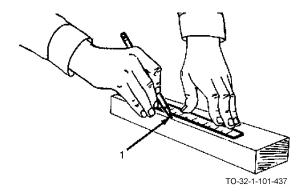
a. With rule and pencil, mark area (1) to be cut with the chisel.
