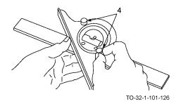
b. Loosen the protractor adjustment screws (4) so the protractor may be pivoted about the rule. Angle being measured is already marked.
