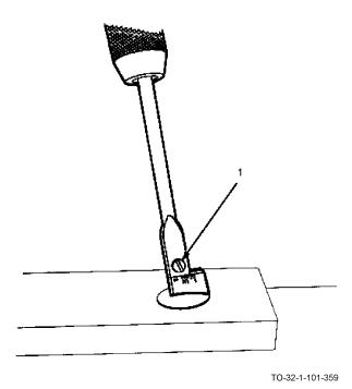
b. Tighten retaining screw (1) and refer to Drill, Paragraph 23.3, Step a through Step e.
