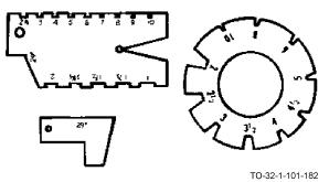
Thread cutting tool gages are hardened steel plates with cutouts around the perimeter. Each cutout is marked with a number that represents the number of threads per inch. These gages provide a standard for thread cutting tools. They have an enclosed angle of 29 degrees and include a 29 degree setting tool. One gage furnishes the correct form for square threads and the other for Acme standard threads.
