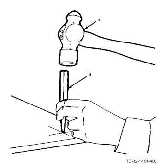
c. Position the punch upright and strike the blunt end (3) of the punch with a hammer (4).
