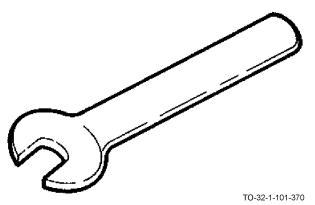
The engineers single open-end wrench has a long smooth shank providing the user with a better gripping surface. It is used to reach behind or below blind surfaces.
