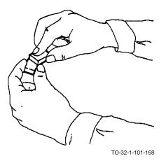
a. Bring the blocks together flat and move them slightly back and forth. This minimizes scratching, as it will detect any foreign particles between the surfaces.
