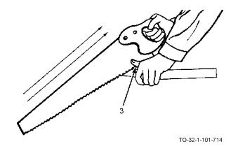
a. In using the crosscut saw, place the work on a level just below the knees. Place one sawhorse, bench or other support (1) fairly close to line of cut (2).
