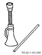
The vertical bell base screw jack is operated by hand using a steel bar handle which is inserted in the holes of the top
