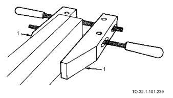
a. Open the clamp jaws (1) and place the work between the jaws. Keep jaws parallel. Use rawhide or soft leather to protect highly polished surface.
