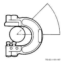
d. If the gage can be rocked further to the position, as shown, the part diameter is too small, since it has passed the NO GO button.
