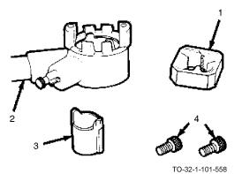
The pipe threading set contains an assortment of cutting dies (1), a handle or wrench (2), a collar (3) and locking screws (4). The cutting dies may range from 1/8 inch to 2 inches in diameter. The threading set is used to cut American Standard Pipe threads on steel, brass, copper, wrought iron, and lead pipe.
