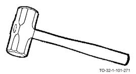
The club hammer is a heavy double-faced demolition hammer. It is primarily used to break up masonry.
