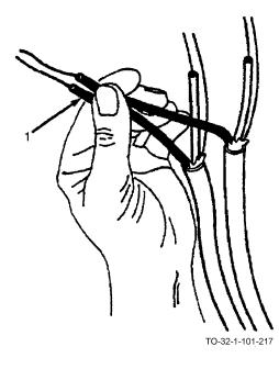
a. Using one hand, hold wires to be twisted (1) just above the point where the twist is to begin.
