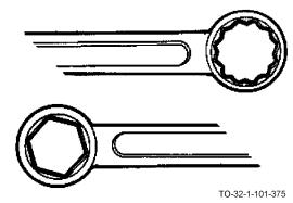
A box wrench surrounds the nut, bolt head, or stud on all sides. It is available with both 6 point and 12 point openings.
