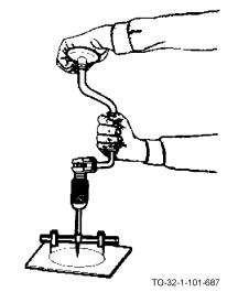
Cutting smaller circular gasket with a bit brace.
