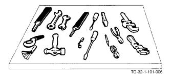
2.2.5 <u>Keep Your Tools Within Easy Reach and Where They Cannot Fall on the Floor or on Machinery</u>. Avoid placing tools anywhere above machinery or electrical apparatus. Serious damage will result if the tool falls into the machinery after the equipment is turned on or running.
