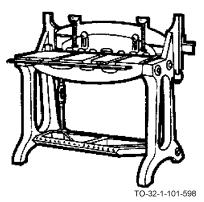
The metal shearing machine is foot-operated and is used to cut original sheets into smaller, usable size stock. The shear blade is 36 inches long and will cut all sheet metal up to and including 1/16 inch of mild steel or 1/8 inch of iron.
