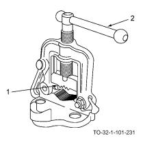
a. Open the pipe-holding jaws (1) by turning the threaded T-handle (2).
