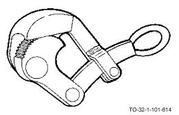
The cable jaw grip is used to tighten or stretch wires or cables for various operations. Examples of application include removing kinks or bends in cables, tightening cables on loads or bales, or for cleaning and oiling of cables. Cable grips, depending on their application, vary in size and design.
