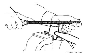
d. File edges of copper, lead or plastic mallets down to the original shape.
