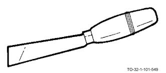
Saddler's knives are used on leather and come in different shapes. One has a broad point on a 1-1/8 inch by 5 inch blade. One has a 5/8 inch by 3-7/8 inch square point blade. Another has a 5 inch rounded-end blade. Shoe knives are similar to saddler's knives, but usually they have a 3/4 inch by 3-1/4 inch blade.
