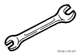
The engineer's double open-end wrench has different size openings on each end. This type of an arrangement permits a smaller number of wrenches to complete a set. The engineer's double open-end wrench is also used to reach behind or below blind surfaces.
