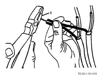
d. Open plier jaws and place the ends of the twisted wires between the cutting edges (5). Trim the ends of the wire.
