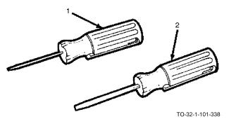
A radio screwdriver (1) has a round blade that is 1-1/2 inches long. Its use is restricted to very small screws generally used in the construction of radio chassis. The pocket screwdriver (2) is also small, with a square blade that is 1-3/4 inches long. Both have pocket clips.
