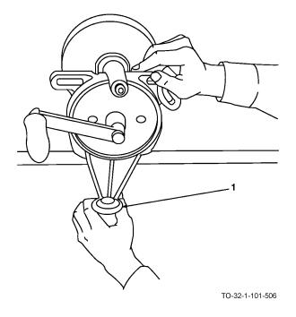
i. When the desired edge is obtained, you are finished. Remove grinder from bench by loosening the clamp (1). Store grinder in its designated storage area.
