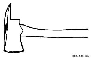
The crash ax, or fireman's ax, is used by emergency personnel to gain quick access to a given area. This ax has a steel head with a cutting blade or bit at one end, and a spike-like extension at the other.
