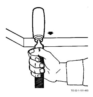
a. To remove a handle, hold the file with one hand. Pull the file from the handle while striking the ferrule end of the handle against the edge of a bench.
