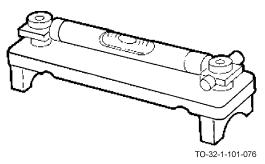
The iron bench level is made of a special design casting which insures its lightness, strength, and rigidity. It is used mostly in the construction industry. It may also be used in a machine shop.
