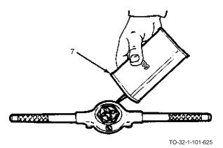
c. Apply cutting oil (7) to the die and to the work.
