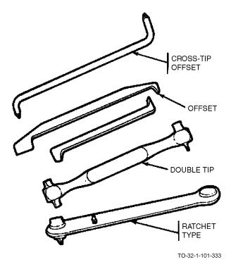
Offset screwdrivers are used to drive or remove screws that cannot be lined up straight with common screwdrivers, or are located in tight corners. Some offset screwdrivers are made with two blades, one of a different size at each end. Others are ratchet-type offset, which are reversible for working in tight spots and allow the screw to be driven without having to remove the tip from the Screw head. A double-tip offset screwdriver has four blades.
