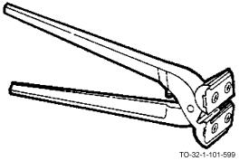
Nippers are used to cut protruding metal flush with a surface. They are also used to cut wire, bolts, nails, and light metal bars to specified dimensions. Nippers come in a variety of styles and sizes.
