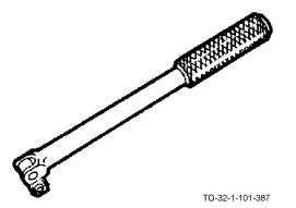
A hinged handle has a hinged adapter on one end which may be rotated in 90 degree steps. The hinged handle is used when additional leverage or torque is needed to loosen nuts or bolts.
