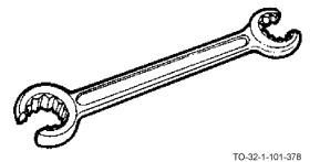
The split-box wrench is a 12 point wrench with 2 points cut away. The split-box wrench is used on pipe unions or cou-
