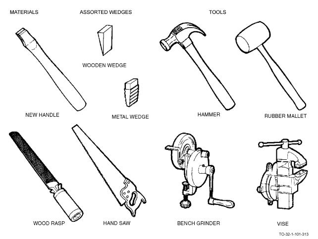
The above items are the basic materials required to replace the handle on a typical carpenter's hammer.
