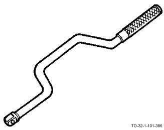
The speed handle has a brace-type shaft with a revolving grip on the top. It is used for rapid removal and/or installation
