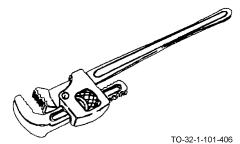
The stillson pipe wrench has a fixed jaw which is on the end of the handle and an adjustable jaw at the top of the
