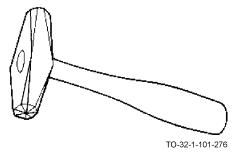
The napping hammer has a high carbon steel head with two tapered faces and weighs about 3 pounds. It is used for chipping stone surfaces or for forming stones during road construction or similar stone work.
