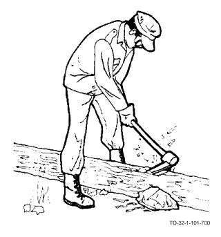
d. Use short, choppy down strokes while keeping the hands in approximately the same position on the handle. The right hand does not slide toward the left hand as in swinging the ax, because the right hand must be in a position to keep control of the adz head at all times. Sliding the right hand to the end of the handle would allow the adz blade face to be deflected toward the user.
