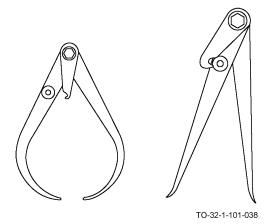
Transfer calipers are used for measuring chamfered grooves or flanges. A screw attaches a small auxiliary leaf to one of the legs. The measurement is made as with ordinary calipers. The leaf is locked to the leg. The legs may be opened or closed as needed to clear the obstruction. The legs are then brought back and locked to the leaf, restoring them to the original setting.
