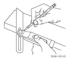
c. Mark with a pencil or marking crayon. Make sure the square does not move while marking.
