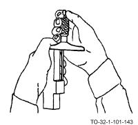
Measuring projection depth with micrometer precision.
