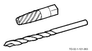
The spiral-tapered type requires a twist drill for drilling a pilot hole.
