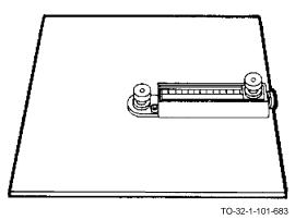
The compass-style circle gasket cutter cuts gaskets from 4 inch diameters through 20 inch diameters. It cuts leather, paper, plastic, rubber, sheet lead, or thin wood. It has an aluminum frame with a graduated scale, steel pivot pin, and tempered tool steel knives. It requires a knurled thumb screw adjustment to change diameters.
