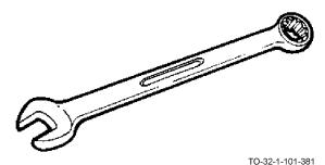
The combination wrench combines the best features of the open-end and box wrench into a single wrench. The size opening on the wrench is the same on both ends, but one end has a box head and the other end has an open-end head. The length of the wrench varies with the size of the head. The most common opening is offset from the shank by 15 degrees. They are used to remove common-size nuts and bolts.
