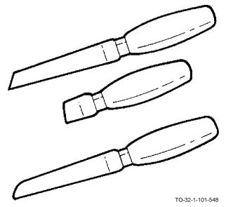
Rubber cutting knives come in a variety of styles and shapes. Some taper to a blunt round point. Some have a short, wide blade. Others have a long, wide hollow ground blade. The handle is usually oval in shape.
