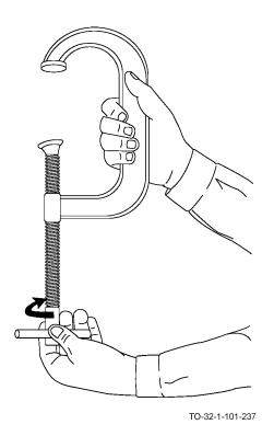
a. Select a clamp which has an opening about 1-1/2 to 2 inches wider than the material to be clamped. Glass and highly polished surfaces must be protected. Use brass shims or wooden blocks. Open clamp as wide as it will go.
