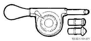
Registering speed indicators are designed to count the number of revolutions of wheels, shafts, etc. Revolutions are counted by attaching spindle of speed indicator to hub of shaft or wheel. Indicator spindle will turn in either direction counting each revolution on a circular dial. Various designs of speed indicators are available depending on nature of use.
