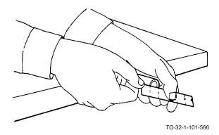
b. Measure outside pipe diameter to determine the proper die.
