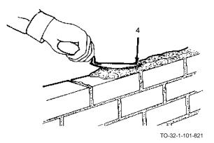
g. To allow enough movement to position bricks, groove the mortar bed with the point (4) of the trowel.
