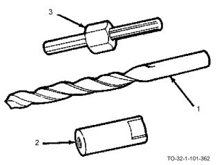
The straight-flute type requires the following tools to drill a pilot hole in the screw: a twist drill (1), a drill guide (2), and a turn nut (3).
