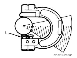
b. If the shaft is not oversized, the first button (3) will pass over it easily.
