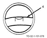
Some levels have a bent tube (4) which allows the bubble to settle quickly.
