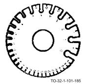
A wire gage is circular in shape with cutouts in the outside edge. Each cutout gages a different size wire, from 0 to 36 of
