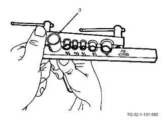
b. Insert tubing to be flared (3) into die block clamp.
