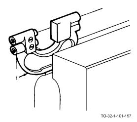
a. The snap (1) gage must first be clamped in a holder.
