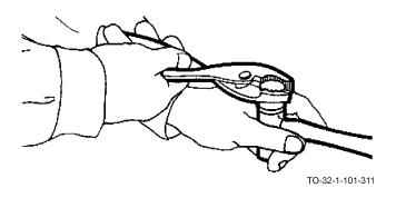
a. Broken or chipped faces may be removed by turning in a counterclockwise direction.
