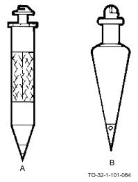
The surveyor's brass plumb bob may be either a spool type (A) or an adjustable cap type (B). Both types have replaceable steel points for increased accuracy. The adjustable cap allows the operator to make minor corrections to height and rotation to make sure the bob hangs straight. The surveyor's brass plumb bob comes with a minimum of 7 feet of nylon, silk or linen cord. It comes in 6, 8, 10, and 16 ounce sizes. The heavier plumb bobs are better for use in windy areas.
