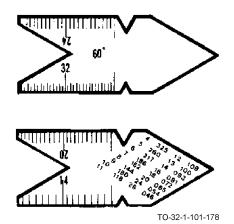
The center gage is graduated in 14ths, 20ths, 24ths, and 32nds of an inch. The back of the center gage has a table giving the double depth of thread in thousandths of an inch for each pitch. This information is useful in determining the size of tap drills. Sixty-degree angles in the shape of the gage are used for checking Unified and American threads as well as for older American National or U.S. Standard threads and for checking thread cutting tools.
