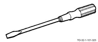
The common screwdriver has a round steel blade with a wood or plastic handle, usually fluted for a good grip. Integral
