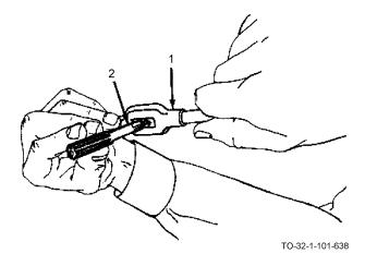
b. Using a tap wrench (1), tighten the handle to the square end of the reamer shank (2).
