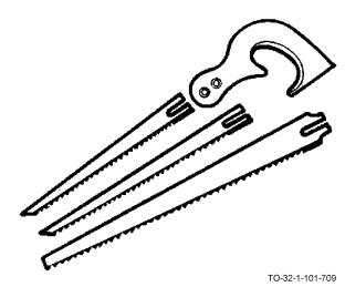
Nested saws consist of a wooden handle to which several different blades can be attached, making up different types of saws such as the keyhole or compass saw. A slotted end at the heel of each blade slips into the pistol-grip type handle where a wingnut fastens it in place. Nested saws are used to cut along curved lines, to start cuts for larger saws, or to make starting saw cuts from drilled holes or small openings. The size of these saws will vary depending on design and nature of use.
