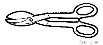
37.2.1 <u>Hand Shears</u>. Hand shears are made with straight or curved cutting blades. Shears are made for right-handed operators so the cutline is always in full view for accurate cutting.
