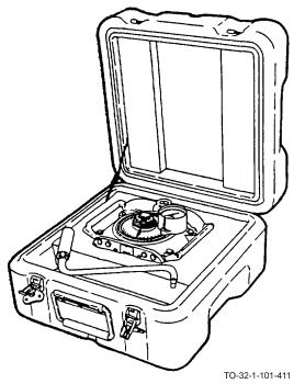
Using a powerful gear train, the power torque wrench is completely mechanical in operation. The power torque wrench is operated by a hand crank, but power tools such as the electric drill can be used to speed operations. The torque is calibrated in foot pounds, which is shown by a dial indicator on the top face of the power torque wrench. This type of torque wrench is used for tightening nuts and bolts requiring 200 or more foot pounds of torque.
