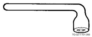
The 90 degree offset handle socket wrench has a fixed socket at the end of a bent handle. It is used for removing and/or installing a nut or bolt which may not be reached with a box or combination wrench.
