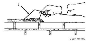
e. Move the trowel steadily backward, tilting it to slide the mortar gradually from the blade (3), leaving an even bed of mortar on the work surface.
