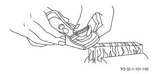
e. Raise the plane from the work after each stroke and return to the starting point.
