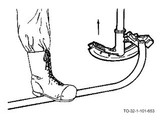
e. When desired bend has been obtained, release the pressure on the conduit by returning the handle to an upright position and slide the conduit out of the bender.
