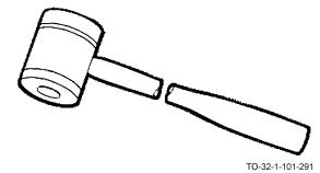
The wooden maul has a cylindrical head which is about 8 inches in diameter and about 10 inches long. It is used to drive wooden pickets, posts and stakes.
