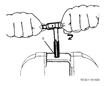
d. Place point of the tap in hole (5) and rotate clockwise for right-hand threads or rotate lefthanded tap counterclockwise for left-hand threads.
