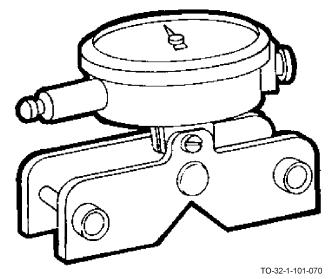
The magnetic base indicator holder is a one-piece metal assembly that attaches to the work surface magnetically. A gage or indicator attaches to the assembly. Base indicator holders are used for attaching gages to lathes, milling machines, shapers, or any machine where graduations are difficult to read. Magnetic base indicator holders are available in many sizes and designs depending on application.
