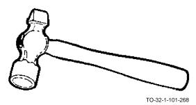
A straight peen hammer is used like the cross peen but differs from the cross peen since its peening edge is turned ninety degrees. This keeps the handle parallel to the struck surface.
