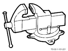
The machinist's bench vise has rough jaws which prevent the work from slipping. It has a swivel base, allowing the user to position the vise in a better working position. Machinist's bench vises are usually bolted to a work bench or table. They are used for holding or clamping large, heavy objects.
