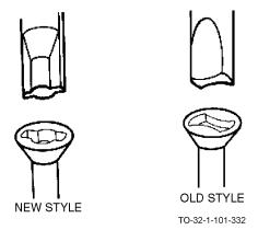
Clutch head screwdrivers are used to drive clutch-bit screws. These screws have recessed heads and are commonly called butterfly or figure-eight screws. There are two styles of clutch heads, old style and new style.
