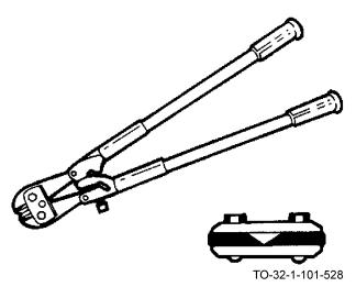
The cutting edges of the clipper cut cutter are in line with the handles and beveled almost entirely from one side. These cutters allow very close cutting of projecting ends. The cutting capacities range from 1/4 inch to 9/16 inch for medium steel, and from 5/16 inch to 11/16 inch for soft steel. The handles range from 14 inch to 42 inch lengths.
