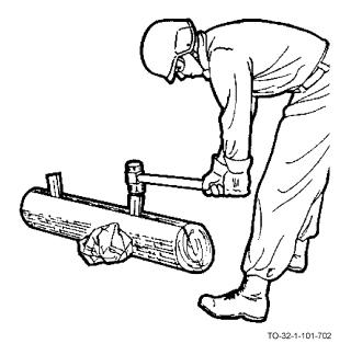
d. Give the wedge a few blows, then start a second wedge on the line farther along the log and drive it with a few sledge blows.
