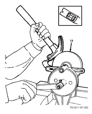
h. Remove excess portion of wedge using a bench grinder (13). Check handle. If it's tight, the task is complete. If handle is loose, repeat procedure.
