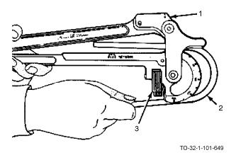
f. Raise the slide bar (1), lift up the locking clip (3), and remove the bent tube (2).
