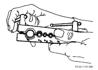
c. Hold tubing so there is about 1/8 inch extending above die block clamp, and tighten die block clamp screws.
