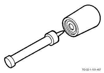
The grommet-inserting punch consists of two parts. The solid punch part has a tapered point and a flat shoulder. The round die part has flat ends with a bored hole in one end to receive the point of the punch. Grommet-inserting punches are used to form the flange on grommets which are installed along the edges of flags, sails, mail bags, and similar items.
