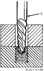
b. Insert extractor (3) in the drilled hole.
