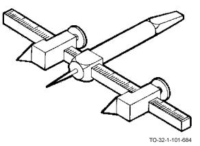
The bit brace circle gasket cutter adjusts from 1 to 5-1/2 inches in diameter. It cuts metal, plastic, wood, hardwood and other materials. It has a tapered square shank to fit a bit brace. It comes with a 3/16 inch tool steel bit, 1/4 inch pilot drill, and a hexagon wrench for easy adjustment.
