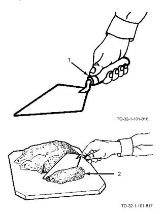
b. Slice off a trowel load of mortar (2).
