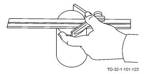
b. Put the center head flush against the cylinder.
