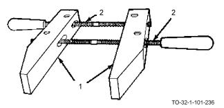
The hand screw clamp is made up of two hardwood or high impact plastic jaws (1) and two hand-operated screws (2) which hold the clamp together. The hand screw clamp is used for holding wood while gluing. They are available in a variety of sizes.
