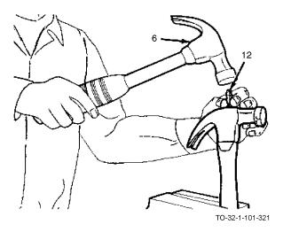
g. Select metal wedge (12) and drive into wooden wedge with hammer (6).
