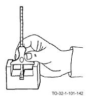
Measuring the distance from a surface to a recessed point.
