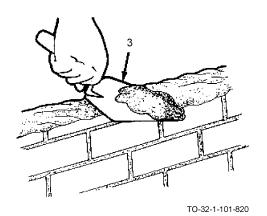
f. Cut off excess mortar after each application by holding the trowel blade (3) slightly angled against the work surface and moving forward.
