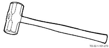
A double face sledge hammer has similar faces on both sides of the head.
