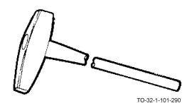
The railroad track maul has a flat faced tapered head which weighs about 10 pounds. They are used for driving railroad track spikes.
