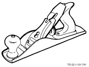
One of the most common types of bench planes is the jack plane. Like all bench planes, the jack plane is designed for cutting with the grain of the wood. Its cutting blade is set at approximately 45 degrees and is used for all purpose planing or to cut lumber to specified lengths.
