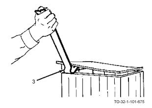
a. Insert the long tapered blade (1) between boards (2) to be removed or ripped. Then exert leverage on the short hooked blade (3) of the bar to pry the boards loose.
