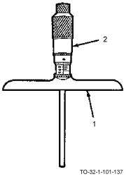
The micrometer depth gage consists of a flat base (1) that is attached to the barrel of a micrometer head (2). These gages have a range from 0 to 9 inches, depending on the length of extension rod used. The hollow micrometer screw has a 1/2 or 1 inch range. Some are provided with a ratchet stop. The flat base ranges in size from 2 to 6 inches. Several extension rods are supplied with this type gage.
