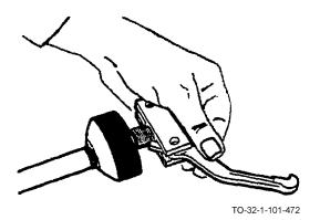
c. Hold the assembled parts while you remove the punch.
