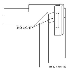
b. To check the end of a board, place stock on vertical edge and extend blade over the end. Light must not be seen around blade edge. If light is seen, the work is not square.
