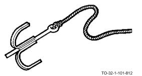
The trip wire grapnel is a metal weight resembling three or four fish hooks, with a common shank ending in an eye. The hooks spread out in different directions at the other end of the shank. Attached to the eye portion of the shank is a marlin
