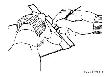
e. Hold down on the straight edge with one hand while holding the cutter (5) in an upright position in the other hand. Your forefinger should extend along the holder with your fingertip near the wheel.
