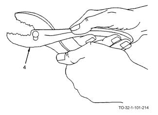
c. Adjust pliers (4) to obtain a wide jaw opening.
