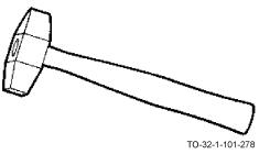
The sawmaker's hammer has a tapered blunt face on one end of the head and a tapered chisel face on the other end. It is used for setting the teeth on saws when a setting tool is unavailable.
