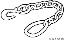
The chain assembly is a heavy duty linked chain with a grab hook at one end and a ring at the other. The chain assembly is used for such applications as towing vehicles, slinging loads, and hauling objects. The chain assembly is available in a wide variety of lengths and link sizes depending on the nature of the use.
