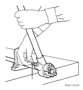
n. Reverse ratchet by pulling ratchet control knob (5) from detent and turning it 180 degrees. Then back up the cutting die.
