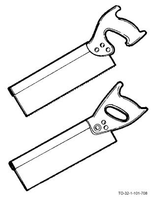
The backsaw has a straight blade and parallel top and bottom, with a heavy strip of steel or brass wrapped along the back to provide rigidity. The handle is of similar shape to other hand saws except it is usually mounted higher. Backsaws are used for general bench work such as cutting joints and smaller sections of lumber to length. Sizes vary depending on design and nature of work.
