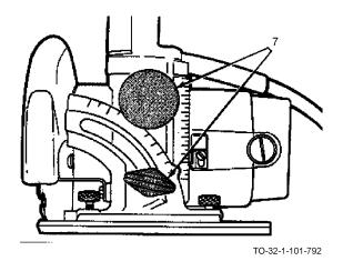
f. Set the saw's guides (7) to the correct angle and depth of the cut required.
