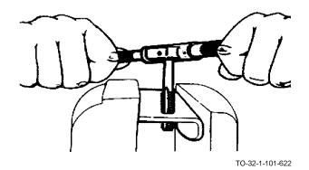
f. Replace the tap wrench and continue tapping operation. It is not necessary to apply pressure, as the threads will be pulled through at all times.
