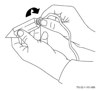
d. Tighten cap securely in the body and suspend the plumb bob by the cord only. Make sure the knot will support the plumb bob.
