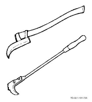
47.2.2 <u>Machete</u>. The machete normally in military use is an 18 inch knife, widest and heaviest at the point of the blade. The blade is attached to a handle shaped to fit the hand. The handle is designed with a slight projection to prevent the machete from slipping from the hand while being used. The machete is used to cut tall grass, vines, and small brush.
