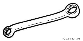
The most common box wrench is the double offset box wrench. It comes with a different size opening at each end. The double offset wrench is used to remove normal nuts and bolts.
