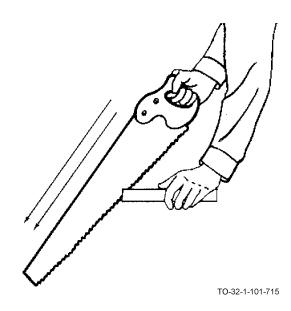
d. At approximately a 45 degree angle, saw only on the downward stroke applying pressure evenly.
