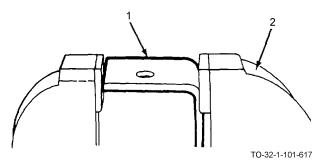
a. Clamp a steel plate (1) securely in a vise (2). Drill and ream a hole of desired size.
