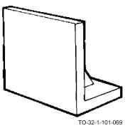
Angle plates are devices consisting of two flat outside working surfaces jointed at right angles. The outside work surfaces are precision ground. The standard angle plate is permanently jointed at a right angle. However, an adjustable type with varying angle adjustments is also available. Angle plates are used for clamping or holding work vertically. They are also used for layout, inspection, or machine set-up. Various sizes and designs are available depending on the task.
