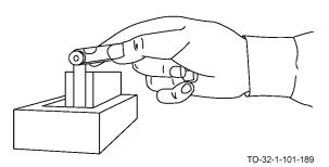
A long blade thickness gage is used to determine the fit between large mating surfaces. By combining blades it is possible to obtain a wide variation of thickness.
