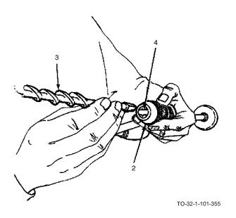
b. Open chuck (2) and insert bit (3) between jaws (4). Tighten chuck (2), securing bit (3).
