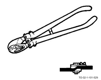
Shear cut, flat bar, and strip cutters are used to cut flat-soft, medium-hard bar, and strip stock. The cutting edges of the jaws pass each other in the manner of scissors, making a complete shear cut. The cutting capacities range from  $7/8 \ge 5/32$  inch to  $1-1/2 \ge 9/32$  inch for soft and medium steel, and from  $3/4 \ge 1/8$  to  $1-7/16 \ge 1/4$  inch for hard steel. The handles range from 14 inch to 36 inch lengths.
