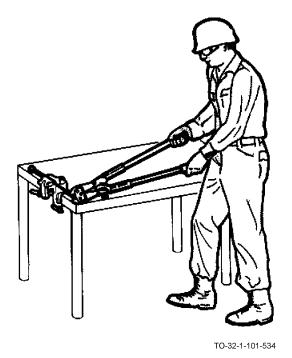
d. Stand at a right angle to the work being cut and apply steady pressure to the handles until the work has been cut off. Do not pry or twist with the handles while cutting.
