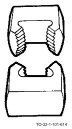
The two-piece collet die consists of the two die sections, the collet cap, and collet guide. The die sections are placed inside the cap and held in place by the guide. Adjustment of the die is done by turning setscrews on either end of the internal slot. They are used to cut American Standard Coarse and Fine Threads and are available in assorted sizes.
