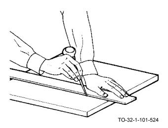
c. Hold straight edge firmly. Hold the awl like a pencil and scribe a line along the straight edge.
