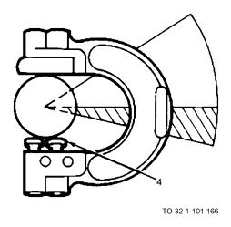
c. Move the gage to the position shown above. If the NO GO button (4) stops the gage, the shaft is within limits.
