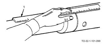
a. Place material to be marked on a firm surface. Place a steel rule or straight edge (1) on the work beside the line to be scribed.
