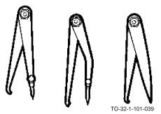
The hermaphrodite calipers have one straight leg ending in a sharp point. On some models this point is removable. This leg is usually bowlegged. This caliper is used for finding shaft centers or locating shoulders.
