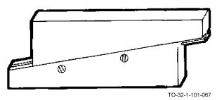
Adjustable parallels consist of two tapered parts fitted together. The distance between the two outside parallel surfaces varies by moving mating parts together or apart. This distance is then measured with a micrometer. Adjustable parallels are used as gages for leveling and setup work. Adjustable parallels are available in various sizes depending on the nature of work.
