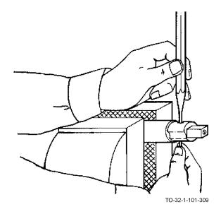
c. Catch the pin in your right hand before it falls out of the shaft.
