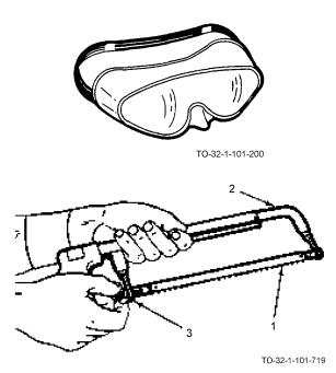
a. Insert the correct blade (1) in the hacksaw frame (2) and adjust wing nut (3) for proper tension.
