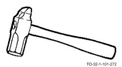
Cross peen hammers have a broad flat face on one side of the head and a peening chisel edge on the other side.
