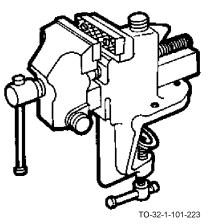
The clamp base bench vise is a lightweight, portable machinist's vise. It is attached to a table or bench with the mounting clamp. It has rough jaws for holding material and may have a swivel base. Clamp base bench vises are used to hold light materials or in areas where a heavier vise is not available.
