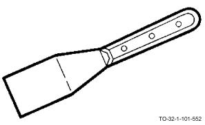
A putty knife is used for applying putty to window sashes in setting panes of glass. The blade has a wide square point and is available in different lengths and widths.
