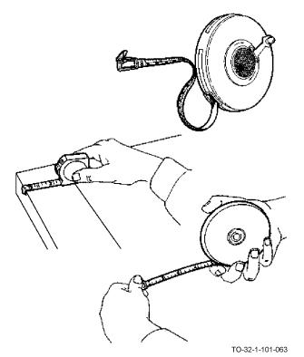
Steel tapes are made from 6 to about 300 feet in length. The shorter tapes are made with a curved, but rigid, cross section flexible enough to be rolled up. Long, flat tapes need support over their full length to avoid sagging. Lack of support can cause reading errors. The most common types of steel tapes have a hook at one end to let one person take all the readings.
