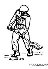
c. Slide one hand near enough to the blade to raise the weight of the blade and the dirt.
