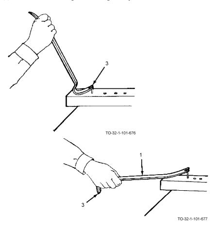
c. To remove nails, use the short hooked blade (3) nail slot to remove a nail that is almost completely driven home. Pull the nail approximately half-way out. Then switch to the long tapered blade (1) nail slot to completely remove the nail.
