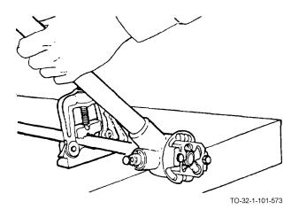
1. After two more turns on the die, back off one turn and apply a coat of cutting oil.
