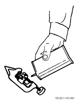
Keep cutting wheel clean and lightly oiled. If a reaming device is mounted on the body of the cutter, keep it retracted when not in use. Store tube cutters on a rack or in a box.
