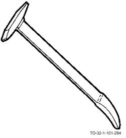
The welder's hammer has one or two tapered chisel faces. Those having only one tapered face have a replaceable brush attached. The hammer face is used for chipping welds, while the brush is used for cleaning welds and brushing away the slag chipped from the weld.
