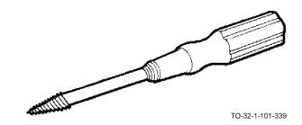
A screw starter or gimlet has a threaded tip. It is used to make a pilot hole in wood for wood screws.
