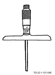
Depth micrometers are used to measure depths to an accuracy of 0.001 inches.
