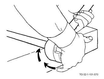
i. Slide cutting die over end of pipe to be threaded and apply light pressure with the heel of your hand.
