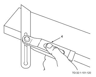
b. The angle may now be laid out by extending the blade across the board with the stock (4) held firmly against the edge.
