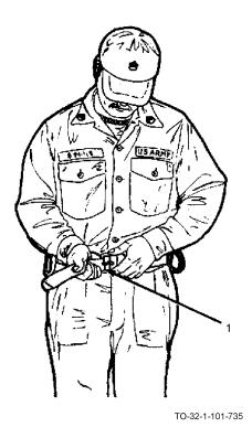
a. Secure safety belt (1) around waist and place tools needed in position on belt.
