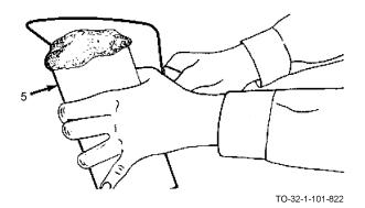
h. Using the trowel, coat the brick ends (5) with mortar before laying them in place.
