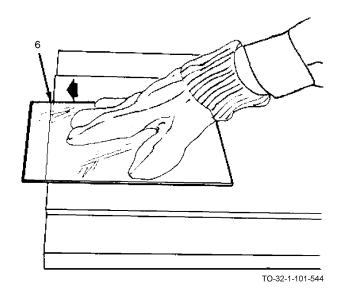
g. A proper cut is indicated by a slight crack in the surface. It is best seen from the side opposite the mark.
