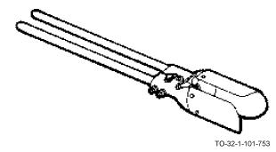
The posthole digger has two concave blades similar to the posthole auger except that each blade is fastened to a long, wooden handle. The blades are hinged at the top so that separating the handles will close them and moving the handles together will open them. Like the auger, the posthole digger is used to bore holes in the ground for posts, explosive charges and similar jobs.
