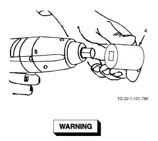
Do not use standard sockets with any impact tool they can shatter causing serious injury and/or damage to the equipment.
