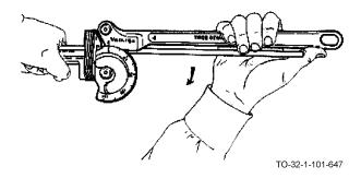
d. Apply downward pressure on the slide bar.
