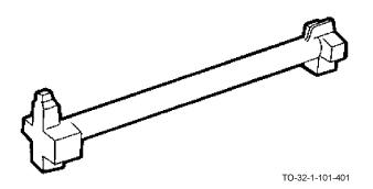
The multiple plug wrench combines several plug ends on a common handle.
