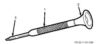
Jeweler's screwdrivers are made for driving and removing small size screws. They usually have knurled handles (1), and a swivel end finger rest plate (2). The tips (3) range from 0.025 inch to 0.1406 inch wide. Some jeweler's screwdrivers have removable blades.
