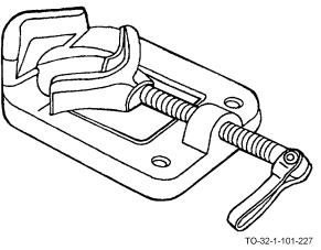
The piston holding vise is a special purpose vise which can hold engine pistons up to and including 5-1/2 inches in diameter. This vise may be bolted to a bench or table.
