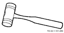
The tinner's mallet has a cylindrical wooden head which is from 1-1/4 to 3-1/2 inches in diameter and from 3 to 6 inches in length. It is used to form and shape sheet metal.
