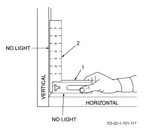
a. To check a square joint, place the stock (1) against a horizontal section and the blade (2) against a vertical section. Light must not be seen around blade edge. If light is seen, the work is not square.
