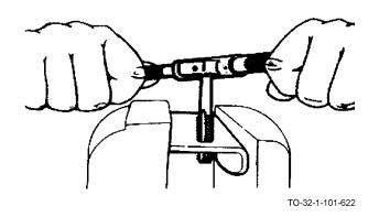
g. Remove tap by turning in the opposite direction. Wipe excess oil and metal shavings from metal plate. Check newlycut threads with screw pitch gage before inserting screw or stud.
