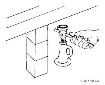
d. Block the load to withdraw the jack.
