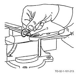
b. Grasp the other section of the extending cotter pin (3) and bend it back flat against the metal surface or nut.
