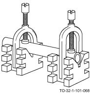
The V-block and clamp assembly consists of a V-shaped, hardened steel body to support round, square, or rectangular shaped work. A clamp (or clamps) holds the work firmly in the body groove. V-blocks and clamps are especially used for grinding, milling, or drilling purposes. Various styles and designs of V-blocks and clamps are available depending on application.
