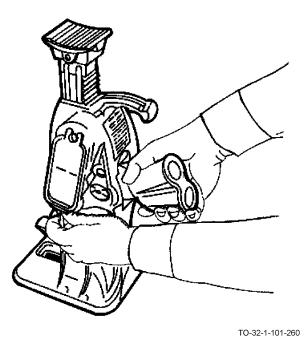
d. When the head of the five-ton jack is not supporting a load, the rack can be allowed to fall free by pressing the reversing lever all the way to the rear and slightly lifting up on the lifting lever. The rack will not fall free if even a slight load is still on the head.
