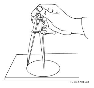
c. Lean the dividers in the direction of movement and scribe the circle by revolving the dividers.
