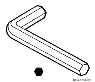
The hexagon key wrench is an L-shaped, six sided wrench. Both ends of the "L" are the same size so you can turn the wrench either to gain access to the screw head or to obtain a leverage advantage. The hexagon key wrench is used to remove and/or install hexagon head screws.
