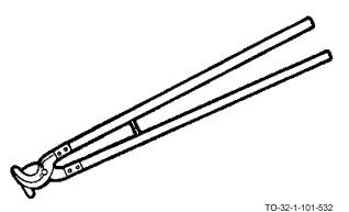
Shear cut cable cutters have curved interposing cutters. They are used to cut lead and rubber-covered cable, and communication cable. Cutting capacities for lead and rubber-covered cable is 1-3/8 inches for the 25-1/2 inch handle, and 2-1/4 inches for the 37 inch handle. The communication cable cutting capacity for the 25-1/2 inch handle is 500,000 circular
