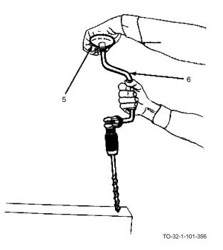
c. Center bit over pencil mark. Push down on head (5) and turn crank (6) until bit goes through the board.
