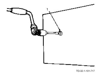
a. To make an inside-out cut, first drill a hole (1) large enough to admit the point of the saw.
