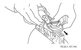
d. Push along the length of the board with a steady, even stroke.
