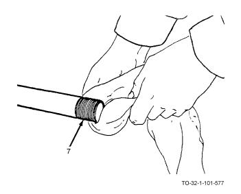
q. Wipe excess oil and shavings from threaded end of pipe (7).
