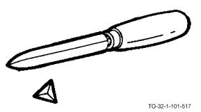
Triangular blade scrapers are used for removing high spots from flat or curved surfaces. They are available with either a 4 or 6 inch blade.
