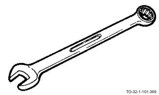
All open-end wrenches have open jaws on one or both ends of the wrench. Most jaw openings are offset from the shank portion of the wrench by 15 degrees. The wrench length is determined by the size of the jaw opening. Some of the more
