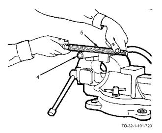
b. Secure the material (4) to be cut in a vise or other holding device to avoid vibration which may snap the blade.
