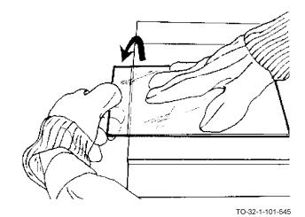
i. Hold down on the section resting on the working surface. Grasp the section extending over the edge with your other hand. Apply a light downward pressure to part the glass.
