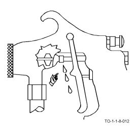
Figure 4-12. Paint Leaks From Spray Gun
