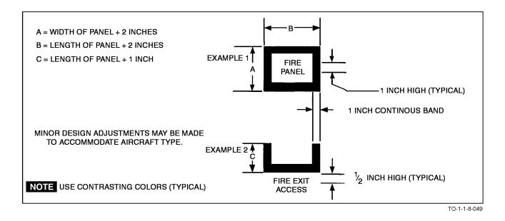
Figure B-9. Markings For Fire Access Panel
