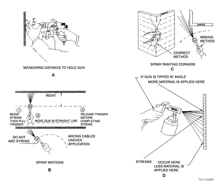
Figure 4-7. Right and Wrong Methods of Spraying
