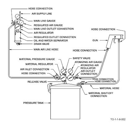
Figure 4-2. Simple Spray System Setup
