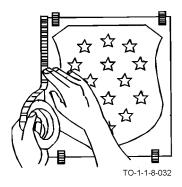
Figure 7-4. Applying Large Emblems (Step 2)
