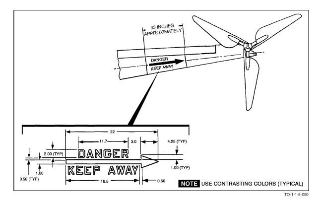
Figure B-10. Helicopter Tail Boom Markings
