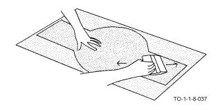
Figure 7-9. Use of Application Tape (Step 3)
