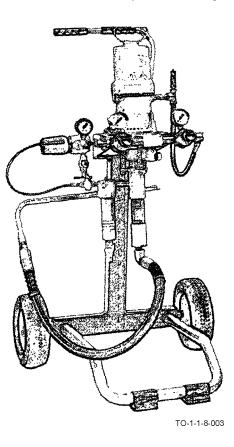
Figure 4-3. Airless Spray System
