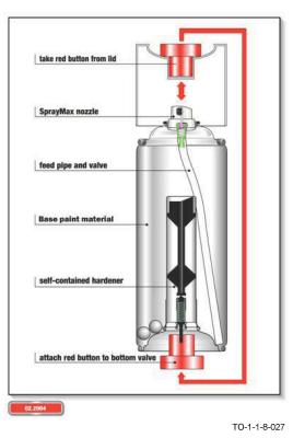
Figure 5-5. Two-Component Aerosol
