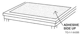
Figure 7-7. Use of Application Tape (Step 1)
