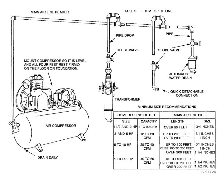
Figure 4-6. Proper Installation of Air Compressor, Piping
