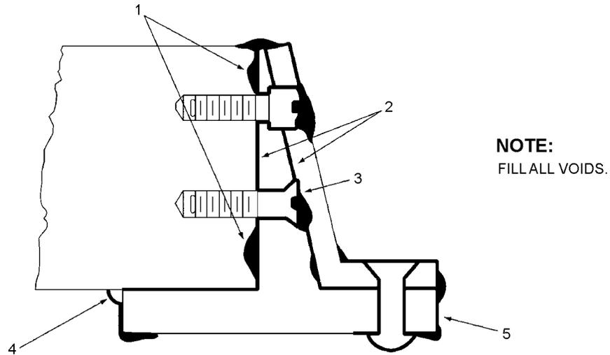
1. REMOVE CORROSION AND SURFACE TREAT IN ACCORDANCE WITH TO 1-1-691, CHAPTER 5.
