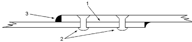
1. ASSEMBLE LAP JOINT WITH MIL-PRF-81733 IN FAYING SURFACES.
