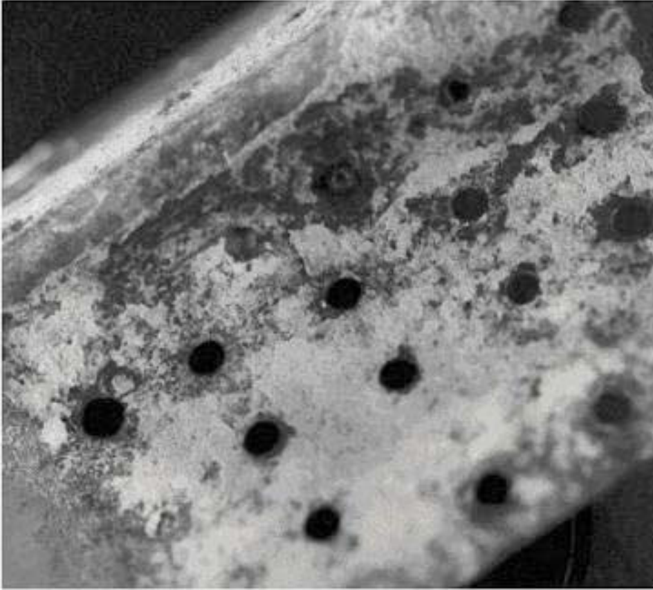
Figure 2-21. Aluminum Surface Corrosion Products
