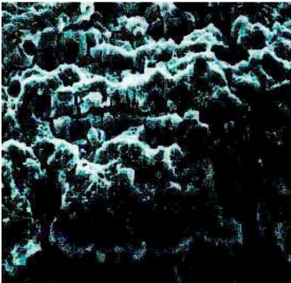
Figure 2-10. Grain Structure of a Corroding Aluminum Surface
