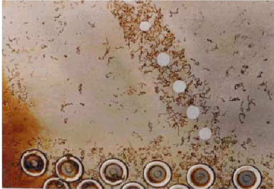
Figure 2-17. Filiform Corrosion Found Under Paint Coating on a Magnesium Panel
