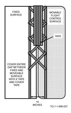
Figure 4-6. "X" Pattern for Control Surfaces
