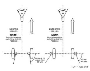
Figure 7-7. Cable Angular Relationship to Aircraft
