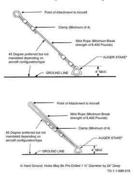
Figure 7-8. Cable Mooring Attachment
