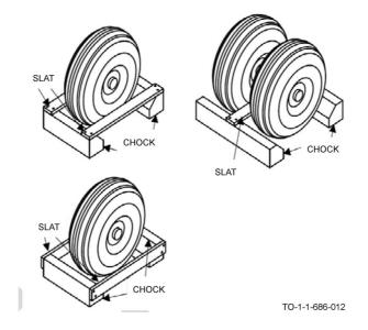
Figure 7-4. Chocks with Slats Attached
