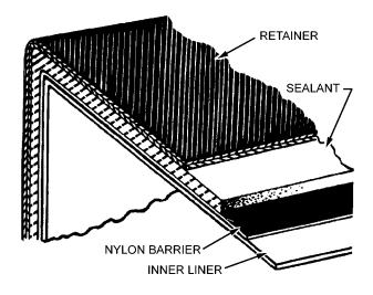
Figure 9-2. Self-Sealing
