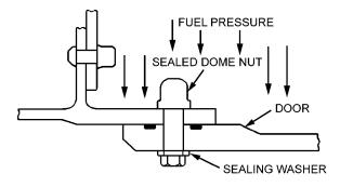
Figure 6-7. Direct Seal Door
