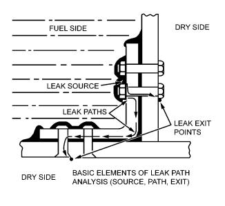
Figure 6-14. Leak Path Analysis
