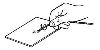
2. ROLL MELTED END ON CARDBOARD OR ANY FLAT SURFACE TO REMOVE EXCESS NYLON AND TO FORM SHARP TIP ON END OF LINE.
