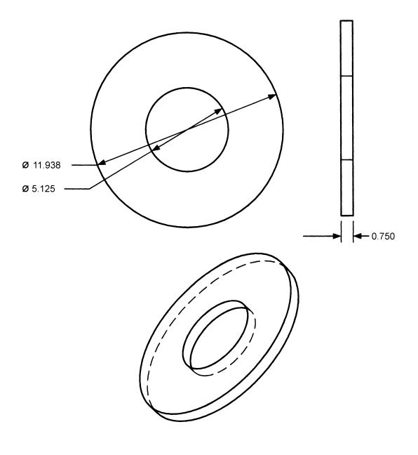
Figure 5-2. Exhaust Purge Adapter (Sheet 6)
