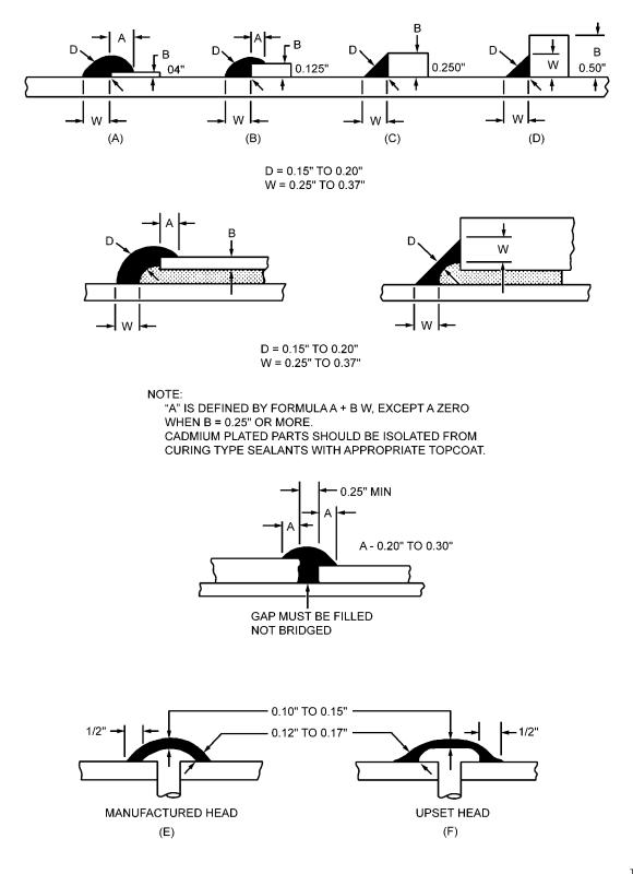
Figure 6-30. Typical Fillet Dimensions
