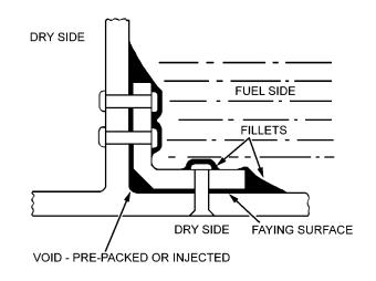
Figure 6-2. Curing Sealant Design
