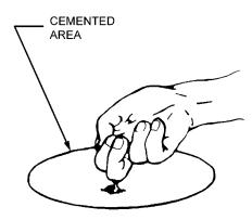
Figure 9-18. Knuckle Test
