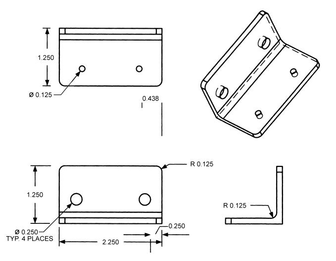
Figure 5-2. Exhaust Purge Adapter (Sheet 10)
