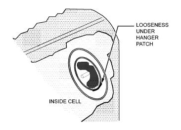
Figure 9-13. Looseness Under Hanger Fitting
