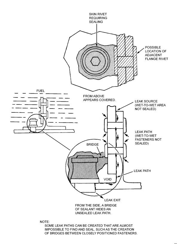
Figure 6-19. Sealant Bridging
