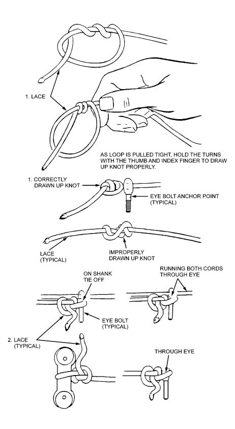
Figure 9-35. Lacing Cord Knots
