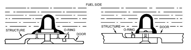
Figure 6-9. O-Ring Seal
