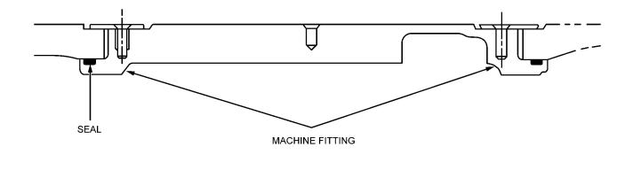
Figure 6-13. Machine Fitted Plug-Type Access Door for Attaching Screws
