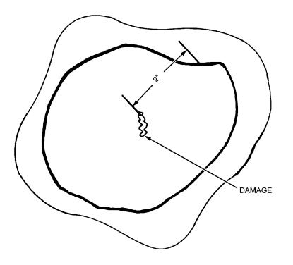
Figure 9-16. Marking Area to be Repaired
