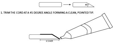
2. APPLY THE SUPERGLUE IN A THING FILM STARTING  $\sim$ 1" FROM THE TIP ACROSS TO THE TIP OF THE CORD INCLUDING THE EXPOSED END OF THE CORD. REPEAT ALL THE WAY AROUND THE CORD UNTIL THE TIP IS COMPLETELY COATED WITH A THIN FILM OF SUPERGLUE.
