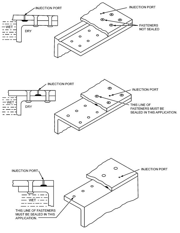
Figure 6-4. Typical Locations of Grooves/Channels (Sheet 1 of 2)
