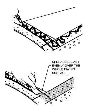
Figure 6-31. Applications of Faying Surface Sealant
