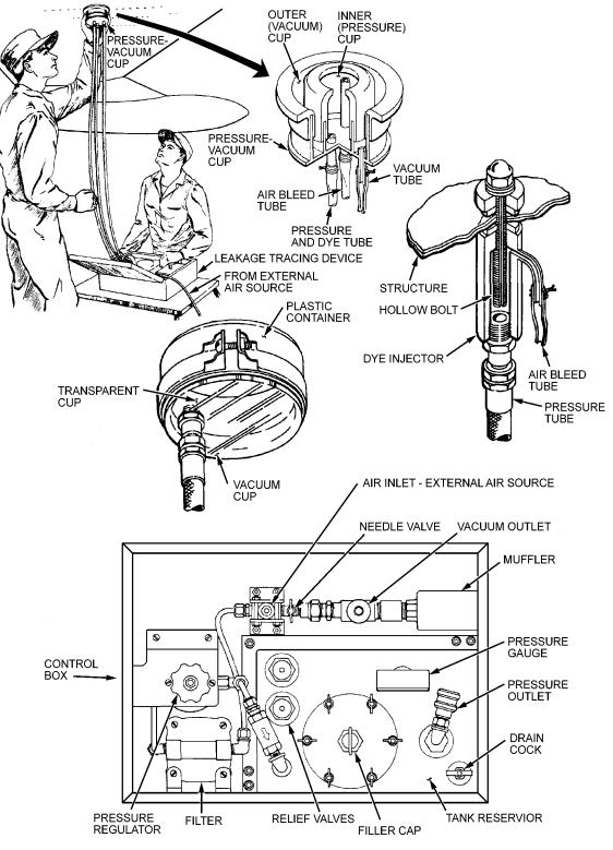
Figure 6-23. Dye Injection Method
