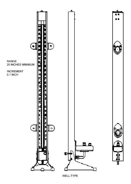
Figure 8-4. Typical Well-Type Manometer
