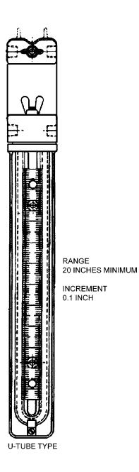
Figure 8-3. Typical U-Tube Type Manometer
