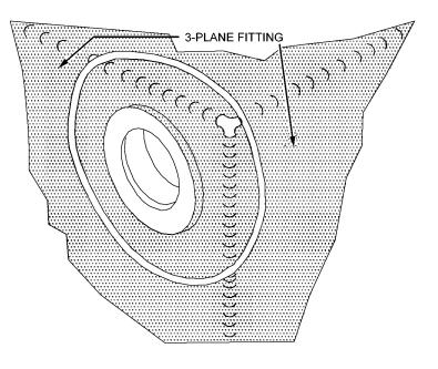
Figure 9-15. Three-Plane Fitting
