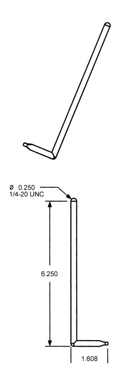
Figure 5-2. Exhaust Purge Adapter (Sheet 3)
