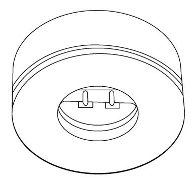
Figure 5-2. Exhaust Purge Adapter (Sheet 12)
