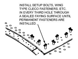
Figure 6-32. Faying Surface Seal Assembly
