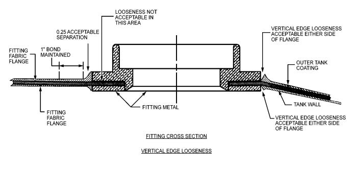
Figure 9-5. Separation of Cell Wall from Fitting Fabric Flange
