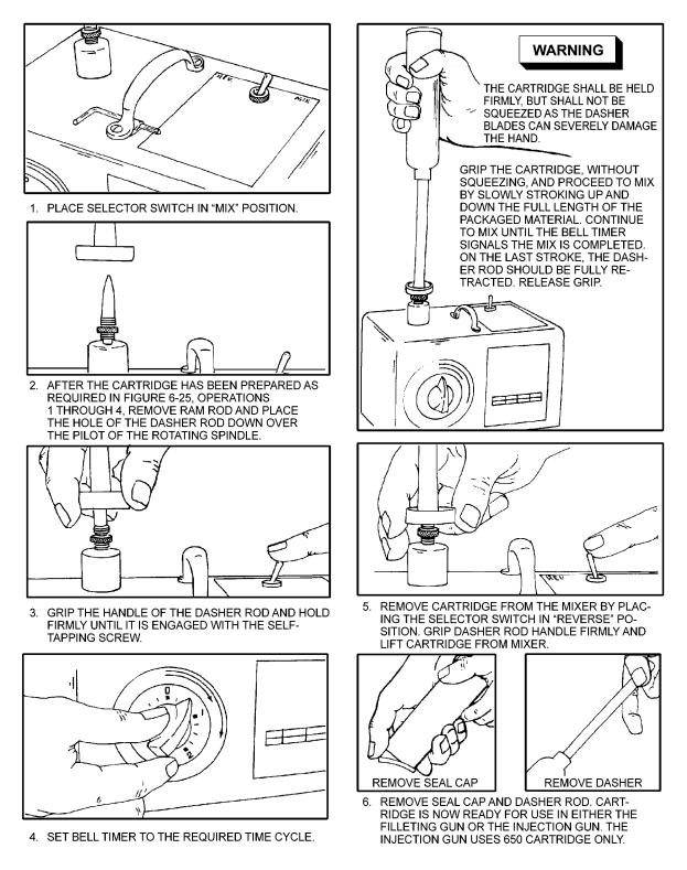
Figure 6-26. Machine Mixing of Cartridges
