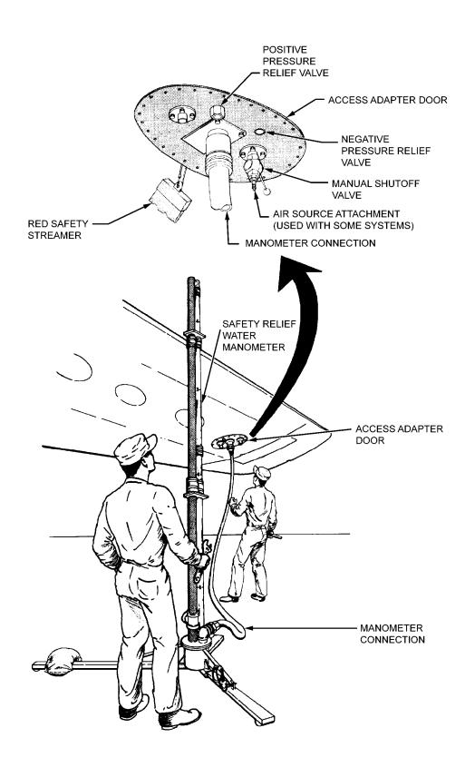
Figure 6-21. Pressure Test Method
