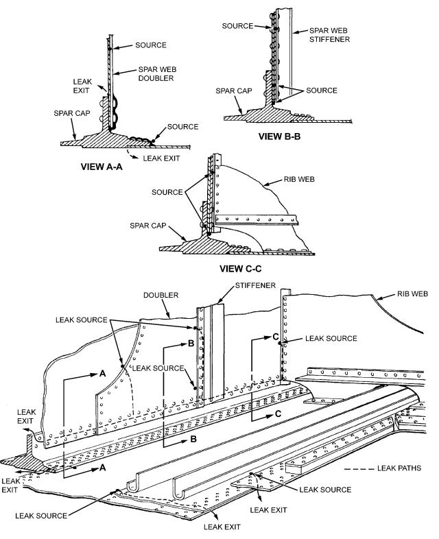
Figure 6-16. Examples of Long Leak Paths
