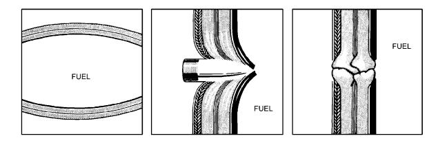
Figure 9-1. Projectile Sealing Action
