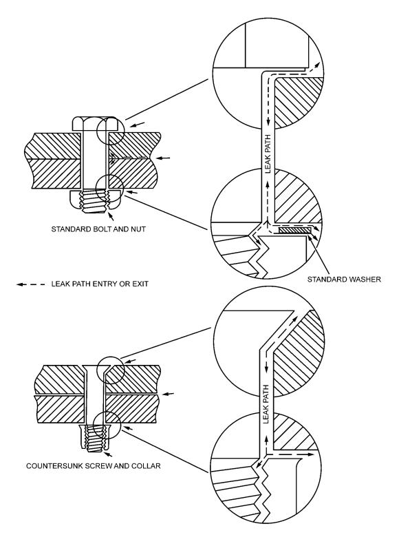
Figure 6-15. Fasteners Leaks
