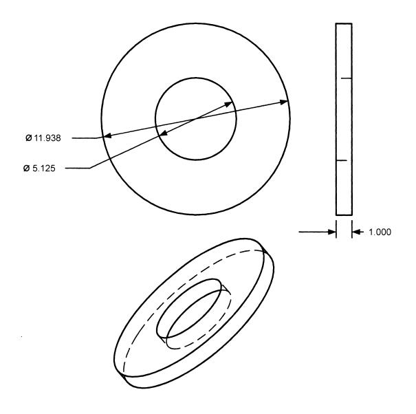
Figure 5-2. Exhaust Purge Adapter (Sheet 5)
