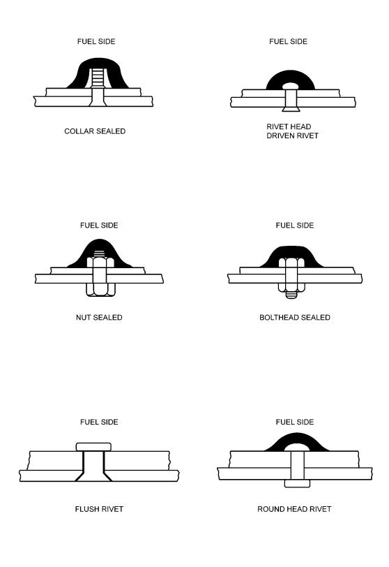
Figure 6-12. Typical Fasteners, Overcoat and Fillet
