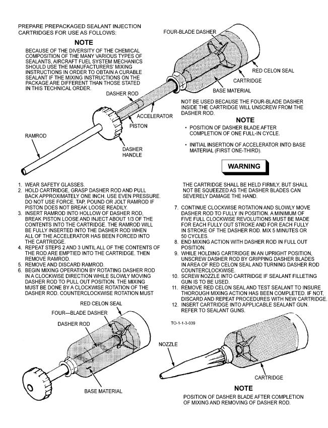
Figure 6-25. Hand Mixing of Sealant Kit
