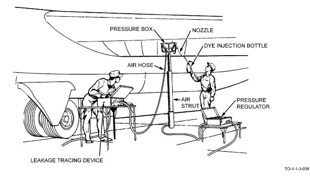
Figure 6-24. Use of Pressure Box for Dye Injection
