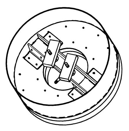
Figure 5-2. Exhaust Purge Adapter (Sheet 8)
