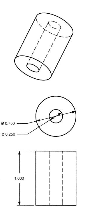
Figure 5-2. Exhaust Purge Adapter (Sheet 2)
