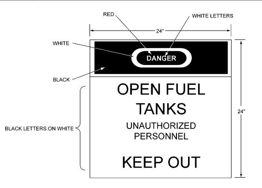
Figure 8-1. Marking of Fuel System Repair Area
