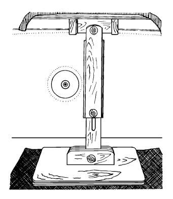
Figure 9-17. Pedestal for Supporting Cells
