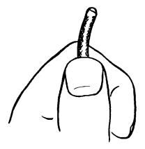
4. ROUNDED END OF LACING LINE PROPERLY PREPARED FOR USE.
