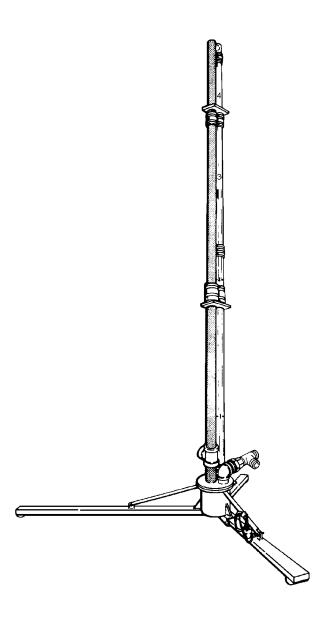
Figure 8-2. Water Manometer
