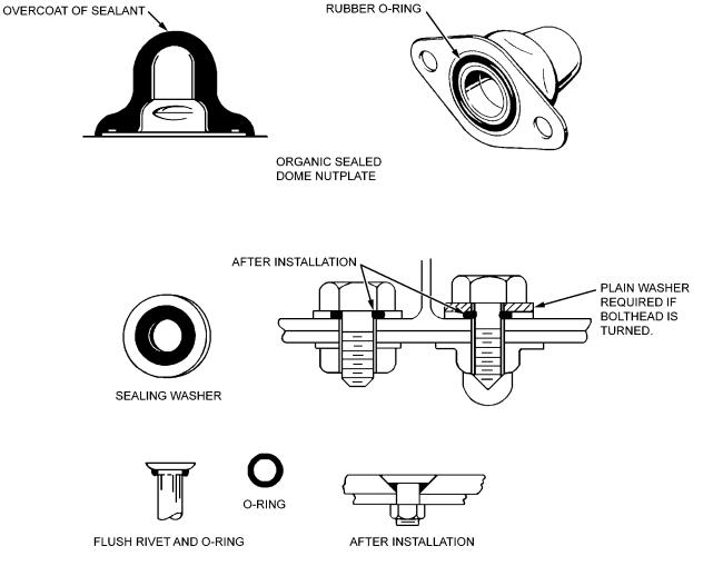
Figure 6-11. Typical Fastener Seal
