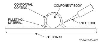
Figure 6-7. Removing Coatings and Fillets from Axial Components
