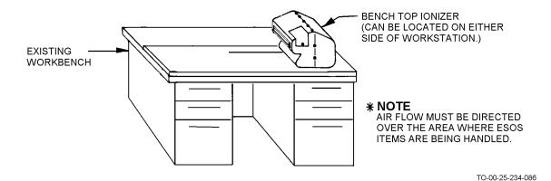
Figure 7-6. Bench Top Ionizer Positioning
