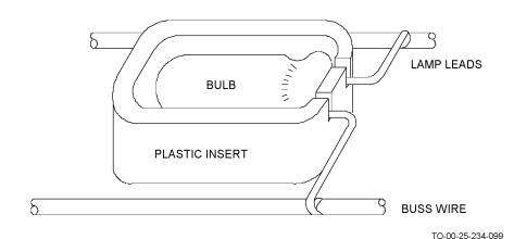
Figure 8-4. Typical Bulb Insert
