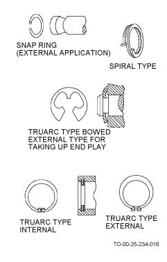
Figure 4-13. Typical Retaining Rings
