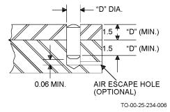
Figure 4-3. Application of Dowel Pin
