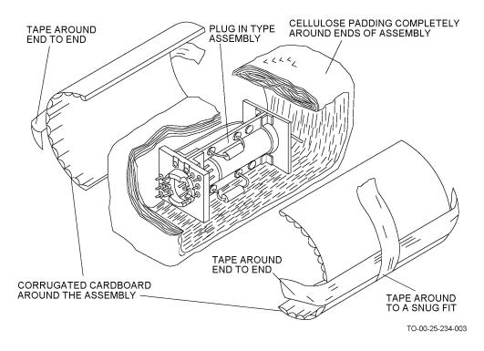
Figure 2-3. Plug-In Type Electronic Assembly, Protective Packaging
