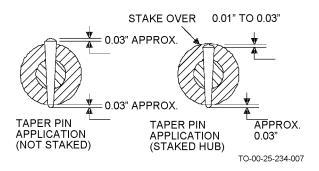
Figure 4-4. Application of Tapered Pins
