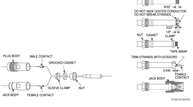
Figure 4-29. Attaching Improved N Connectors to Coaxial Cable
