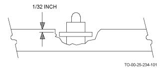
Figure 8-6. Typical Excavated Plug
