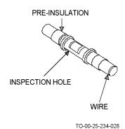
Figure 4-25. Pre-Insulated Permanent Copper Splices
