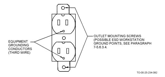
Figure 7-12. Typical Electrical AC Outlet
