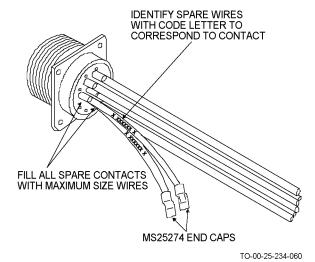
Figure 4-57. Spare Wires for Potted Connector
