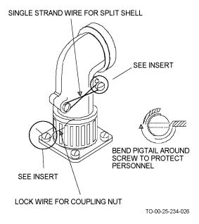
Figure 4-23. Safety Wiring AN Split-Shell Assembly Screws
