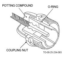
Figure 4-60. Installation of O-Ring on Potted Connector
