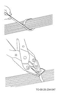
Figure 4-44. Nylon Strapped Spot Tie
