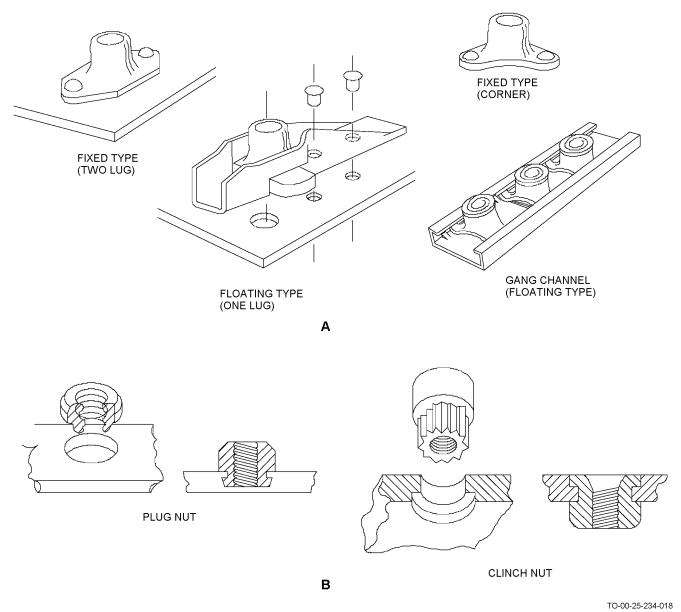
Figure 4-15. Anchor Nuts, Clinch Nut, and Plug Nut
