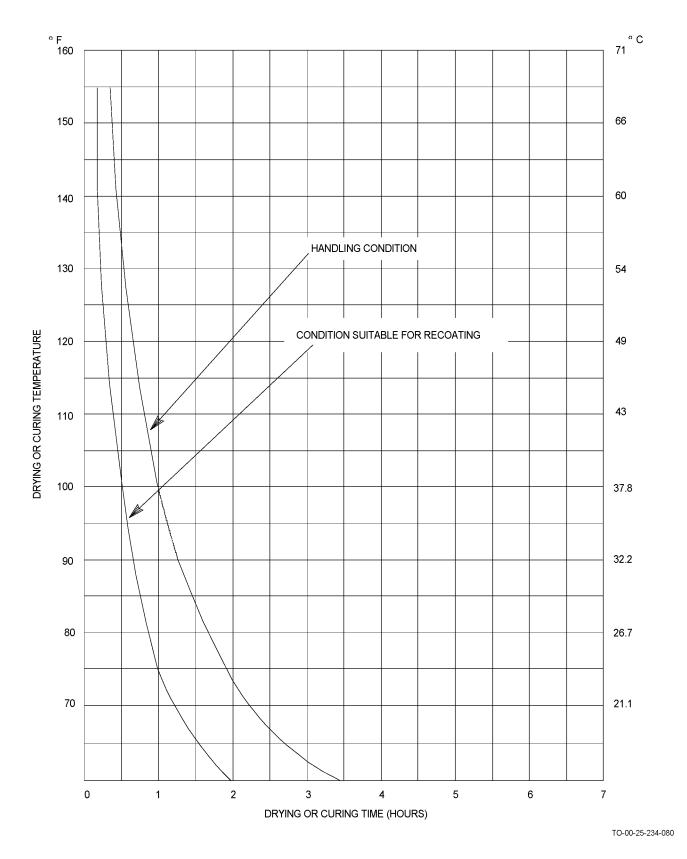
Figure 6-9. Drying or Curing Schedule for Coating Material Applied Near End of Work Life
