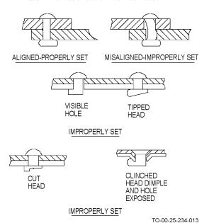
Figure 4-10. Properly and Improperly Set Rivets
