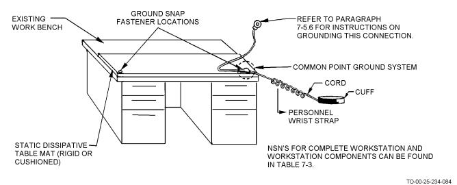
Figure 7-4. Static Control Workstation (work cushioned or rigid work surface on an existing work bench)
