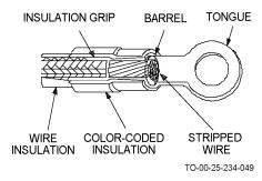
Figure 4-46. Pre-Insulated Terminal Lug Cutaway
