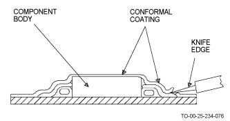
Figure 6-5. Removing Polyurethane Coating from Lead
