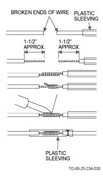
Figure 4-27. Splicing Broken Wire by Soldering
