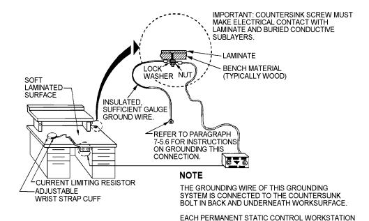
Figure 7-3. Permanent Static Control Workstation
