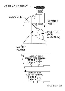
Figure 4-50. Hand Crimping Tool, Aluminum Terminals
