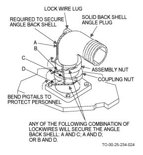
Figure 4-21. Safety Wiring AN Connectors
