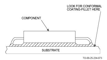
Figure 6-2. Conformal Coating Fillet
