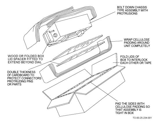
Figure 2-1. Chassis-Type Electronic Assembly, Protective Packaging
