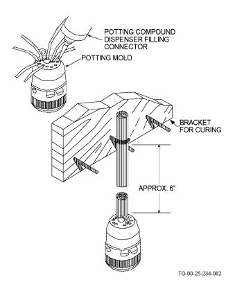
Figure 4-59. Filling and Curing Potted Connector
