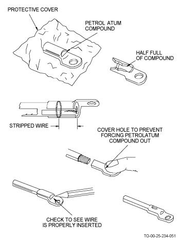
Figure 4-48. Inserting Aluminum Wire Into Aluminum Terminal Lugs
