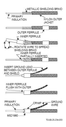
Figure 4-30. Grounding Sheath Termination for Shielded Wire
