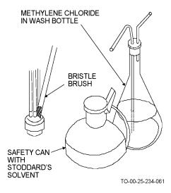
Figure 4-58. Cleaning Connector Prior to Potting
