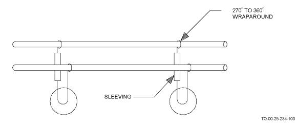
Figure 8-5. Buss Wire Connection
