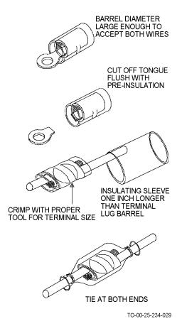
Figure 4-26. Terminal Lug Barrel Splice
