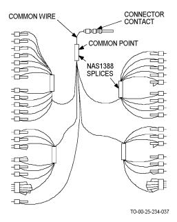
Figure 4-34. Typical Cascading Pigtails
