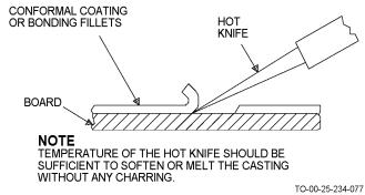
Figure 6-6. Removing Polyurethane Coating or Fillets
