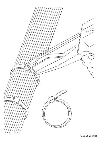
Figure 4-41. Installing Self-Clinching Plastic Cable Straps
