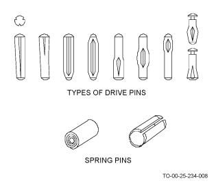
Figure 4-5. Typical Drive Pins and Spring Pins
