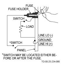
Figure 4-63. Correct Wiring of Instrument-Type Fuse Holder
