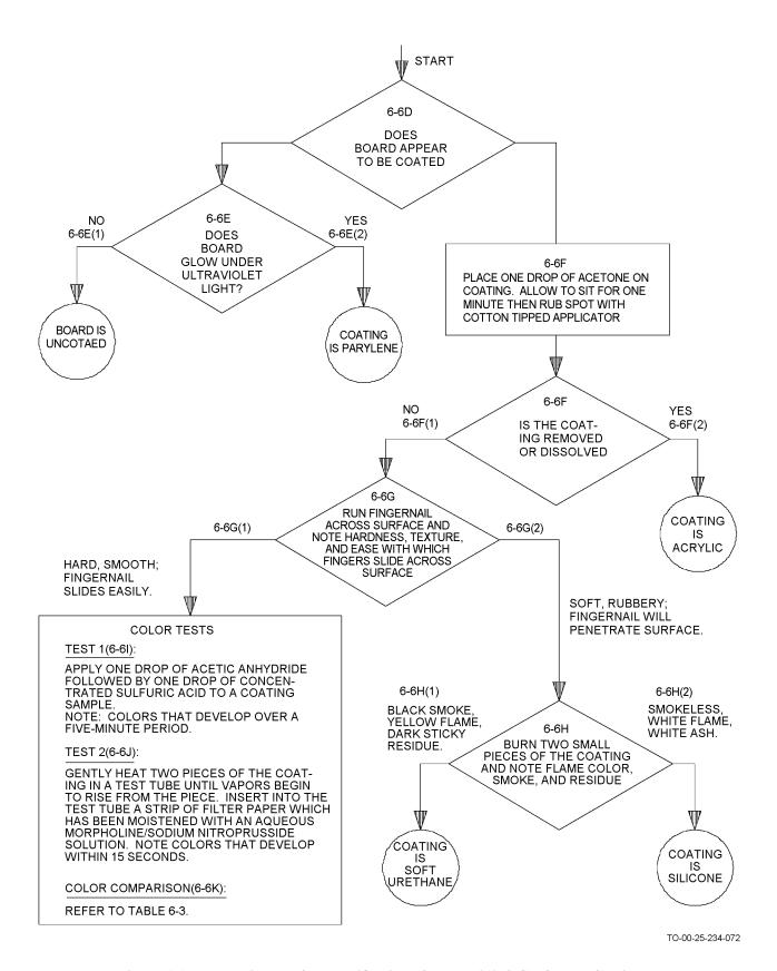
Figure 6-1. Flow Diagram for Identification of MIL-I-46058 Conformal Coatings
