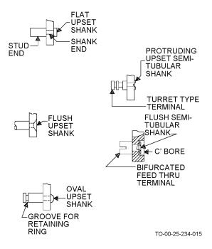
Figure 4-12. Typical Studs and Terminals
