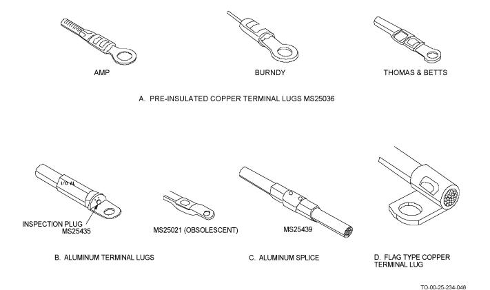
Figure 4-45. Solderless Terminal Lugs
