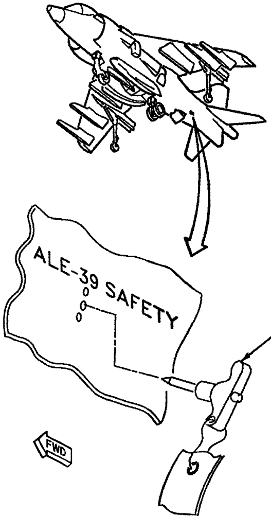
Figure 7-5. ALE-39 Ejector Rack Safety Pin
