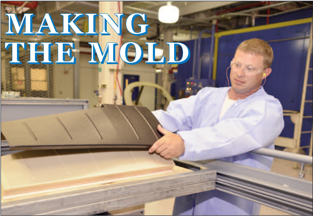
Above, Chad Lemoine, 573rd Composites Shop plastic worker, operates the base's new plastic thermo forming machine in Bldg. 670.
