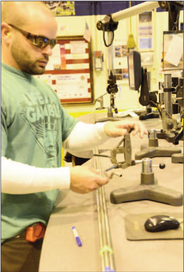
U.S. Air Force photo by RAY CRAYTON Hal Mickel, 402nd Commodities Maintenance Group, cuts tubing using the cut-off saw. where we streamlined getting the materials we needed. It’s a true suc-
