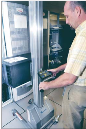
U.S. Air Force photo by SUE SAPP Luke Sarazine uses a powered lift to move a computer server into a shelving unit. One person can move a server with the lift where it took three people before to do it manually.
