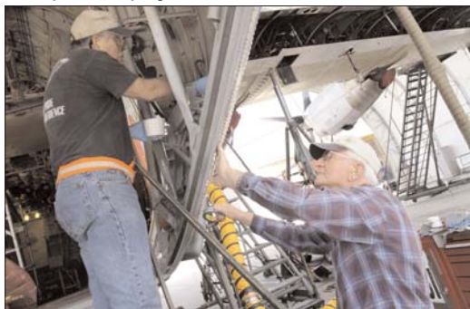
Above, Art Bazaruto and Jack Rogers, aircraft sheet metal mechanics, seal a skin on the C-130 undergoing the high velocity maintenance.
