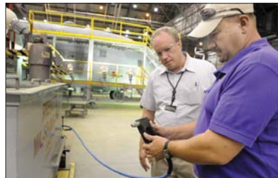
James Cranford and Todd Lavender look over a Prekote surface pretreatment vat. The treatment is less hazardous than previous methods.
