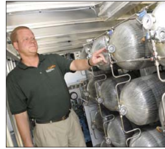
U.S. Air Force photo by SUE SAPP Scott Slyfield, Advanced Power Technology Office program manager, shows off the hydrogen storage tanks inside the HyHauler.
