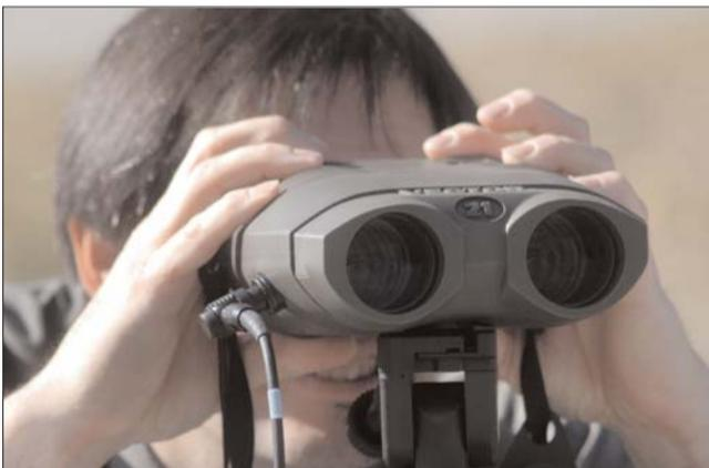
Frank Rowe, system engineer, uses a laser range finder to identify and locate a target using a VECTOR 21 LRF. When the unit locates a target the information can be sent to a combat aircraft in order to coordinate an attack.
