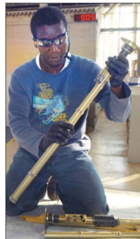
David Williams, aircraft mechanic, puts in a fuel quantity probe into a fuel tank on the C-130 wing.
