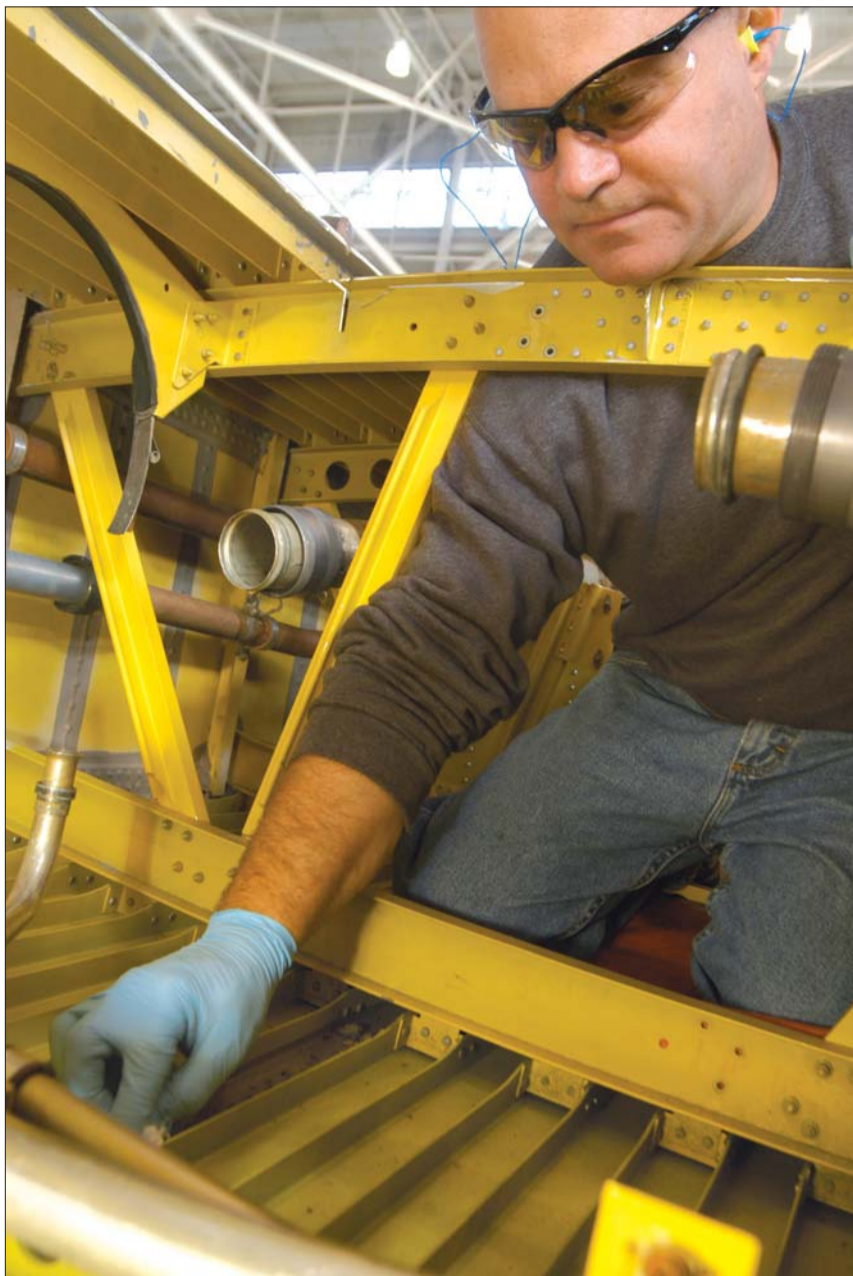
Michael Gayon, a C-130 maintainer, does a seal repair inside of a fuel tank on the C-130 wing.
