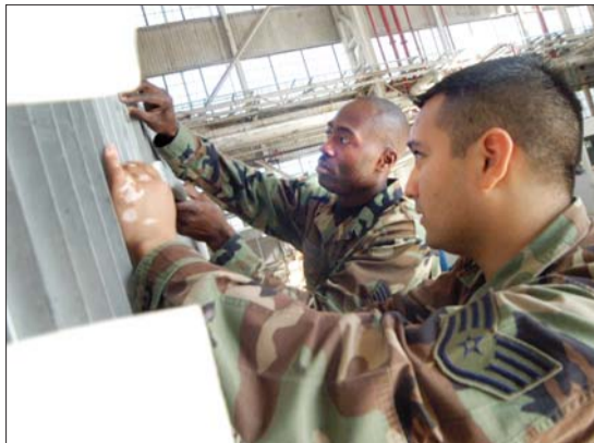
Staff Sgts. Wali Williams and Edgar Torres, 653rd Combat Logistics Support Squadron, replace an access panel on the C-130 wing that is used now for training.
