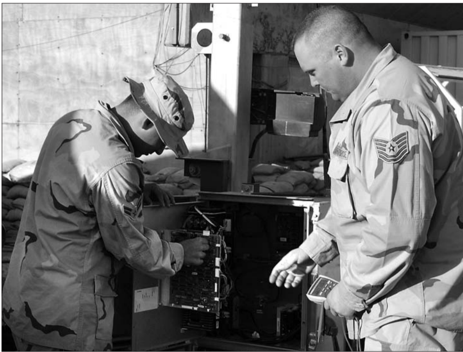
Airman 1st Class Mahendra J. Dataram and Tech. Sgt. Jeffery Jordan with the 5th Combat Communications Group, check the voltage on a Giant Voice System March 16, at Sather Air Base, Iraq. The GVS is used to address all commands and send messages to every individual in the area if there are intrusions in support of Operation Iraqi Freedom.
