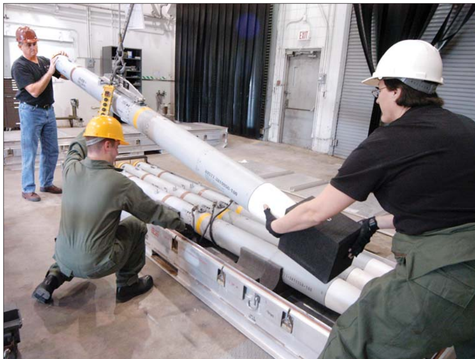
Above, Joe Harbin, Staff Sgt. Christopher Williams and Master Sgt. Patricia Logue load an AIM-120B onto a missile stand. U.S. Air Force photos by SUE SAPP
