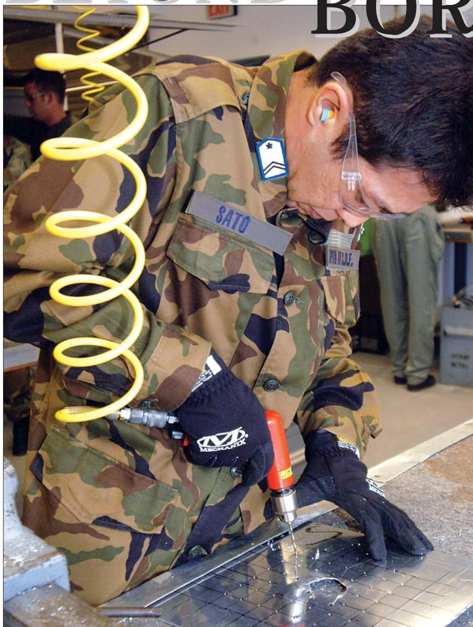
Tech. Sgt. Tatsuya Sato drills rivet holes in a simulated battle damaged piece of sheet metal so a patch can be attached. U.S. Air Force photos by SUE SAPP
