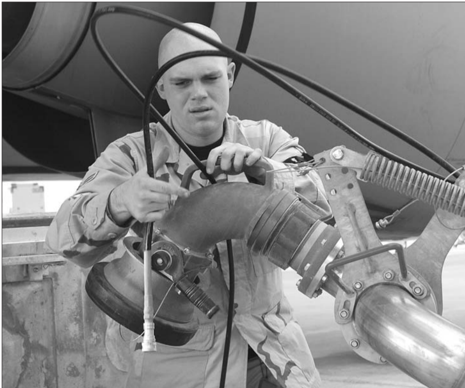
U.S. Air Force photo SENIOR AIRMAN ERIK HOFMEYER Airman 1st Class Robert Walsh prepares to refuel the first KC-135 Stratotanker through the new hydrant system Jan. 24 in Southwest Asia. Airman Walsh is assigned to the 379th Expeditionary Logistics Readiness Squadron Petroleum, Oil and Lubricants Flight.
