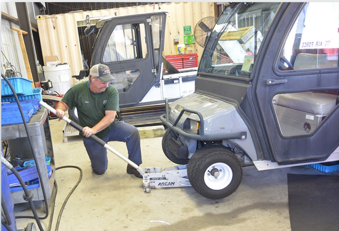
David Barrentine, 402nd Maintenance Support Squadron mechanic, jacks up a golf cart for to perform maintenance on its wheel and tire assembly. Complex golf cart sustainment was previously accomplished by contract until the 402nd Maintenance Support Group took over the workload in March 2016. In just one year, the crew had not just kept up with demand for the vehicles; it had vastly improved every facet of the operation. (U.S. Air Force photo/RAYMOND CRAYTON, JR.)
