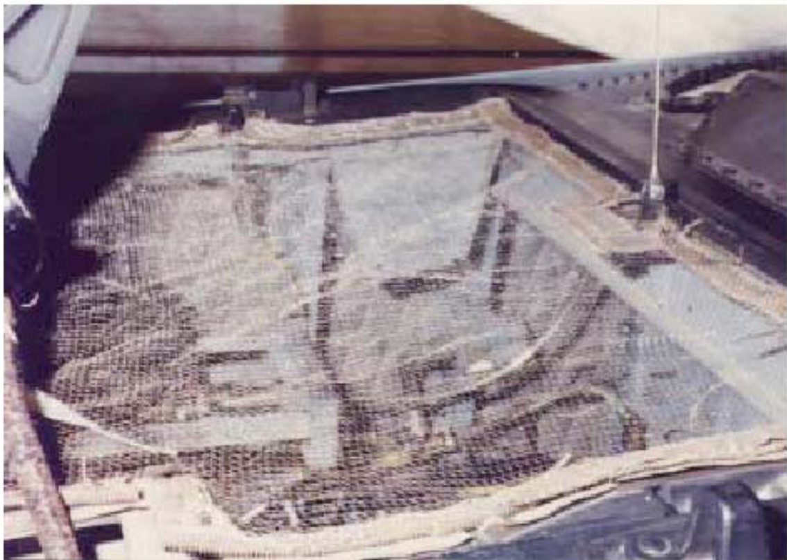
Figure 7-3. Stainless Steel (CRES) EMI Screen
