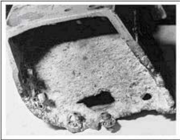
Figure 2-19. Magnesium Corrosion Products
