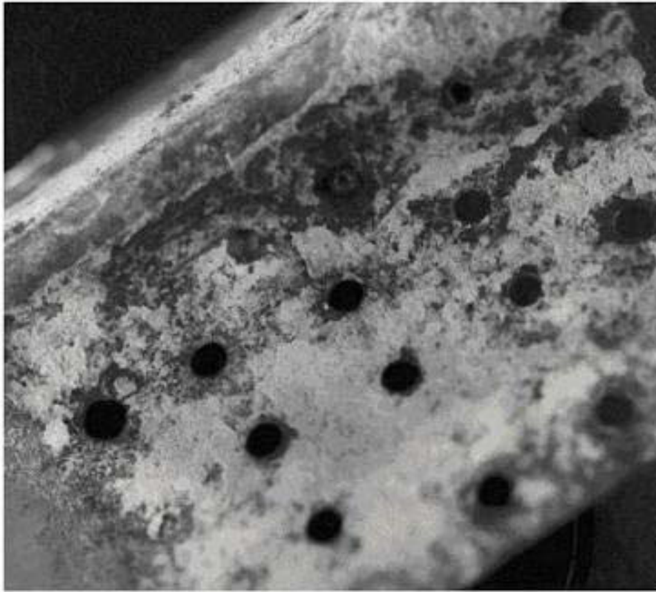
Figure 2-21. Aluminum Surface Corrosion Products
