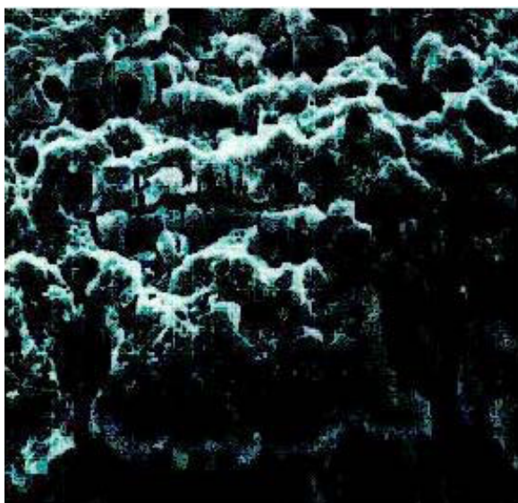
Figure 2-10. Grain Structure of a Corroding Aluminum Surface
