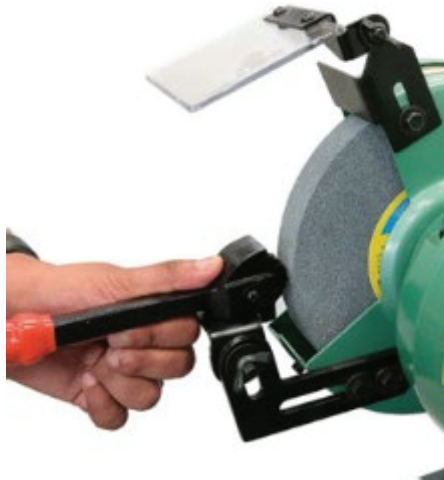
Figure 3-13. Hand Dressing a Grinding Wheel
