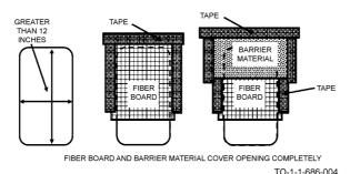
Figure 4-3. Sealing Openings Greater Than 12 Inches
