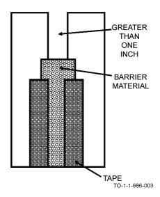
Figure 4-2. Tape and Barrier Material Application
