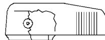
ONE CRACK EXTENDING ABOVE SET SCREW NOT PERMISSABLE. ONE CRACK BELOW SET SCREW PERMISSABLE.
