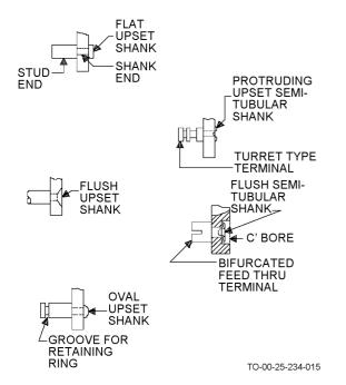
Figure 4-12. Typical Studs and Terminals
