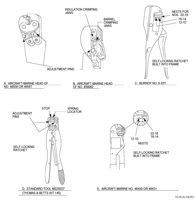
Figure 4-49. Hand Crimping Tools for Pre-Insulated Terminals
