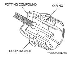
Figure 4-60. Installation of O-Ring on Potted Connector
