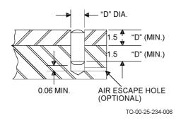
Figure 4-3. Application of Dowel Pin
