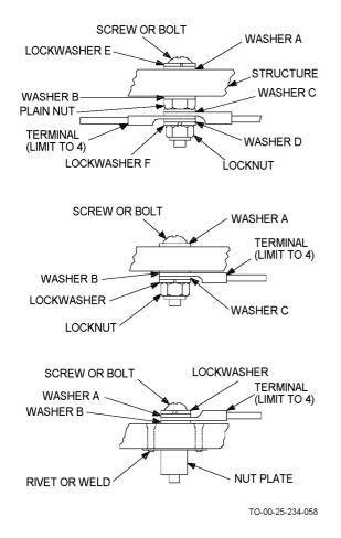
Figure 4-55. Typical Bolted Connections
