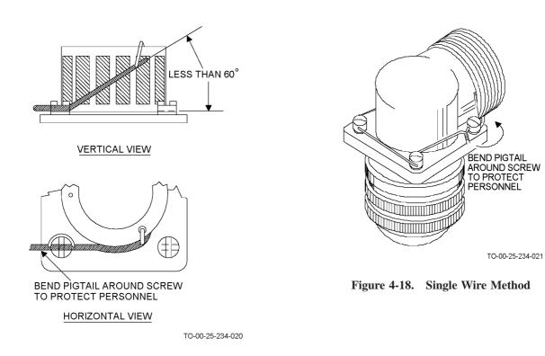
Figure 4-17. Double Twist Safety Wiring
