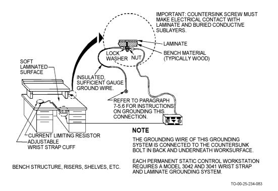
Figure 7-3. Permanent Static Control Workstation
