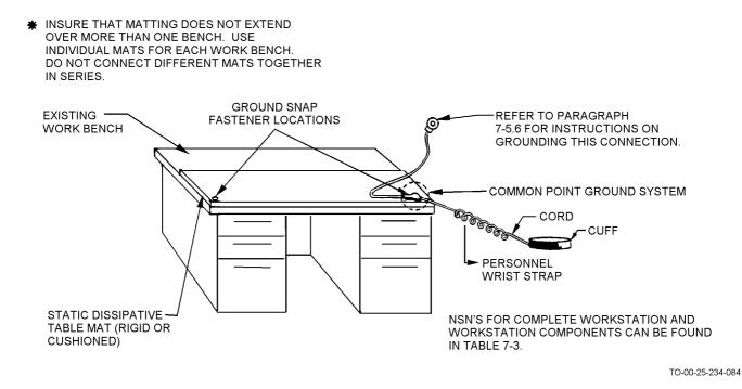
Figure 7-4. Static Control Workstation (work cushioned or rigid work surface on an existing work bench)
