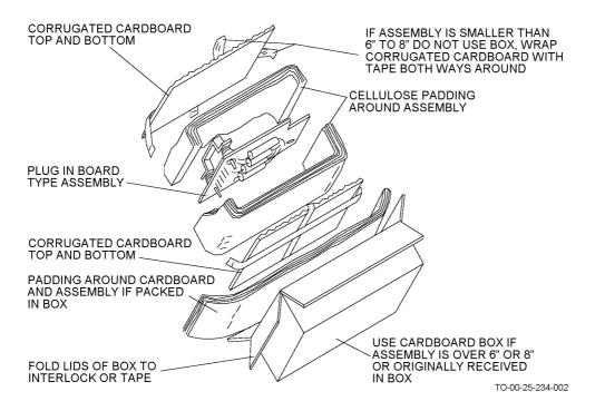
Figure 2-2. Circuit Board-Type Electronic Assembly, Protective Packaging
