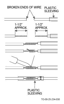
Figure 4-27. Splicing Broken Wire by Soldering
