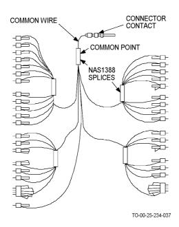
Figure 4-34. Typical Cascading Pigtails
