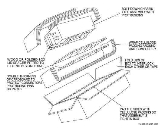
Figure 2-1. Chassis-Type Electronic Assembly, Protective Packaging
