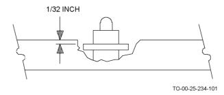
Figure 8-6. Typical Excavated Plug
