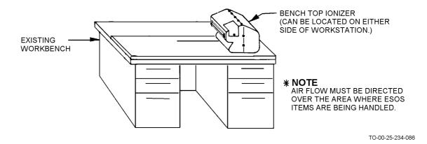
Figure 7-6. Bench Top Ionizer Positioning
