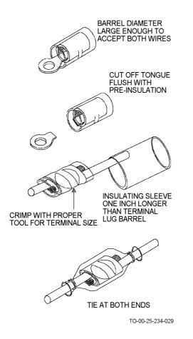
Figure 4-26. Terminal Lug Barrel Splice
