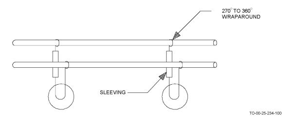
Figure 8-5. Buss Wire Connection
