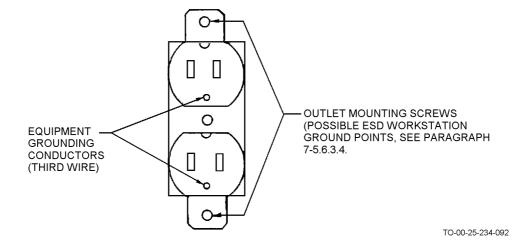
Figure 7-12. Typical Electrical AC Outlet
