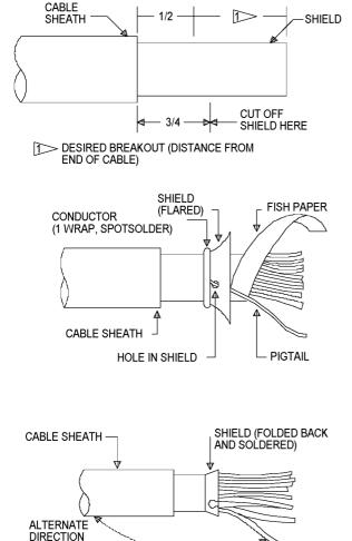
Figure 4-31. Soldered On Pigtail Preparation
