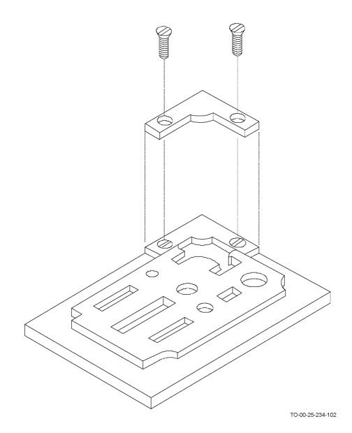
Figure 8-7. Front Panel Mold
