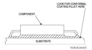
Figure 6-2. Conformal Coating Fillet
