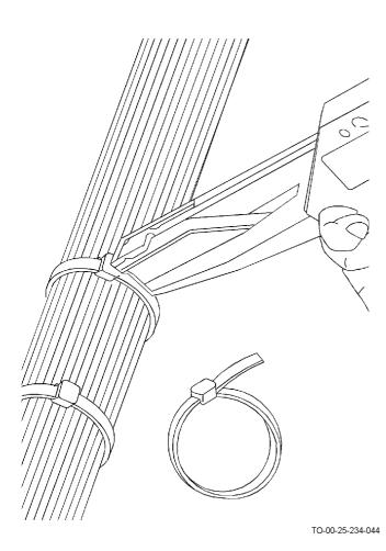
Figure 4-41. Installing Self-Clinching Plastic Cable Straps
