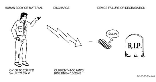
Figure 7-1. Reasons for Device Failure Due to ESD
