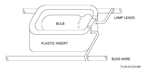
Figure 8-4. Typical Bulb Insert
