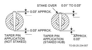
Figure 4-4. Application of Tapered Pins
