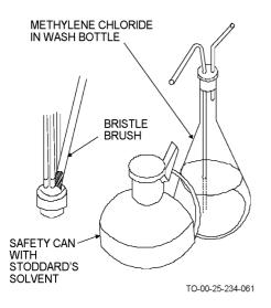
Figure 4-58. Cleaning Connector Prior to Potting
