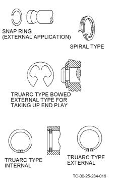
Figure 4-13. Typical Retaining Rings
