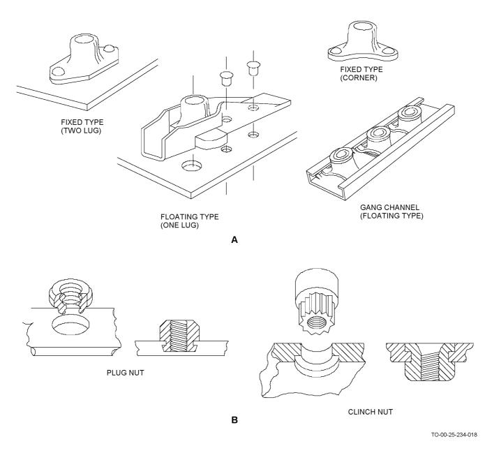
Figure 4-15. Anchor Nuts, Clinch Nut, and Plug Nut
