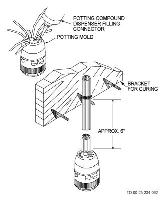
Figure 4-59. Filling and Curing Potted Connector
