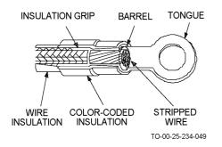
Figure 4-46. Pre-Insulated Terminal Lug Cutaway
