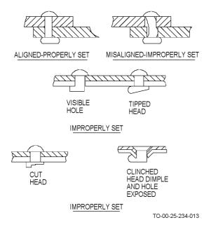
Figure 4-10. Properly and Improperly Set Rivets
