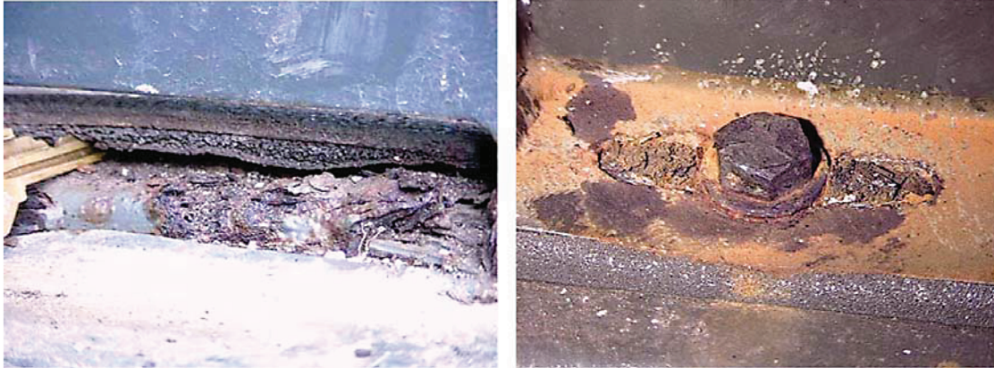
Figure 1-4. Open Cell Foam and Resulting Corrosion
