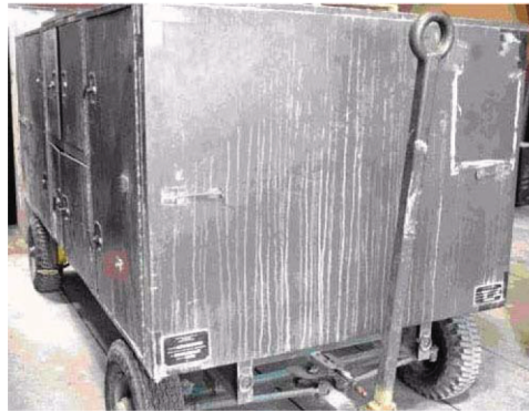
Figure 7-3. Residue from Salts Caused by Condensation
