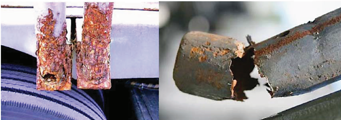
Figure 1-3. Corrosion Accelerated by Condensed Moisture
