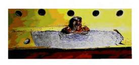
Figure 6-9. Exfoliation Corrosion
