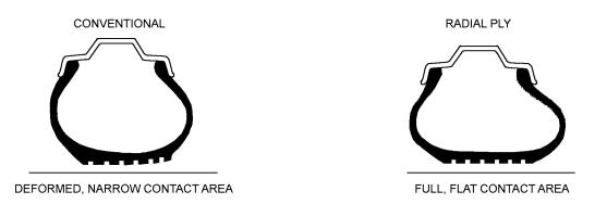
DIAGRAMS SHOW DIFFERENCES IN CONVENTIONAL BIAS PLY TIRES AND RADIAL PLY TIRES WHEN CORNERING. STIFF SIDEWALL OF CONVENTIONAL TIRE LIFTS PART OF THREAD OFF THE PAVEMENT. WHEN RADIAL IS PROPERLY INFLATED, IT RESISTS SUCH DEFORMATION DUE TO ALL OF TREAD AREA AND SIDEWALL, WHICH FLEXES MORE EASILY.
