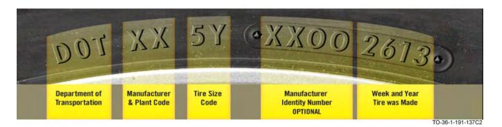
Figure 4-26. Tire Identification Number and Date of Manufacture Code
