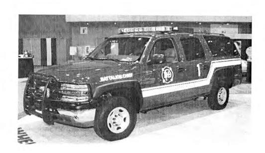
Figure 2-18. Angular Striping Example
