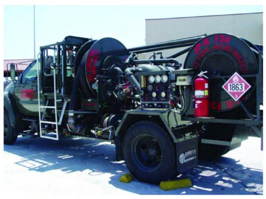
Figure 2-20. Hydrant Fueling Truck (Sheet 1 of 6)
