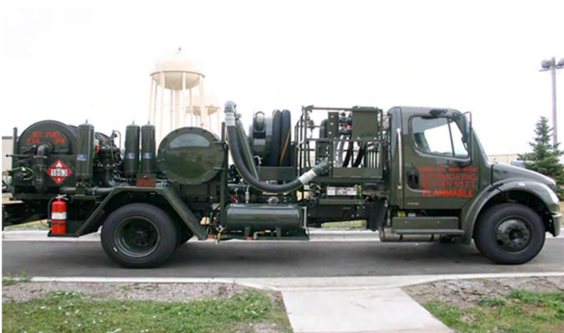
Figure 2-20. Hydrant Fueling Truck (Sheet 5)
