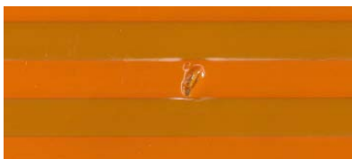
Figure 13-2 Flex Print Damage
