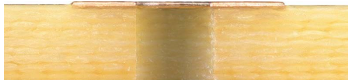
Figure 07-1 Single-Sided CCA (cross-section)
