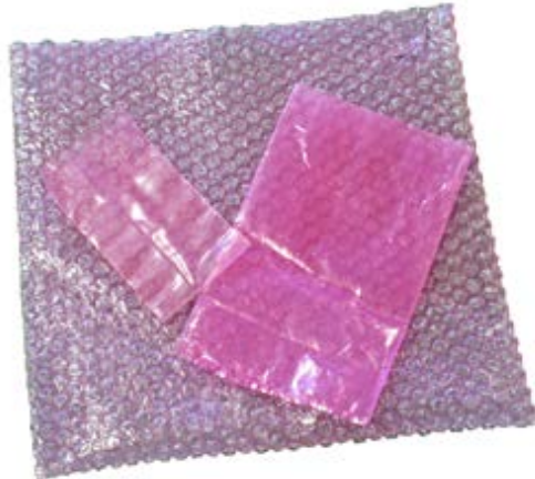
Figure 04-12 Antistatic ESD Protective Material (Pink Poly)
