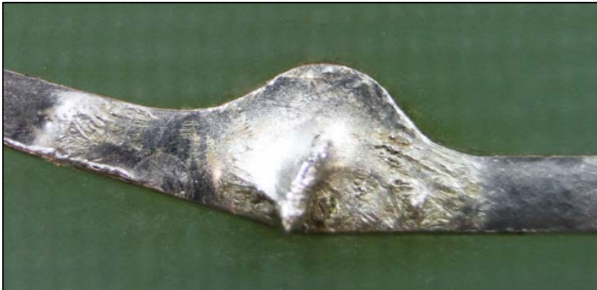
Figure 05-9 Overheated Solder Joint
