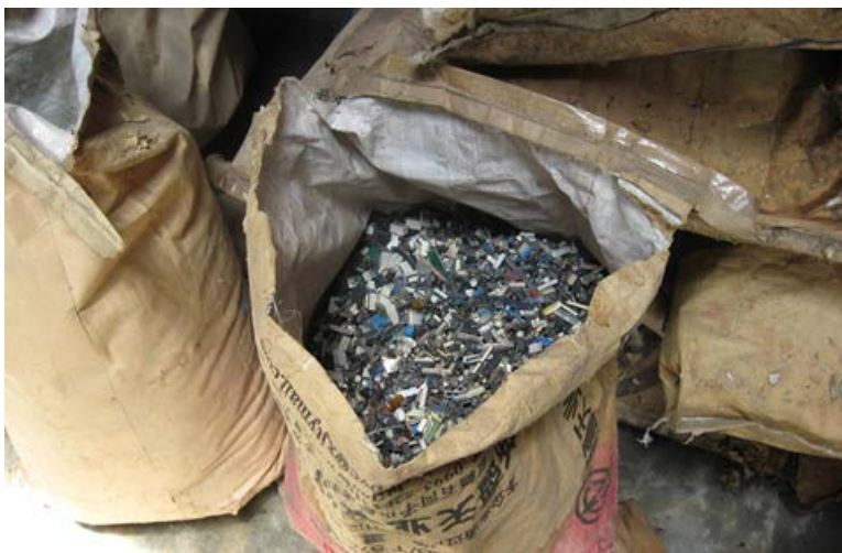
Figure 03-25: A bag full of harvested electronic components to be used in counterfeiting operations. Figure provided by SMT Corp.
