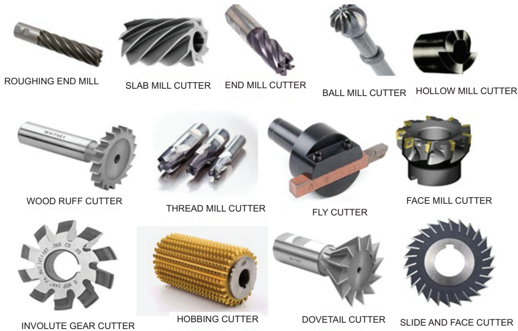
Figure 5-10. Types of Milling Cutters
