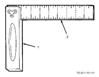
The try square is made of a steel or wood stock (1) and a blade (2). The blade is from 2 to 12 inches long and is graduated in eighths. The try square is used to set or check lines which are at right angles (90 degrees) to each other.
