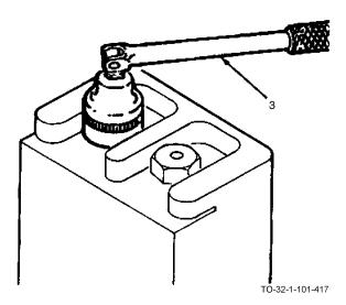
d. When a tight nut is to be loosened or a nut is to be set up, the nut hinged handle (3) can be swung at right angles to the socket to provide the most leverage. At the point where the nut turns easily, the handle can be swung to a vertical position and twisted rapidly between the fingers in the same manner as a screwdriver.
