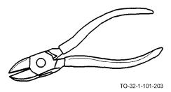
The diagonal cutting pliers have a fixed pivot. The jaws are offset by about 15 degrees and are shaped to give enough knuckle clearance while making flush cuts. The diagonal cutting pliers are used for cutting small, light materials such as wire, cotter pins, and similar materials. These pliers are not to be used to hold or grip objects.
