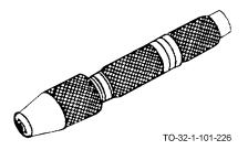
The pin vise is a special purpose vise which has a knurled metal handle and a chuck. It is designed to hold material from 0 to 0.187 inches in diameter. The pin vise is used to hold files, taps, and small drills during machining operations.
