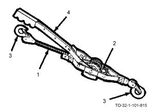
Like the cable jaw grip, the tension puller is used to tighten or stretch cables. The tension puller has strong cable (1) attached to a cable notch gear (2). At the end of the cable is a hook (3). This hook (3) can be attached to the eyelet of the cable to be tightened. Tension is then applied to the cable by moving the tension handle (4) in an up and down motion.
