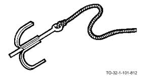
The trip wire grapnel is a metal weight resembling three or four fish hooks, with a common shank ending in an eye. The hooks spread out in different directions at the other end of the shank. Attached to the eye portion of the shank is a marlin cord of varying length. The grapnel is used to trip wires designed to go off on contact, to find booby traps, or to detonate mines.
