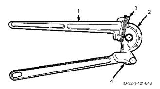
The hand tube bender consists of the following components: a handle (1), a radius block (mandrel) (2), a clip (3), and a slide bar (4). The radius block is graduated from 0 to 180 degrees, and the slide bar has a scribe mark which indicates the degree of bend. These benders are available in 3/16, 1/4, 5/16, 3/8, and 1/2 inch sizes. The hand tube bender is used to bend copper, brass, or aluminum tubing to specific angles.
