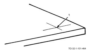
a. Mark the material to be punched with an "X" (1).
