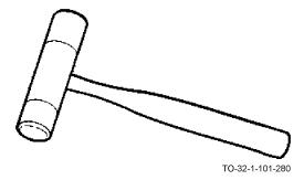
Soft-faced hammers are capable of delivering heavy blows to machined, highly polished or soft surfaces without damaging the surface.
