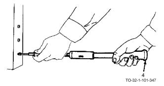
d. Insert the tip in the screw slot. Hold the screwdriver blade as shown. Move handle (4) back and forth to install or remove a screw.
