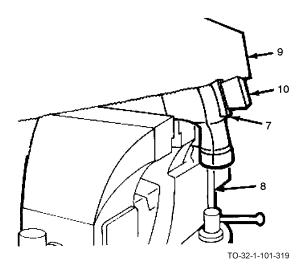
e. Place hammer (7) in vise (8). Using handsaw (9), remove projecting end of wedge (10).
