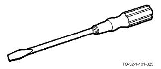
The common screwdriver has a round steel blade with a wood or plastic handle, usually fluted for a good grip. Integral blade screwdrivers are used for heavy-duty work.
