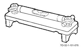
The iron bench level is made of a special design casting which insures its lightness, strength, and rigidity. It is used mostly in the construction industry. It may also be used in a machine shop.
