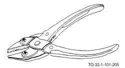
The parallel jaw pliers are constructed so that the jaws remain parallel to each other throughout the entire distance of travel. It has two jaws, a pivot pin, curved handles, and tension springs. The tension springs are contained within the curved handles and will open the jaws when the handles are released. These pliers are used to grip objects which have flat surfaces.
