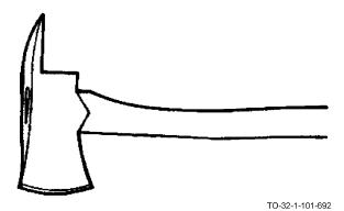
The crash ax, or fireman's ax, is used by emergency personnel to gain quick access to a given area. This ax has a steel head with a cutting blade or bit at one end, and a spike-like extension at the other.
