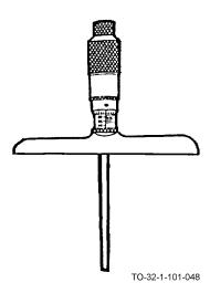
Depth micrometers are used to measure depths to an accuracy of 0.001 inches.
