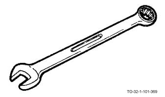
All open-end wrenches have open jaws on one or both ends of the wrench. Most jaw openings are offset from the shank portion of the wrench by 15 degrees. The wrench length is determined by the size of the jaw opening. Some of the more common types of open-end wrenches and their uses are listed below.
