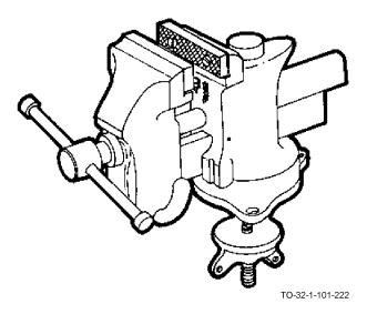
The bench and pipe vise is a dual purpose vise. It has rough jaws and a swivel base similar to the machinist's bench vise. However, it also has built-in pipe jaws. Bench and pipe vises are usually bolted to a work bench or table. They are used for holding or clamping heavy objects, holding pipe for cutting and threading, and for forming and shaping metal.
