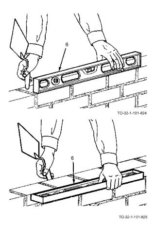
j. Lay enough bricks to cover the mortar bed and tap into line using a builder's level (6).
