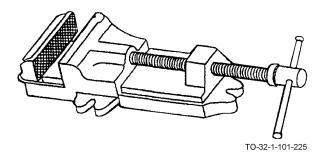
The machine table vise is a special purpose vise which may be bolted to a drill press, lathe, or table. It is available in two sizes, one having a 3-1/2 inch jaw width and a 3 inch jaw opening, and the other having a 6 inch jaw width and a 6 inch jaw opening. Machine table vises are used to hold small pieces of wood or metal for machining or drilling operations.
