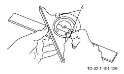
b. Loosen the protractor adjustment screws (4) so the protractor may be pivoted about the rule. Angle being measured is already marked.
