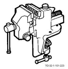
The clamp base bench vise is a lightweight, portable machinist's vise. It is attached to a table or bench with the mounting clamp. It has rough jaws for holding material and may have a swivel base. Clamp base bench vises are used to hold light materials or in areas where a heavier vise is not available.
