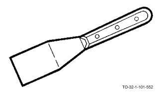
A putty knife is used for applying putty to window sashes in setting panes of glass. The blade has a wide square point and is available in different lengths and widths.
