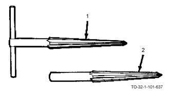
Pipe reamers are made of carbon steel. They are tapered with straight or spiral flutes. They come in three sizes, 1/8 inch to 1 inch pipe capacity, 1/4 inch to 1-1/4 inch pipe capacity, and 1/4 inch to 2 inch pipe capacity. Most pipe reamers are designed to receive a T-handle (1). Others (2) have a tapered square shank for use with a brace, or a round shank for use with a hand drill. They are used to remove burrs from the inside diameters of pipe and drilled holes.
