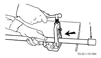
j. Place protective cap (1) on cut pipe end and remove from vise.
