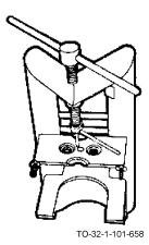
The electrical unit bearing puller is used to pull bearings from shafts of electrical units. It is supplied with plates to fit a variety of unit constructions and to fit behind the particular shaft bearings to be pulled.
