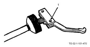
a. Select a punch having a smaller diameter than the smallest hole (1) to be aligned.
