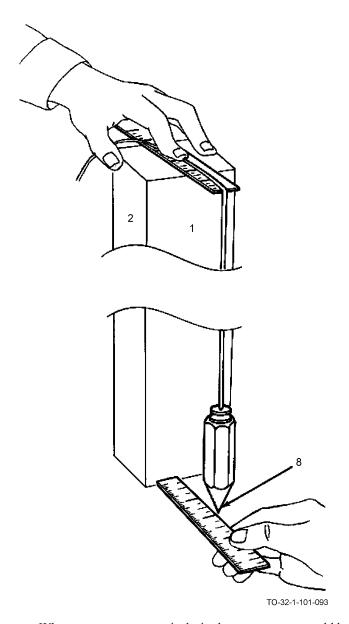
When extreme accuracy is desired, measurement would be taken to the point of the plumb bob (8). Repeat  $\underline{\underline{Step}} \, \underline{\underline{e}}$ , and  $\underline{\underline{Step}} \, \underline{\underline{g}}$  on side 2.
