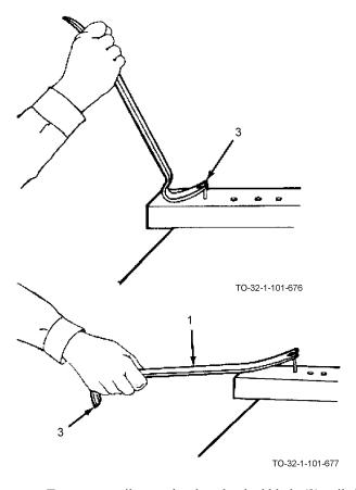
c. To remove nails, use the short hooked blade (3) nail slot to remove a nail that is almost completely driven home. Pull the nail approximately half-way out. Then switch to the long tapered blade (1) nail slot to completely remove the nail.
