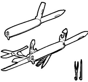
Pocket knives are used for light cutting, sharpening pencils, cutting string, and whittling. They are not suitable for heavy work. There are many styles and shapes. Some are multipurpose and have an assortment of blades which are used for forcing holes, driving screws, and opening cans, as well as cutting. The blades are hinged and contained within the case when not in use and are spring loaded to keep them firmly in place when open or closed.
