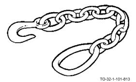
The chain assembly is a heavy duty linked chain with a grab hook at one end and a ring at the other. The chain assembly is used for such applications as towing vehicles, slinging loads, and hauling objects. The chain assembly is available in a wide variety of lengths and link sizes depending on the nature of the use.
