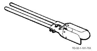
The posthole digger has two concave blades similar to the posthole auger except that each blade is fastened to a long, wooden handle. The blades are hinged at the top so that separating the handles will close them and moving the handles together will open them. Like the auger, the posthole digger is used to bore holes in the ground for posts, explosive charges and similar jobs.
