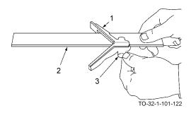
a. Slide center head (1) on rule (2) and fasten by tightening setscrew (3).
