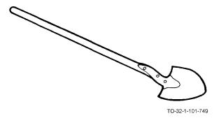
The long-handled shovel consists of a curved, shaped steel blade attached to a long wooden handle. The lower metal edge of the blade is tapered to help it cut into the ground. The longhandled shovel is used for heavy digging, especially when it is necessary to throw or move dirt a substantial distance.
