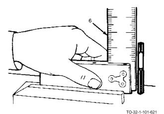
e. Remove tap wrench and, using a square (6), check tap for squareness. Check at least two different positions on the tap.
