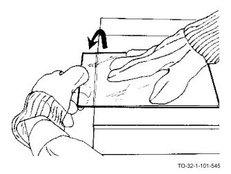
i. Hold down on the section resting on the working surface. Grasp the section extending over the edge with your other hand. Apply a light downward pressure to part the glass.
