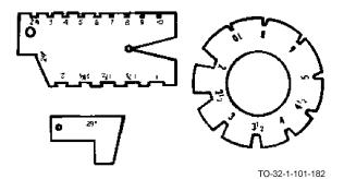
Thread cutting tool gages are hardened steel plates with cutouts around the perimeter. Each cutout is marked with a number that represents the number of threads per inch. These gages provide a standard for thread cutting tools. They have an enclosed angle of 29 degrees and include a 29 degree setting tool. One gage furnishes the correct form for square threads and the other for Acme standard threads.
