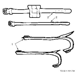
The leg irons (1) are often called tree and pole climbers. They consist of flattened metal bars, curved at one end to fit under the foot arch, and with the straight portion along the inside of the lower leg. Leather straps (2) secure the irons to the leg and ankle.
