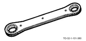
Ratchet-box wrenches are either reversible or nonreversible. The ratchet-box wrench does not have to be lifted up and repositioned each time the shank has reached its maximum travel between two obstructions. The ratchet-box wrench provides an easy means of removing and/or installing nuts or bolts which are not under strain. These wrenches should not be used to torque down or to free nuts or bolts.
