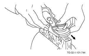
d. Push along the length of the board with a steady, even stroke.
