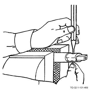
c. Catch the pin before it falls out of the shaft. When the pin is about half way out of the shaft, you can let go of the punch.
