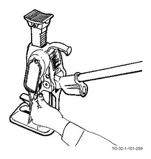
c. To lower a load, push reversing lever to straight-down position and operate the lever. The jack will lower the load one notch for each upstroke of the lever.
