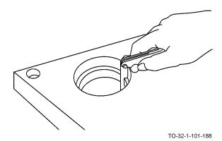
Thickness (feeler) gages are used in one of two ways: as a means for determining a measure or a means for adjusting to a definite limit. A thickness gage is used to check piston ring gap clearance in a cylinder bore.
