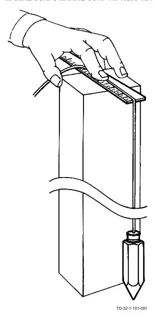
g. Have the assistant measure distance (7) from post to string just above the plumb bob. It should read 2 inches. If it doesn't, move the base or the top of the post right or left until you get a 2 inch reading on both rules.
