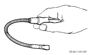
A flexible screwdriver has a spring steel blade which bends, allowing the user to get around flanges, shoulders, and other parts to drive and remove screws.
