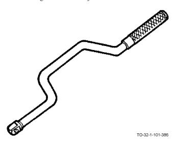
The speed handle has a brace-type shaft with a revolving grip on the top. It is used for rapid removal and/or installation of nuts or bolts, which are out in the open and have little or no torque.
