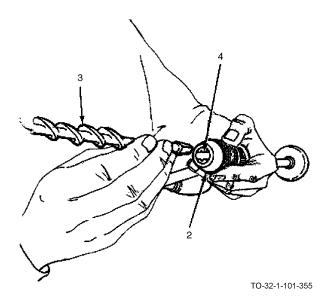
b. Open chuck (2) and insert bit (3) between jaws (4). Tighten chuck (2), securing bit (3).
