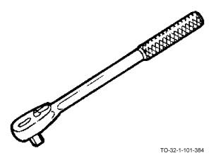
Ratchet handles may have either a straight-head or a flex-head. Both types have a selection lever on the top of the head to determine the direction of drive. The flex-head is used to go around objects. Both types are used with socket wrenches for rapid removal of nuts or bolts.
