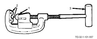
There are two sizes of pipe cutters. One size can cut from 1/8 to 2 inches, while the other can cut from 2 to 4 inches. The pipe cutter has a cutting blade (1) and two pressure rollers (2) which are adjusted and tightened by turning the handle (3). Pipe cutters are used to cut steel, brass, copper, wrought iron, and lead pipe.
