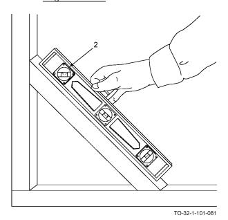
Place the level on an angled surface. If the angle is 45 degrees, the bubble will appear between the notched lines on the 45 degree vial (2).
