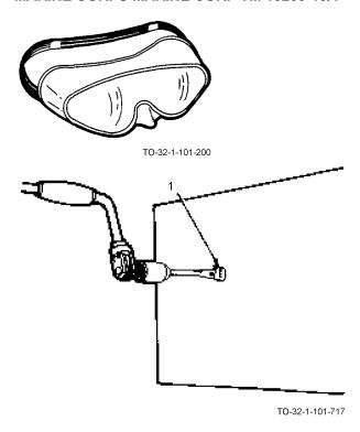
a. To make an inside-out cut, first drill a hole (1) large enough to admit the point of the saw.
