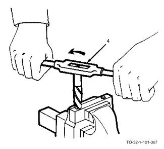
c. Remove the broken screw by turning the extractor counterclockwise. The extractor may be turned using a tap wrench or open end wrench (4).
