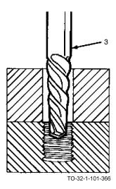
b. Insert extractor (3) in the drilled hole.
