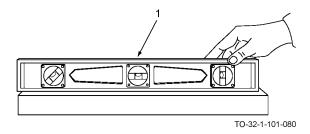
Place the level on a flat horizontal surface. Check the horizontal vial (1). The bubble should be between the two etched lines on the vial. If it is not, the surface is not horizontal.
