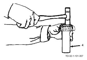
j. While supporting bearing with left hand, use soft-faced hammer to tap in a circular motion until edge of bearing is flush with shaft (4).
