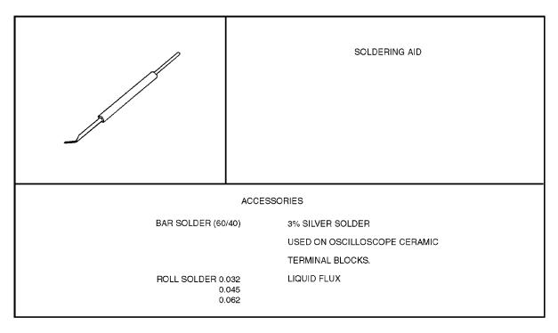
Figure 53-1. Soldering Tools and Accessories (Sheet 4)
