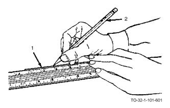
a. Place the wire (1) on the table. Measure the section to be cut off. Mark it with pencil, chalk, soapstone or other suitable marking piece (2).
