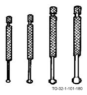
Small hole gages are adjustable, having a rounded measuring member. A knurled screw in the end of the handle is turned to expand the ball-shaped end in small holes and recesses. A micrometer caliper is used to measure the ball end. Maximum measuring capacity is 1/2 inch. This set of 4 or more gages is used to check dimensions of small holes, slots, grooves, and so forth from approximately 1/8 to 1/2 inch in diameter.
