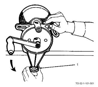
c. Position grinder where it will be used and tighten the mounting clamp (1) to hold securely on the bench.
