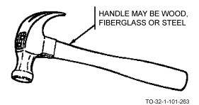
The carpenter's hammer is used for driving and pulling nails and tapping wood chisels. There are two types of claws.
