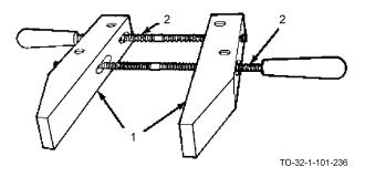
The hand screw clamp is made up of two hardwood or high impact plastic jaws (1) and two hand-operated screws (2) which hold the clamp together. The hand screw clamp is used for holding wood while gluing. They are available in a variety of sizes.
