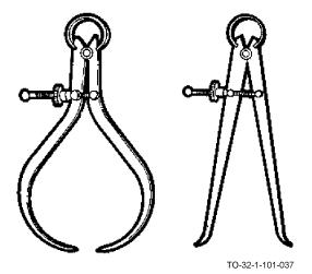
The spring-joint calipers have the same type of legs, but are joined by a strong spring hinge, screw, and adjustment nut.
