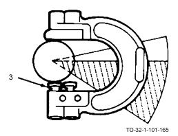
b. If the shaft is not oversized, the first button (3) will pass over it easily.
