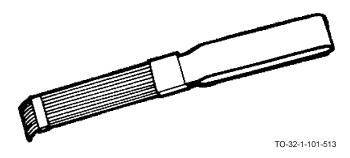
A carbon scraper is used to clean carbon from cylinder heads, pistons, and other metal surfaces. It is flexible and has an overall length of approximately 9 inches. The carbon scraper consists of ten round spring steel blades, and their flexibility is controlled by a sliding ferrule.
