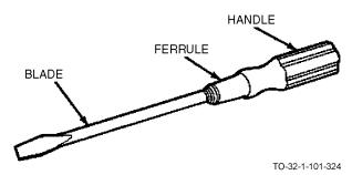
Screwdrivers are available in many different shapes, sizes, and materials. Screwdrivers are used for driving or removing screws or bolts with slotted, recessed, or special heads.
