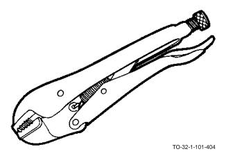
The clamp pliers are generally used more as a wrench than as a pair of pliers. It has a fixed jaw and handle which contains an adjustment screw for the movable jaw. The other handle is in two sections, one section to apply pressure and to lock the pliers, and the other section, when pulled, to release the grip. Clamp pliers are used to hold or clamp nuts and bolts which have been
