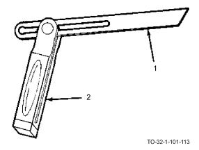
The sliding T-bevel is made up of a slotted blade (1) and a solid stock (2). The blade is adjustable so it can be set to measure any angle. The T-bevel is used for testing bevels and laying out angles.
