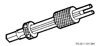
The tap extractor is usually of the flute type and requires the use of a wrench to turn the tap. It is used for removing taps with no external area.
