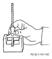
Measuring the distance from a surface to a recessed point.
