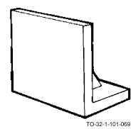
Angle plates are devices consisting of two flat outside working surfaces jointed at right angles. The outside work surfaces are precision ground. The standard angle plate is permanently jointed at a right angle. However, an adjustable type with varying angle adjustments is also available. Angle plates are used for clamping or holding work vertically. They are also used for layout, inspection, or machine set-up. Various sizes and designs are available depending on the task.
