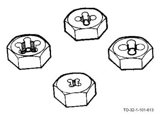
Rethreading dies are used to restore bruised (rounded) or rusty threads on screws and bolts. The rethreading die is hexagonal in shape and may be turned with a socket, box, open-end, or any other wrench that will fit. They are available in American Coarse and Fine Threads. Rethreading dies are available in a variety of sizes and are usually assembled in sets with a case.
