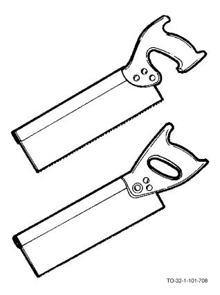
The backsaw has a straight blade and parallel top and bottom, with a heavy strip of steel or brass wrapped along the back to provide rigidity. The handle is of similar shape to other hand saws except it is usually mounted higher. Backsaws are used for general bench work such as cutting joints and smaller sections of lumber to length. Sizes vary depending on design and nature of work.
