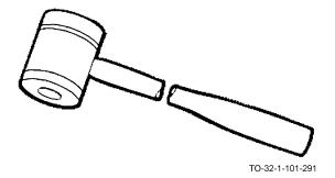
The wooden maul has a cylindrical head which is about 8 inches in diameter and about 10 inches long. It is used to drive wooden pickets, posts and stakes.
