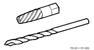
The spiral-tapered type requires a twist drill for drilling a pilot hole.
