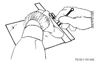
f. Start your cut at the far end of the pane of glass drawing the cutter toward you. It is important that you maintain proper pressure throughout the cut. Correct pressure is indicated by a scratching sound. Too much pressure or a dull wheel will produce a crunching sound. Make a continuous mark from one edge to the other edge.
