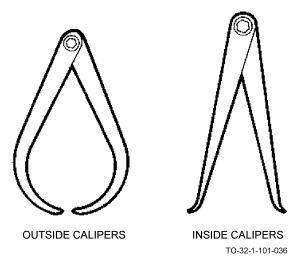
The simple outside calipers are bowlegged. Those used for inside diameters have straight legs with feet turned outward. Calipers are adjusted by pulling or pushing the legs to open or close them.
