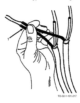
a. Using one hand, hold wires to be twisted (1) just above the point where the twist is to begin.
