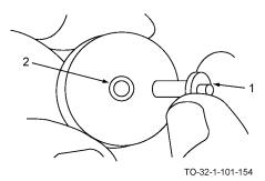
a. Line the stud (1) up with the hole (2) and press in gently. If the stud will not go in, the shank is too large. If it will go in, the stud is not oversize.
