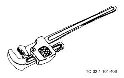
The stillson pipe wrench has a fixed jaw which is on the end of the handle and an adjustable jaw at the top of the wrench. Adjustment is made by turning a knurled adjusting screw which moves the jaw. Always pull the pipe fitting towards the fixed jaw. The serrated (grooved) jaws of the stillson wrench will mar soft pipe.
