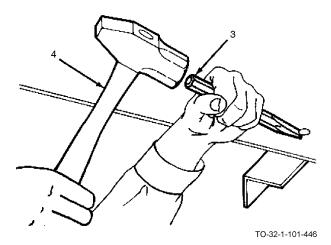
b. Grip the chisel firmly and strike chisel head (3) with a machinist's or sledge hammer (4).
