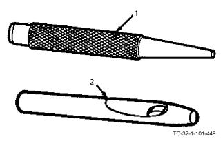
27.2.1 <u>Center Punches</u>. There are two types of center punches, both used for starting drill holes.
