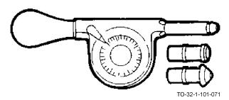
Registering speed indicators are designed to count the number of revolutions of wheels, shafts, etc. Revolutions are counted by attaching spindle of speed indicator to hub of shaft or wheel. Indicator spindle will turn in either direction counting each revolution on a circular dial. Various designs of speed indicators are available depending on nature of use.
