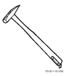
The trimmer's hammer has a round flat face on one end of the head and has a tapered chisel face on the other end. A claw is attached on the end of the handle and is used for pulling tacks. It is used for installing tacks and brads.
