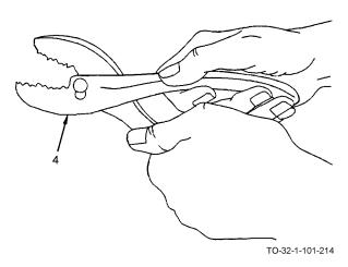
c. Adjust pliers (4) to obtain a wide jaw opening.
