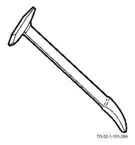
The welder's hammer has one or two tapered chisel faces. Those having only one tapered face have a replaceable brush attached. The hammer face is used for chipping welds, while the brush is used for cleaning welds and brushing away the slag chipped from the weld.
