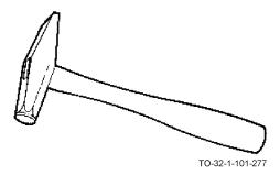
The riveting hammer has a round face on one end of the head. It is used for peening rivet heads. The other end has a tapered chisel which is used for upsetting rivets.
