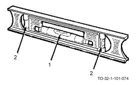
The master precision level has a ground and graduated main vial (1). The top and bottom of the level are milled and ground to make sure both surfaces are absolutely parallel. This level is used to determine the true horizontal with the main vial (1). The true vertical is determined by using the two smaller vials (2).
