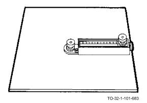
The compass-style circle gasket cutter cuts gaskets from 4 inch diameters through 20 inch diameters. It cuts leather, paper, plastic, rubber, sheet lead, or thin wood. It has an aluminum frame with a graduated scale, steel pivot pin, and tempered tool steel knives. It requires a knurled thumb screw adjustment to change diameters.
