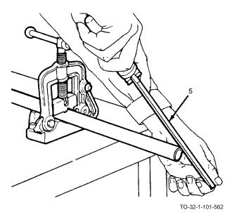
h. Remove the shoulder (the rough edge left by cutting) from the outside of the pipe with a file (5).
