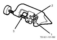
Tube cutters have a cutting blade (1), guide rollers (2), and an adjusting screw (3). Some cutters have a reaming blade attached to the frame of the cutter. Tube cutters can cut from 1/8 inch through 2-5/8 inches tubing. They can cut copper, aluminum, or brass tubing.
