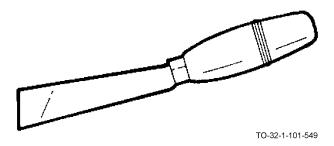
Saddler's knives are used on leather and come in different shapes. One has a broad point on a 1-1/8 inch by 5 inch blade. One has a 5/8 inch by 3-7/8 inch square point blade. Another has a 5 inch rounded-end blade. Shoe knives are similar to saddler's knives, but usually they have a 3/4 inch by 3-1/4 inch blade.
