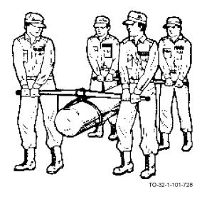
Lifting and moving heavy log with timber carriers.
