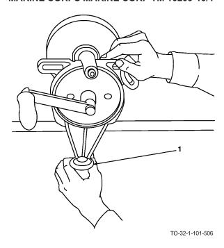
i. When the desired edge is obtained, you are finished. Remove grinder from bench by loosening the clamp (1). Store grinder in its designated storage area.
