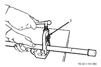
b. Fasten pipe securely in a pipe vise (2). Be sure mark is clear so that it can be cut. Pipe must be supported on both ends to keep it from bending.
