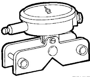
The magnetic base indicator holder is a one-piece metal assembly that attaches to the work surface magnetically. A gage or indicator attaches to the assembly. Base indicator holders are used for attaching gages to lathes, milling machines, shapers, or any machine where graduations are difficult to read. Magnetic base indicator holders are available in many sizes and designs depending on application.
