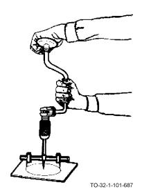
Cutting smaller circular gasket with a bit brace.
