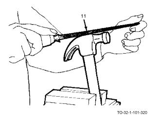
f. Remove excess portion of wedge using wood rasp (11).
