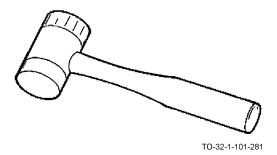
Lead or copper hammers are usually used for aligning steel surfaces. Copper hammers range in head weight from 8 ounces up to 3 pounds. Working surfaces of lead and copper hammers may be filed to restore even faces. Molds are available for repouring lead hammers.
