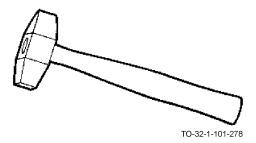
The sawmaker's hammer has a tapered blunt face on one end of the head and a tapered chisel face on the other end. It is used for setting the teeth on saws when a setting tool is unavailable.
