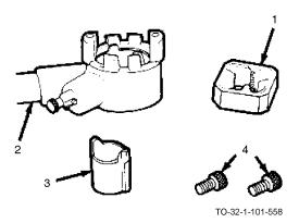
The pipe threading set contains an assortment of cutting dies (1), a handle or wrench (2), a collar (3) and locking screws (4). The cutting dies may range from 1/8 inch to 2 inches in diameter. The threading set is used to cut American Standard Pipe threads on steel, brass, copper, wrought iron, and lead pipe.
