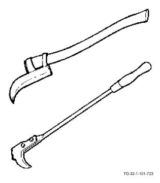
47.2.2 <u>Machete</u>. The machete normally in military use is an 18 inch knife, widest and heaviest at the point of the blade. The blade is attached to a handle shaped to fit the hand. The handle is designed with a slight projection to prevent the machete from slipping from the hand while being used. The machete is used to cut tall grass, vines, and small brush.
