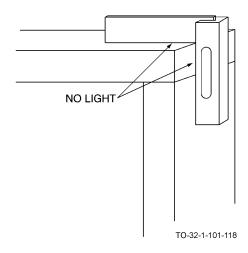
b. To check the end of a board, place stock on vertical edge and extend blade over the end. Light must not be seen around blade edge. If light is seen, the work is not square.
