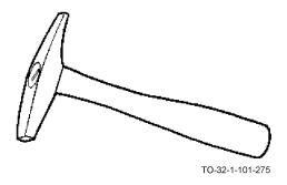
The mason's hammer has a flat striking face on one end of the head and a tapered chisel on the other end. It is used for setting and cutting bricks and flat stones.
