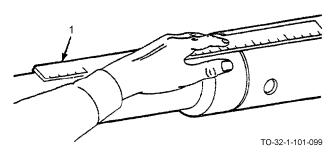
a. Place material to be marked on a firm surface. Place a steel rule or straight edge (1) on the work beside the line to be scribed.
