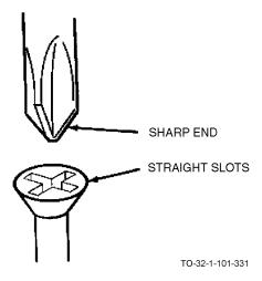
Cross-point screwdrivers are similar to the cross-tip. The cross-point slots meet at an exact right at angle at their intersection. These screwdrivers are issued in 3 to 8 inch sizes.
