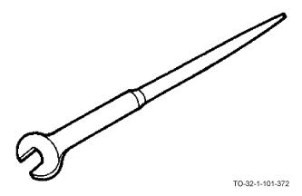
The construction wrench combines the open-end jaw with along tapered shank providing a wrench/alignment punch combination. The construction wrench is used in the building trades and on heavy objects which require alignment before fastening.
