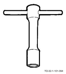
The T-handle socket wrench has a fixed T-handle above a fixed socket wrench. The T-handle socket wrench has many uses. One of the more common uses is for shutting off or turning on water or gas lines. The T-handle permits the operator to apply the turning force required to operate the valve.
