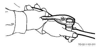
a. Broken or chipped faces may be removed by turning in a counterclockwise direction.
