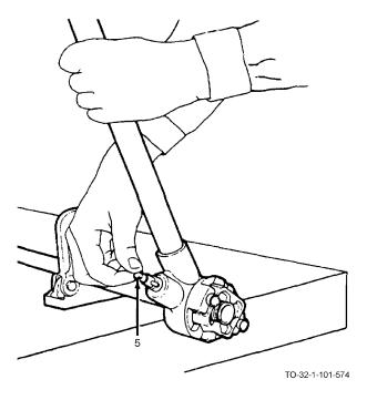
n. Reverse ratchet by pulling ratchet control knob (5) from detent and turning it 180 degrees. Then back up the cutting die.
