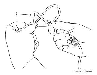
b. Place cap in the palm of your hand and tie an overhand knot (3) in the cord. Pull the cord drawing the knot against cap base. Make sure the knot is not too large or tied at an angle which would affect the hanging of the plumb bob.
