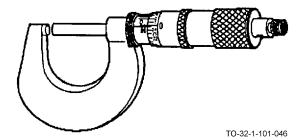
Outside micrometers are used to measure an outside distance or diameter to an accuracy of 0.001 of an inch.
