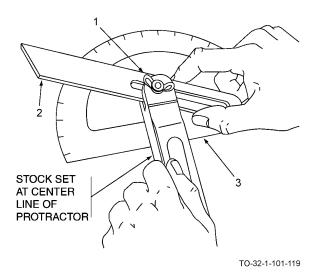
a. Loosen locking nut (1) and adjust blade (2) to measure a desired angle using protractor (3). Tighten locking nut (1).
