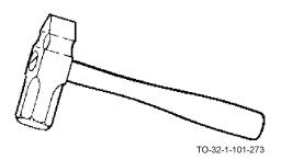
The straight peen is similar to the cross peen except that its peening edge is turned ninety degrees. This keeps the handle parallel to the struck surface.
