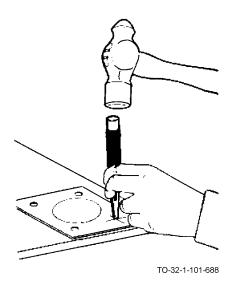
Cutting small holes in gasket with a hollow punch.
