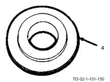
Ring gages are used more often in the inspection of finished parts than parts in process. The reason for this is that the finished parts are usually readily accessible; whereas, parts in a machine that are supported at both ends would have to be removed to be checked.
