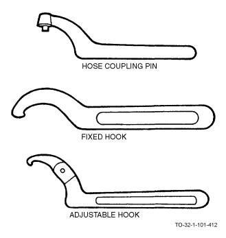
Three kinds of hook-type wrenches include the hose coupling pin, for tightening and loosening hose couplings, the fixed hook, for tightening or loosening couplings with protruding rims or edges, and the adjustable hook-type. The adjustable hook-type is similar to the fixed hook-type. However, it may be adjusted around objects and fastened before use.
