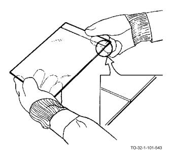
g. A proper cut is indicated by a slight crack in the surface. It is best seen from the side opposite the mark.
