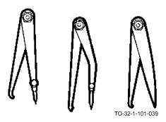
The hermaphrodite calipers have one straight leg ending in a sharp point. On some models this point is removable. This leg is usually bowlegged. This caliper is used for finding shaft centers or locating shoulders.
