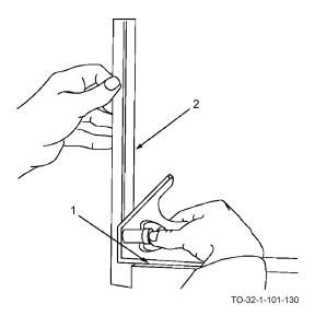
c. Set the flat surface of the square head (1) above the hole and adjust the rule (2) until it hits the bottom.
