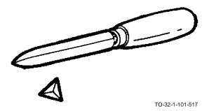
Triangular blade scrapers are used for removing high spots from flat or curved surfaces. They are available with either a 4 or 6 inch blade.
