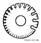
A wire gage is circular in shape with cutouts in the outside edge. Each cutout gages a different size wire, from 0 to 36 of the English Standard Wire Gage. A separate gage is used for American standard wire and another for U.S. Standard sheet and plate iron, and steel. Similar gages are also used to check the size of hot and cold rolled steel, sheet and plate iron, and music wire.
