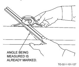
c. Place the rule on the angle being measured and pivot the protractor head against the edge. Tighten adjustment screws.
