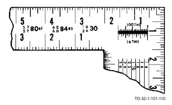
The brace measure is used to find the exact lengths of common braces. The following scales or inch divisions are found on the carpenter's square:
