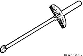
A scale torque wrench has a rod which runs parallel to the handle and the drive element. This rod moves across the scale to the right or left as torque is applied.
