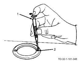
a. Hold screwdriver as shown, with forefinger on rotating head (1).
