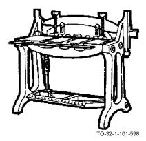
The metal shearing machine is foot-operated and is used to cut original sheets into smaller, usable size stock. The shear blade is 36 inches long and will cut all sheet metal up to and including 1/16 inch of mild steel or 1/8 inch of iron.
