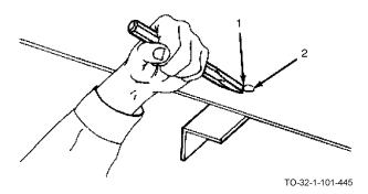
a. Place cutting edge (1) of the chisel firmly against the rivet shaft (2) between the head and the metal.
