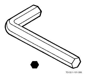
The hexagon key wrench is an L-shaped, six sided wrench. Both ends of the "L" are the same size so you can turn the wrench either to gain access to the screw head or to obtain a leverage advantage. The hexagon key wrench is used to remove and/or install hexagon head screws.
