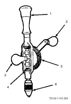
The hand drill is made up of the following parts: handle (1), drive handle (2), side handle (3), pinion (4), gear wheel (5) and chuck (6). The handle provides a storage area for drill bits. The side handle may be used to steady the drill when drilling in soft wood. The pinion turns the chuck and drill. Through mechanical linkage, the gear wheel transfers the driving force from the drive handle to the chuck. Hand drills are used to drill holes in wood and sheet metal.
