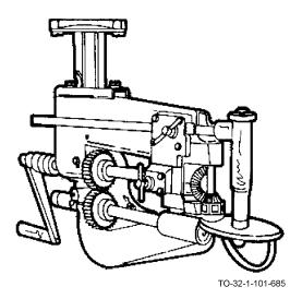
The bench mount gasket cutter is used for heavy duty jobs requiring gaskets cut from the heaviest of materials.
