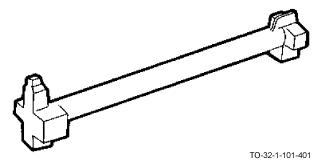
The multiple plug wrench combines several plug ends on a common handle.
