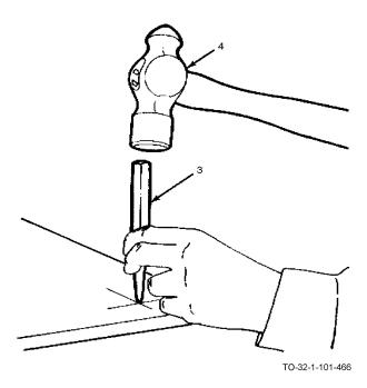
c. Position the punch upright and strike the blunt end (3) of the punch with a hammer (4).
