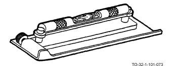
The machinist's level has an extra large vial. This increases its accuracy and sensitivity. Some of these levels have grooved bottoms which fit over pipes and shafts. They are used in machine shops for leveling work and equipment.
