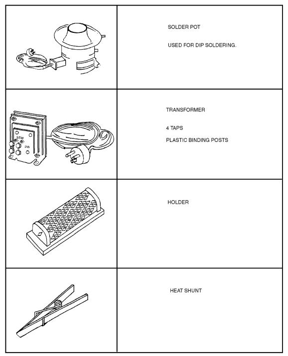
Figure 53-1. Soldering Tools and Accessories (Sheet 3)
