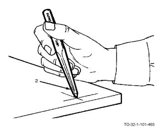
b. Hold the punch (2) over the mark. Tilt it so that you can align the tip with the center of the "X".
