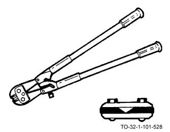
The cutting edges of the clipper cut cutter are in line with the handles and beveled almost entirely from one side. These cutters
