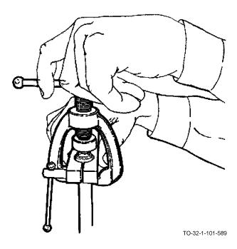
f. When desired flare is reached, unscrew feed screw, and remove yoke from die block clamp.
