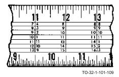
The essex board measure is used to compute the number of board feet in a given piece of lumber.
