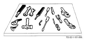
2.2.5 Keep Your Tools Within Easy Reach and Where They Cannot Fall on the Floor or on Machinery. Avoid placing tools anywhere above machinery or electrical apparatus. Serious damage will result if the tool falls into the machinery after the equipment is turned on or running.
