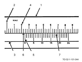
The steel rule (1) is divided into centimeters (cm) (2) and the longest lines represent 10 mm each. Each millimeter is divided into quarters. The vernier scale (3) is divided into 25 parts and is numbered 0, 5, 10, 15, 20 and 25.
