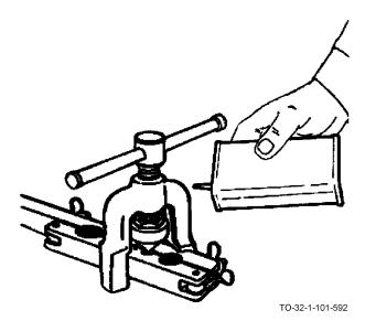
Keep surfaces clean and lightly oiled. Close single flaring tools and tighten cone into block for storing. Keep double flaring tools in the case when not in use.
