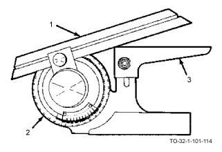
The bevel protractor is made up of an adjustable blade (1) and a graduated dial (2) which contains a vernier scale. The bevel protractor is used to establish an angle and determine its relationship to other surfaces. The acute angle attachment (3) is used for measuring acute angles accurately.
