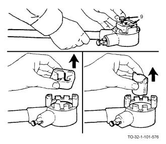
p. Disassemble the die from the ratchet handle as shown, by removing locking screws (9). Remove die and collar from ratchet head.
