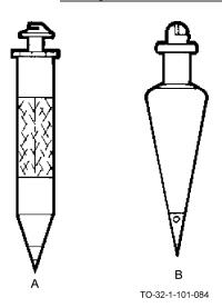
The surveyor's brass plumb bob may be either a spool type (A) or an adjustable cap type (B). Both types have replaceable steel points for increased accuracy. The adjustable cap allows the operator to make minor corrections to height and rotation to make sure the bob hangs straight. The surveyor's brass plumb bob comes with a minimum of 7 feet of nylon, silk or linen cord. It comes in 6, 8, 10, and 16 ounce sizes. The heavier plumb bobs are better for use in windy areas.
