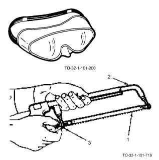
a. Insert the correct blade (1) in the hacksaw frame (2) and adjust wing nut (3) for proper tension.
