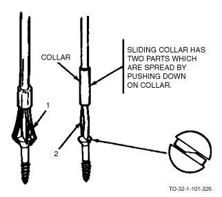
Some common screwdrivers have a screw-holding feature. These are used for working in close quarters, overhead, and hard to reach places. The two most common types are the clip (1) and sliding collar (2). After the screw has been firmly started, switch to a conventional screwdriver to complete the job.
