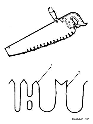
The one-man crosscut saw is about 36 inches long and has a handle at one end. This type of saw is characterized by a highgrade steel blade with two types of teeth known as "cutters (1) and "rakers" (2). The cutters do the cutting, and the rakers chisel out and remove chips from the cut. It is used for heavy work such as cutting down trees and sawing heavy timbers.
