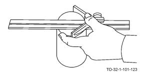
b. Put the center head flush against the cylinder.
