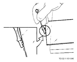
j. Remaining chips may be removed by applying a downward twisting motion using the notches of the cutter.
