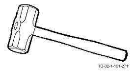
The club hammer is a heavy double-faced demolition hammer. It is primarily used to break up masonry.
