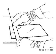
c. Place a straight edge (2) along line to be cut. A wooden yardstick should be used when available, since wood will not slip easily on glass. The cutter will cut 1/16 inch from your mark, so adjust your guide before cutting.
