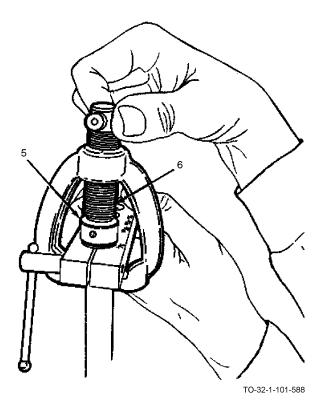
e. Tighten feed screw (6), forcing the tip (5) into the tubing and forcing the tubing into the chamber of the die block clamp.
