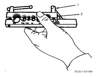
a. Loosen die block clamp screws (1), and open die block clamp (2).
