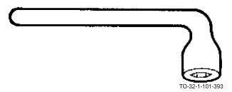
The 90 degree offset handle socket wrench has a fixed socket at the end of a bent handle. It is used for removing and/or installing a nut or bolt which may not be reached with a box or combination wrench.
