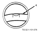
Some levels have a bent tube (4) which allows the bubble to settle quickly.
