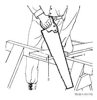
a. In using the crosscut saw, place the work on a level just below the knees. Place one sawhorse, bench or other support (1) fairly close to line of cut (2).
