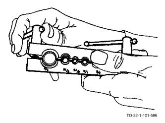
c. Hold tubing so there is about 1/8 inch extending above die block clamp, and tighten die block clamp screws.
