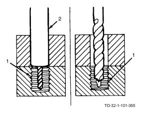
a. Drill a hole in the broken screw (1). Use a drill size guide (2) if available. If one is not available, drill the hole slightly smaller than the diameter of the extractor. (When drilling larger screws it may be necessary to drill a small pilot hole first, then a larger hole).
