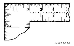
The octagon or eight square scale is used for cutting an octagon from a square piece of material. The back side contains the hundredths scale and is divided into tenths, twelfths, and sixteenths as shown. There are two tables down the center.
