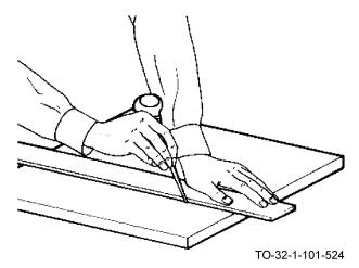
c. Hold straight edge firmly. Hold the awl like a pencil and scribe a line along the straight edge.
