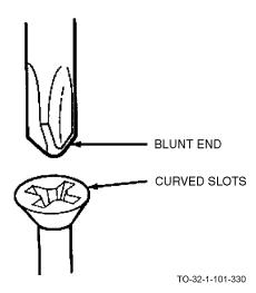
The tip of a cross-tip screwdriver is shaped like a cross so that it fits into cross-tip screws. Cross-tip screws have two slots which cross at the center. These screwdrivers are made with four different sized tips. Cross-tip screwdrivers also have different length blades ranging from 1 inch to 8 inches.
