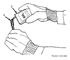
d. Apply a drop of light machine oil (3) to the cutting blade (4).
