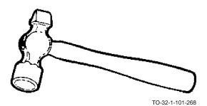
A straight peen hammer is used like the cross peen but differs from the cross peen since its peening edge is turned ninety degrees. This keeps the handle parallel to the struck surface.
