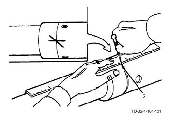
c. Scribe the line by drawing the scriber (2) along the straight edge at a 45 degree angle and tipped in the direction it is being moved.
