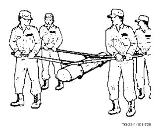
Lifting and moving heavy log with peavies.
