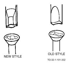
Clutch head screwdrivers are used to drive clutch-bit screws. These screws have recessed heads and are commonly called butterfly or figure-eight screws. There are two styles of clutch heads, old style and new style.
