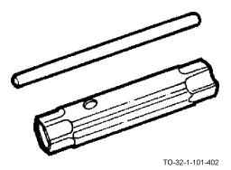
Socket-type plug wrenches are usually combined in sets with an assortment of handles. The set will contain several sizes.
