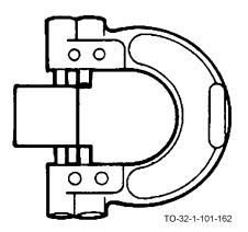
c. If the part is within limits, the NO GO pins will stop the part.
