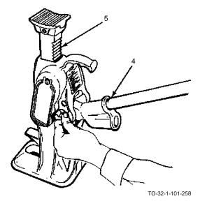
b. To raise a load, pull reversing lever up and toward the operator and operate the lever (4). The jack will raise the load one notch for each lever downstroke. The rack (5) cannot be ratcheted out of the base, as it is designed to stop when raised to its top limit.
