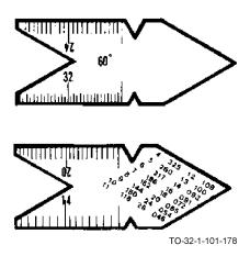
The center gage is graduated in 14ths, 20ths, 24ths, and 32nds of an inch. The back of the center gage has a table giving the double depth of thread in thousandths of an inch for each pitch. This information is useful in determining the size of tap drills. Sixty-degree angles in the shape of the gage are used for checking Unified and American threads as well as for older American National or U.S. Standard threads and for checking thread cutting tools.
