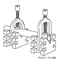
The V-block and clamp assembly consists of a V-shaped, hardened steel body to support round, square, or rectangular shaped work. A clamp (or clamps) holds the work firmly in the body groove. V-blocks and clamps are especially used for grinding, milling, or drilling purposes. Various styles and designs of V-blocks and clamps are available depending on application.
