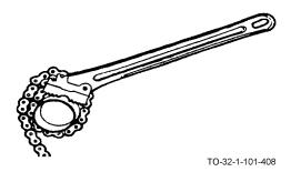
Chain pipe wrenches have a section of bicycle-type chain permanently attached to the handle. The upper section of the head has teeth which mate with the links of the chain. The chain is wrapped around the pipe and pulled over the head section of the wrench to grip the pipe. Chain pipe wrenches will scratch the surface of the pipe.
