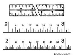
There are many variations of the common rule. Sometimes the graduations are on one side only, sometimes a set of graduations is added across one end for measuring in narrow spaces, and sometimes only the first inch is divided into 64ths, with the remaining inches divided into 32nds and 16ths. A metal or wood folding rule may be used.
