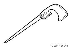
The keyhole saw is the smallest type of nested saw. Its blade has a very narrow point small enough to enter a 1/4 inch hole. It is used for close-quarter work, such as cutting, shaping, or enlarging holes in a board.
