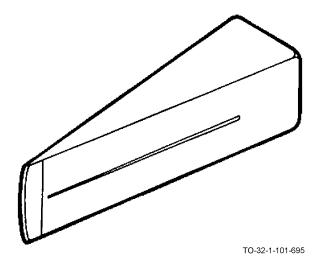
The timber wedge is used with a sledge, primarily to split logs and timber. When sawing timber or thick lumber, it may also be used to spread the cut so the saw will not bind. The timber wedge is a steel tool resembling a slender single-bit ax head. One end is slightly fan-shaped and sharpened to a dull edge. The other end is flat where a sledge can strike when driving the wedge into a log.
