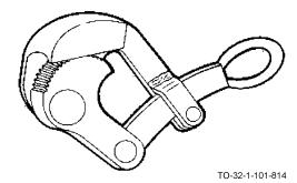
The cable jaw grip is used to tighten or stretch wires or cables for various operations. Examples of application include removing kinks or bends in cables, tightening cables on loads or bales, or for cleaning and oiling of cables. Cable grips, depending on their application, vary in size and design.
