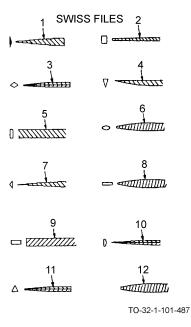
These files are usually supplied in sets. The most common set consists of twelve assorted files in a set which are marking (half-round) (1), square (2), slitting (3), knife (4), joint (round edge) (5), crossing (oval) (6), barrette (7), flat (8), equaling (9), half-round (10), three-square (triangular) (11), and round (12). Swiss pattern files are made in seven cuts. Nos. 00, 0, 1, 2, 3, 4, and 6. They are most often used for fitting parts of delicate mechanisms, and for tool and die work.
