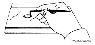
The bent point is used to scribe through holes or other hard to reach places.
