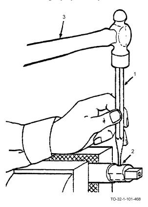
b. Hold punch (1) centered over pin (2). Tap punch lightly with hammer (3). This should move the pin. It may be necessary to apply penetrating oil to the pin before it will move.
