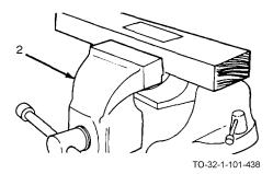
b. Examine the grain of the wood, and place securely in a vise (2) so you are cutting with the grain. The wood should not be able to move in any direction.
