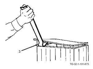
b. Insert the short hooked blade (3) between the boards if greater leverage is required.
