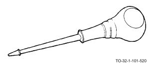
The scratch awl has a fixed tapered blade and a wooden handle. It is used to scribe marks or as a center punch on soft wood and plastics. Cover points when not in use.
