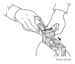
c. Place the plane on the edge of board with the plane pointing across the grain.
