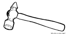
A cross peen hammer is used as a chisel for removing rivet heads and for stretching or bending metal.
