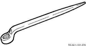
The structural-tapered handle wrench combines a box wrench opening with a tapered shank to produce a box wrench/alignment pin combination. It is usually used on heavy structural construction (bridge girders, building beams, etc.).
