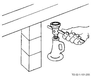
d. Block the load to withdraw the jack.
