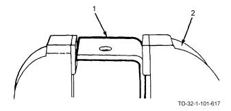
a. Clamp a steel plate (1) securely in a vise (2). Drill and ream a hole of desired size.
