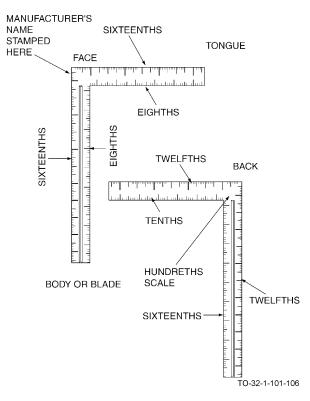
The carpenter's square is made up of two parts: the body or blade, and the tongue. It has inches divided into eighths, tenths, twelfths, and sixteenths. The face side contains the manufacturer's name and the inches are divided into eighths and sixteenths as shown. There are two tables down the center.
