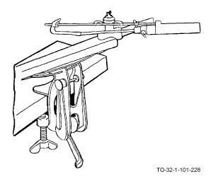
The handsaw filing vise is a special purpose vise used for holding handsaws while they are being sharpened. It has jaws between 9-1/2 and 11 inches wide, and an attachment for holding a file at a constant angle.
