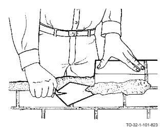
i. Cut off any excess mortar.
