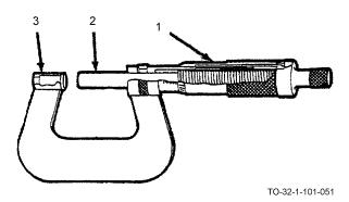
Reading a micrometer is only a matter of reading the micrometer scale or counting the revolutions of the thimble and adding to this any fraction of a revolution. The micrometer screw has 40 threads per inch. This means that one complete and exact revolution of the micrometer screw (1) moves the spindle (2) away from or toward the anvil (3) exactly 1/40 or 0.025 inch.
