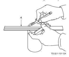
c. Mark the diameter on the cylinder using a pencil or marking crayon by drawing a straight line along the inside edge (4). Make sure the square does not slip while marking.
