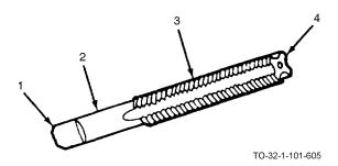
Taps are made of hardened steel and have the following parts: a square end (1), a round shank (2), a body (threaded) section
