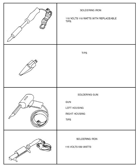
Figure 53-1. Soldering Tools and Accessories (Sheet 2)
