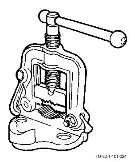
The pipe vise is a special purpose vise designed to hold round stock. It has hinged jaws which allow the user to position the work and then lock it in place. Some pipe vises have a section of chain instead of jaws for holding the pipe. Pipe vises are usually bench mounted. They are used to hold pipe from 1/8 inch to 8 inches in diameter while cutting or threading.
