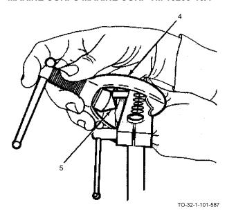
d. Slide yoke (4) over die block clamp, and align the tip (5) over the end of tubing.
