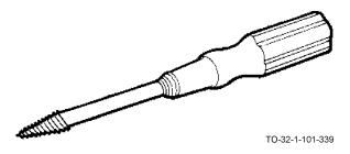
A screw starter or gimlet has a threaded tip. It is used to make a pilot hole in wood for wood screws.
