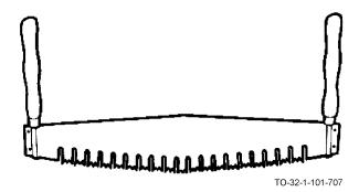
The two-man crosscut saw is 5 to 6-1/2 feet long with a handle at each end. As with the one-man crosscut saw, it also has a high-grade steel blade with the "cutter" and "raker" teeth arrangement. It is used when two men are required for extra heavy cutting jobs.
