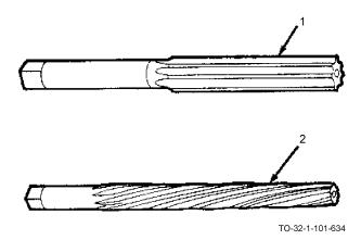
Solid taper-pin reamers are used to finish tapered holes for the insertion of tapered pins or other tapered parts. They are made with a standard taper of 1/4 inch per foot. Solid taper-pin reamers come with straight (1) or spiral flutes (2). Sizes range from 5/0 to 14, with the diameter at the large end ranging from 0.0984 to 1.5412 inches. They also come in sets of 10, sizes 3/0 to 7, and a set of 11, sizes 0 to 10. They are also included in mixed sets of straight and taper-pin reamers.
