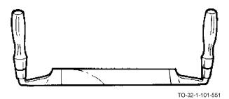
A draw knife is a flat-edged tool used especially on round timber to rough-shape wood. It is used to smooth wood after chopping with a hatchet or axe. It consists of a single bevel blade and two round wooden handles, one at each end and at right angles to the blade. The handles may be adjustable or rigid.
