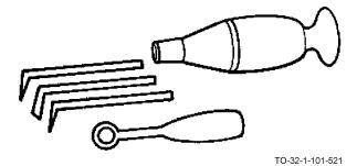
The saddler's sewing and stitching awl has a round wooden handle and interchangeable blades. The awl is used to punch holes in leather and as an aid during sewing. Cover points when not in use.
