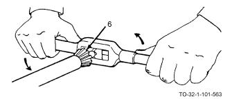
i. Remove the burr from the inside of the pipe with a pipe reamer (6). (See Chapter 39 for care and use of pipe reamers.)
