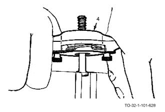
i. Carefully back the diestock (4) off the threads by turning in a counterclockwise direction.
