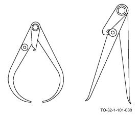
Transfer calipers are used for measuring chamfered grooves or flanges. A screw attaches a small auxiliary leaf to one of the legs. The measurement is made as with ordinary calipers. The leaf is locked to the leg. The legs may be opened or closed as needed to clear the obstruction. The legs are then brought back and locked to the leaf, restoring them to the original setting.
