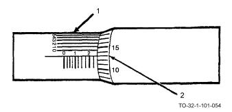
The ten spaces on the vernier (1) are equivalent to 9 spaces on the thimble (2). Therefore, each unit on the vernier scale is equal to 0.0009 inch and the difference between the sizes of the units on each scale is 0.0001 inch.
