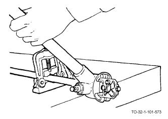
1. After two more turns on the die, back off one turn and apply a coat of cutting oil.
