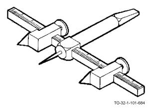
The bit brace circle gasket cutter adjusts from 1 to 5-1/2 inches in diameter. It cuts metal, plastic, wood, hardwood and other materials. It has a tapered square shank to fit a bit brace. It comes with a 3/16 inch tool steel bit, 1/4 inch pilot drill, and a hexagon wrench for easy adjustment.
