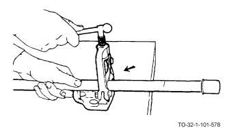
r. Place cap, if available, over threads and remove the pipe from the vise.
