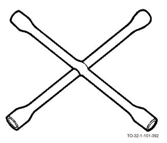
The four-way socket wrench has four non-removable sockets attached to four arms. Each of the sockets is a different size. The four-way socket wrench is usually used to remove or install the wheel stud nuts of a vehicle. The handle construction provides extra leverage when loosening and tightening the stud nuts.
