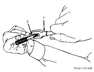
b. Using a tap wrench (1), tighten the handle to the square end of the reamer shank (2).
