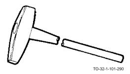
The railroad track maul has a flat faced tapered head which weighs about 10 pounds. They are used for driving railroad track spikes.
