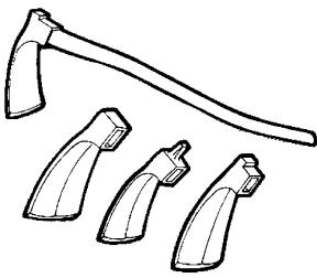
The adz is a chopping tool used for chopping and smoothing lumber or logs where a great deal of wood or bark is to be removed. The adz is a form of ax where the edge of the blade is at a right angle to the handle. It has a curved steel head attached to a curved handle.
