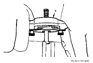
h. Turn the diestock (4) one turn forward and one-quarter turn backward. Repeat this procedure until desired thread length has been cut.
