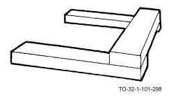
a. Lay two pieces of wood parallel to each other. Place a third piece on top and align so that the edges are even.
