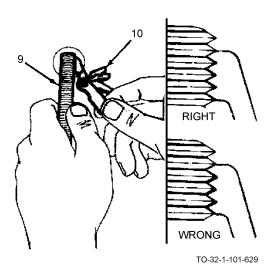
j. Clean threads (9) with a clean rag and check with a screw pitch gage (10) before using.
