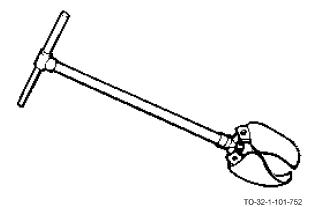
The posthole auger is a long tool made up of a steel shaft that has two shovel-like blades at one end. The blades have curved faces which are hinged to permit slight movement with the concave surfaces of these blades facing each other. The posthole auger is used to bore holes in the ground for posts, poles and explosive charges.
