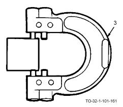
b. Using a slight hand pressure, push the gage (3) over the part.
