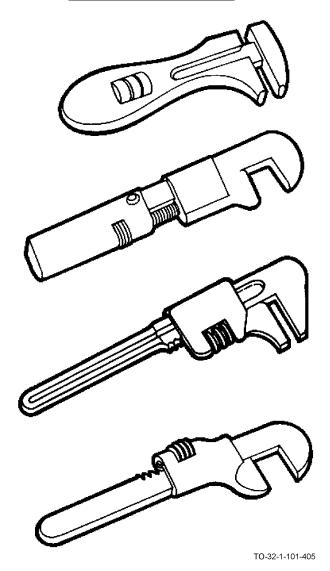
The monkey and auto wrenches are similar and have one fixed jaw and an adjustable jaw which moves along the handle by turning a knurled worm gear. Monkey and auto wrenches are used to install or remove odd size nuts and bolts. An adjustable wrench must be used with care. Always apply pressure against the fixed jaw.
