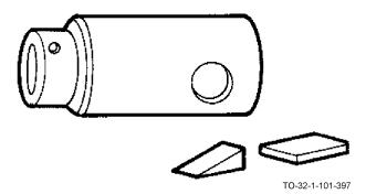
Wedge-type stud removers are made of a socket housing and two metal wedges. The socket is placed over the stud to be removed and the wedges are driven into the socket to hold the stud. The socket housing is now turned with a handle to remove the stud.
