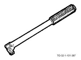
A hinged handle has a hinged adapter on one end which may be rotated in 90 degree steps. The hinged handle is used when additional leverage or torque is needed to loosen nuts or bolts.
