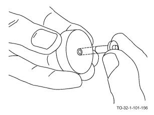
c. After checking the part in the GO gage, check it in the NO GO gage. The stud must not enter this gage to establish it as being between the desired limits.
