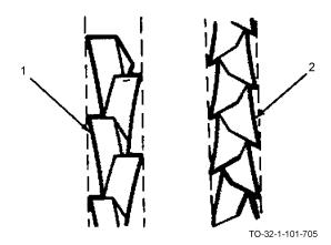
The handsaw consists of a thin flat blade with teeth and a wooden or plastic handle, called the heel, fastened to the end of the blade by screws. There are two categories of handsaws: the ripsaw (1) and the crosscut (2). The ripsaw is designed to cut with the grain of wood, and the crosscut saw is designed to cut against the grain. The handsaw is used in carpentry, roughout work, and for "finish" hand sawing. Sizes of handsaws vary depending on design and nature of the task.
