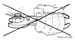
2.2.4 <u>Use Each Tool Only on the Job for Which it was Designed</u>. If you use the wrong tool to make an adjustment, the result will probably be unsatisfactory. For example, if you use a socket wrench that is too big, you will round off the corners of the wrench or nut. If this rounded wrench or nut is not replaced immediately, the safety of your equipment may be endangered in an emergency.
