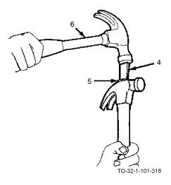
d. Drive wooden wedge (4) in handle face (5) with hammer (6).
