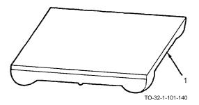
A surface plate provides a true, smooth, plane surface. It is often used as a level base for surface and height gages from which to make accurate measurements. Surface plates are usually made of close grained cast iron (1), are rectangular in shape, and come in a variety of sizes.
