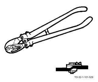
Shear cut, flat bar, and strip cutters are used to cut flat-soft, medium-hard bar, and strip stock. The cutting edges of the jaws pass each other in the manner of scissors, making a complete shear cut. The cutting capacities range from  $7/8 \times 5/32$  inch to  $1-1/2 \times 9/32$  inch for soft and medium steel, and from  $3/4 \times 1/8$  to  $1-7/16 \times 1/4$  inch for hard steel. The handles range from 14 inch to 36 inch lengths.
