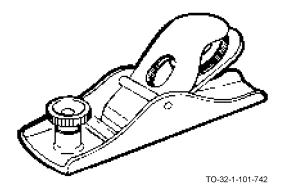
The block plane is the smallest type of plane. It is available in a variety of patterns and is designed to cut end grain with the cutting blade set between 12 degrees and 20 degrees. Although it can usually be used with one hand, a toe knob is provided when additional pressure is needed.
