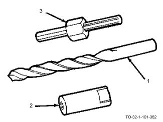
The straight-flute type requires the following tools to drill a pilot hole in the screw: a twist drill (1), a drill guide (2), and a turn nut (3).
