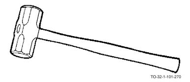
A double face sledge hammer has similar faces on both sides of the head.
