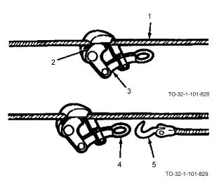
b. Fasten eye (4) to tension puller hook (5).
