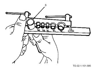
b. Insert tubing to be flared (3) into die block clamp.
