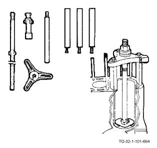
The universal cylinder sleeve is used to pull cylinder sleeves from engine blocks. It is adjustable to provide clearance regardless of the position of the cylinder studs and to simplify centering the tool over the bore. This puller is used in conjunction with four adapter plates supplied with the puller. The combination is capable of pulling cylinder sleeves 4-1/4, 4-1/2, 4-3/4, and 5-3/4 inches in diameter.
