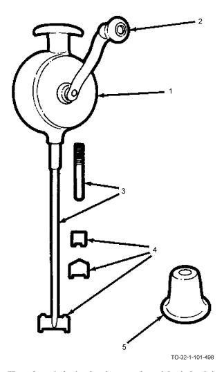
The valve grinder is a hand-operated special grinder. It is used for grinding the valve seating surfaces on combustion engines. It grinds with cutting blades on a rotating shaft instead of an abrasive wheel. It consists of an encased gear housing (1), a handcrank (2), interchangeable shafts (3), cutting blades (4), and a suction cup (5). The suction cup is used in place of a blade to grind non-slotted valves to fit seating surfaces.
