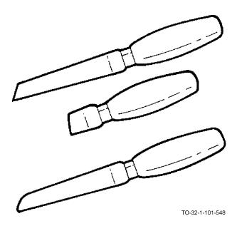
Rubber cutting knives come in a variety of styles and shapes. Some taper to a blunt round point. Some have a short, wide blade. Others have a long, wide hollow ground blade. The handle is usually oval in shape.
