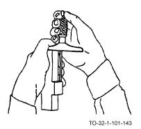
Measuring projection depth with micrometer precision.
