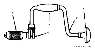
The brace drill is made up of the following parts: head (1), crank (2), crank handle (3), ratchet mechanism (4), and chuck (5). The brace is used to drill holes in wood and with a screwdriver bit, remove and install screws.
