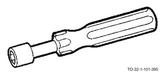
The screwdriver-type socket wrench has a socket fixed on the bottom of a screwdriver handle. They are used to remove and/or install small nuts and bolts. Stud removers may be either the cam-operated type or the wedge type. They are used to remove studs from their seats for replacement. A single stud remover can be adjusted to remove different size studs.
