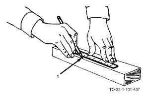
a. With rule and pencil, mark area (1) to be cut with the chisel.
