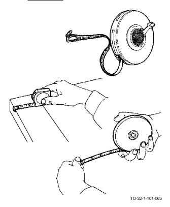
Steel tapes are made from 6 to about 300 feet in length. The shorter tapes are made with a curved, but rigid, cross section flexible enough to be rolled up. Long, flat tapes need support over their full length to avoid sagging. Lack of support can cause reading errors. The most common types of steel tapes have a hook at one end to let one person take all the readings.
