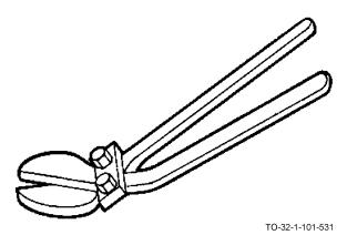
Angular cut cutters have the cutting edges offset 30 degrees from the handles. This is so the user can keep the work in sight. It is used for close cutting of soft or medium-hard metals. Cutting capacities range from 1/4 inch to 1/2 inch for medium steel. The handles range from 14 inches to 36 inches in length.
