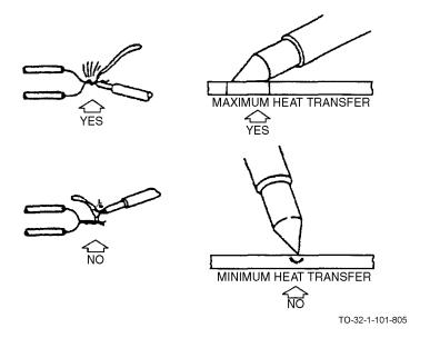
Figure 53-2. Using the Soldering Iron
