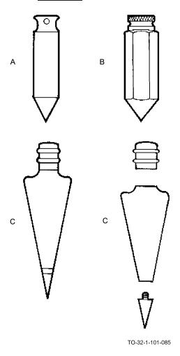
The solid steel plumb bob (A) may have a machined integral head, body, and point. It may have just a removable head (B), or a removable head and a replaceable point (C). It may be round or hexagonagonal in shape and it comes in 3, 8, and 12 ounce sizes. Cord for the solid steel bobs must be obtained from a separate source. This type plumb bob is used when extreme accuracy is not required.
