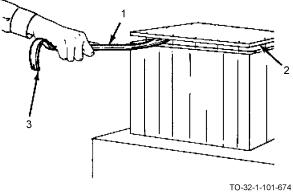
a. Insert the long tapered blade (1) between boards (2) to be removed or ripped. Then exert leverage on the short hooked blade (3) of the bar to pry the boards loose.
