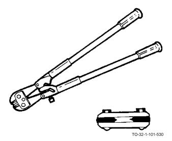
The side nut splitter cutter has the edge of the cutting jaws in line with the handles. When adjusted properly, the cutting edges will remain separated after the nut is split. This tool is used to split nuts off bolts, with the tool "head on" to the bolt, without damaging the bolt. Cutting capacity is rated for a 3/8 inch bolt nut and is adjustable to 5/16 inch and 1/4 inch capacity. The handle is 24 inches long.
