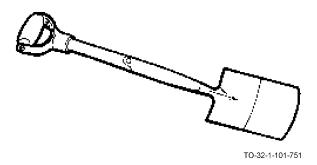
The spade, like the shovel, has a steel blade a wooden handle. The blade may be rounded, pointed or square in shape and the handle may have the D or T-shaped handgrip. The spade is used for heavy digging or in confined areas.
