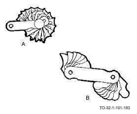
The blades of fillet and radius gages are made of hard-rolled steel. The double-ended blades of the gage have a lock which holds the blades in position. The inside and outside radii are on one blade on gage (A). The other gage (B) has separate blades for inside and outside measurements. Each blade of each gage is marked in 64ths. Each gage has 16 blades.
