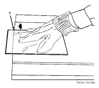
h. To part the glass, slide the pane of glass so the scored groove (6) is about 1/8 inch beyond the table edge.
