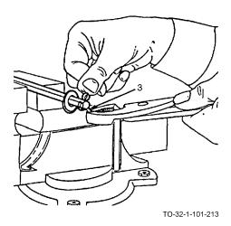
b. Grasp the other section of the extending cotter pin (3) and bend it back flat against the metal surface or nut.
