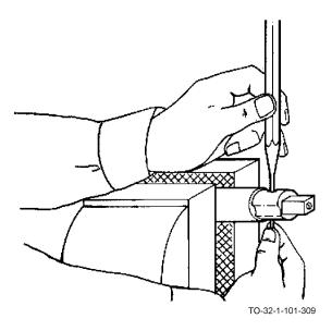
c. Catch the pin in your right hand before it falls out of the shaft.
