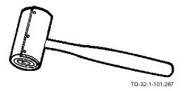
The rawhide mallet has a cylindrical head which is made by tightly wrapping and staking a sheet of leather. It is used for forming and shaping sheet metal.
