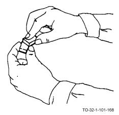
a. Bring the blocks together flat and move them slightly back and forth. This minimizes scratching, as it will detect any foreign particles between the surfaces.
