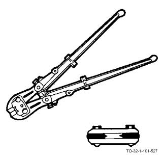
The center cut cutter is used for all general-purpose cutting. The cutting jaws are firmly fixed in line with the handles. The cutting edges are in the center of the jaw between equal levels. The longer the handle, the greater the cutting capacity. The cutting capacities range from 3/16 inch to 1/2 inch for medium steel, and from 5/16 inch to 11/16 inch for soft steel. The handles range from 14 inch to 42 inch lengths.
