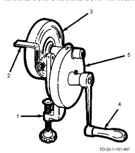
Bench grinders are used for reshaping and sharpening chisels, drills, hatchets, and other similar small hand tools. The bench grinder consists of a clamp (1), a rest (2), an abrasive wheel (3) a handcrank (4), and an encased gearing assembly (5). The clamp is used for fastening the grinder to a working surface. The rest supports tools which are being ground. It is adjustable and may be moved from side to side. The abrasive wheel may be changed depending upon the type of metal being ground.
