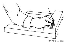
b. Support a common nail (1) between thumb and first finger about halfway up the nail.
