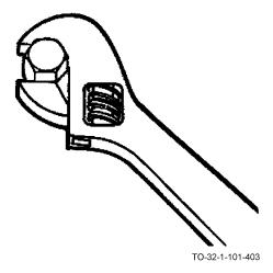
The adjustable open-end wrench has one fixed jaw and a movable or adjustable jaw. The adjustable jaw is set against the face of the nut by turning a knurled worm gear. Care must be exercised when using an adjustable wrench. Always use the fixed jaw for applying pressure to tighten or loosen nuts or bolts. Adjustable wrenches are used to remove and/or install nuts, bolts, and studs when the correct size wrench or socket is not available.
