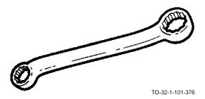
The most common box wrench is the double offset box wrench. It comes with a different size opening at each end. The double offset wrench is used to remove normal nuts and bolts.
