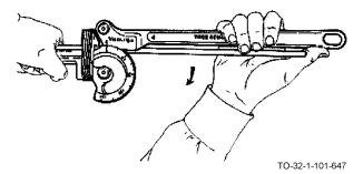
d. Apply downward pressure on the slide bar.
