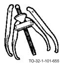
The universal gear puller is usually of yoke and screw construction with two jaws. The jaws have a capacity from 0 to 14
