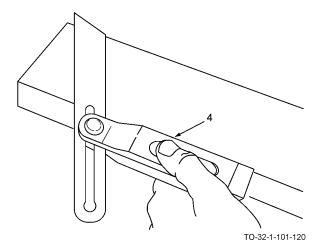
b. The angle may now be laid out by extending the blade across the board with the stock (4) held firmly against the edge.
