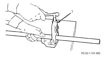
a. Clamp pipe securely in pipe vise (1) with end to be threaded extending beyond the edge of the vise jaws as shown.
