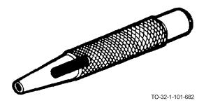
The hollow gasket cutter is also known as a hollow punch. It is extremely serviceable for cutting soft materials. It comes in a set with a mandrel. The sizes are 1/4, 5/16, 3/8, 7/16, 1/2, 9/16, and 5/8 inch. The set will withstand unlimited use if a hardwood block is used under the gasket material when cutting gaskets. They are not designed for cutting metal or cutting against a hard surface. Other individual hollow gasket cutters are also available.
