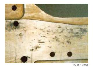
Figure 1-8. Example of Pitting Corrosion
