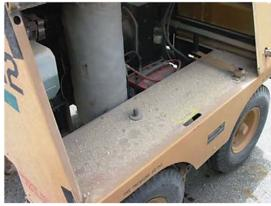
Figure 7-2. Sand/Dust Intrusion
