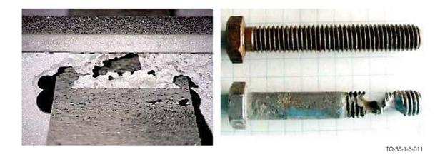
Figure 1-11. Examples of Concentration/Crevice Corrosion
