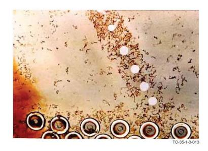
Figure 1-13. Example of Filiform Corrosion
