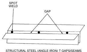
Figure 5-1. Angle Iron Sealant Application
