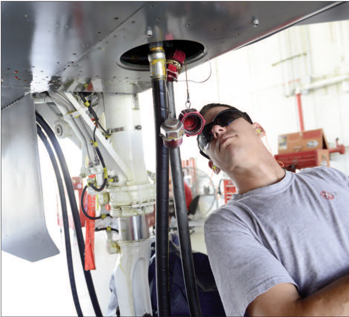
U.S. Air Force photos by TOMMIE HORTON Above, Brent Hunnicutt, 561st Aircraft Maintenance Squadron aircraft mechanic, services the hydraulic reservoir of an F-15-Eagle readying for a functional test flight. During these flights, pilots follow a standard checklist, running through the performance of flight controls, shutting down motors and restarting them, and flying at supersonic speeds.
