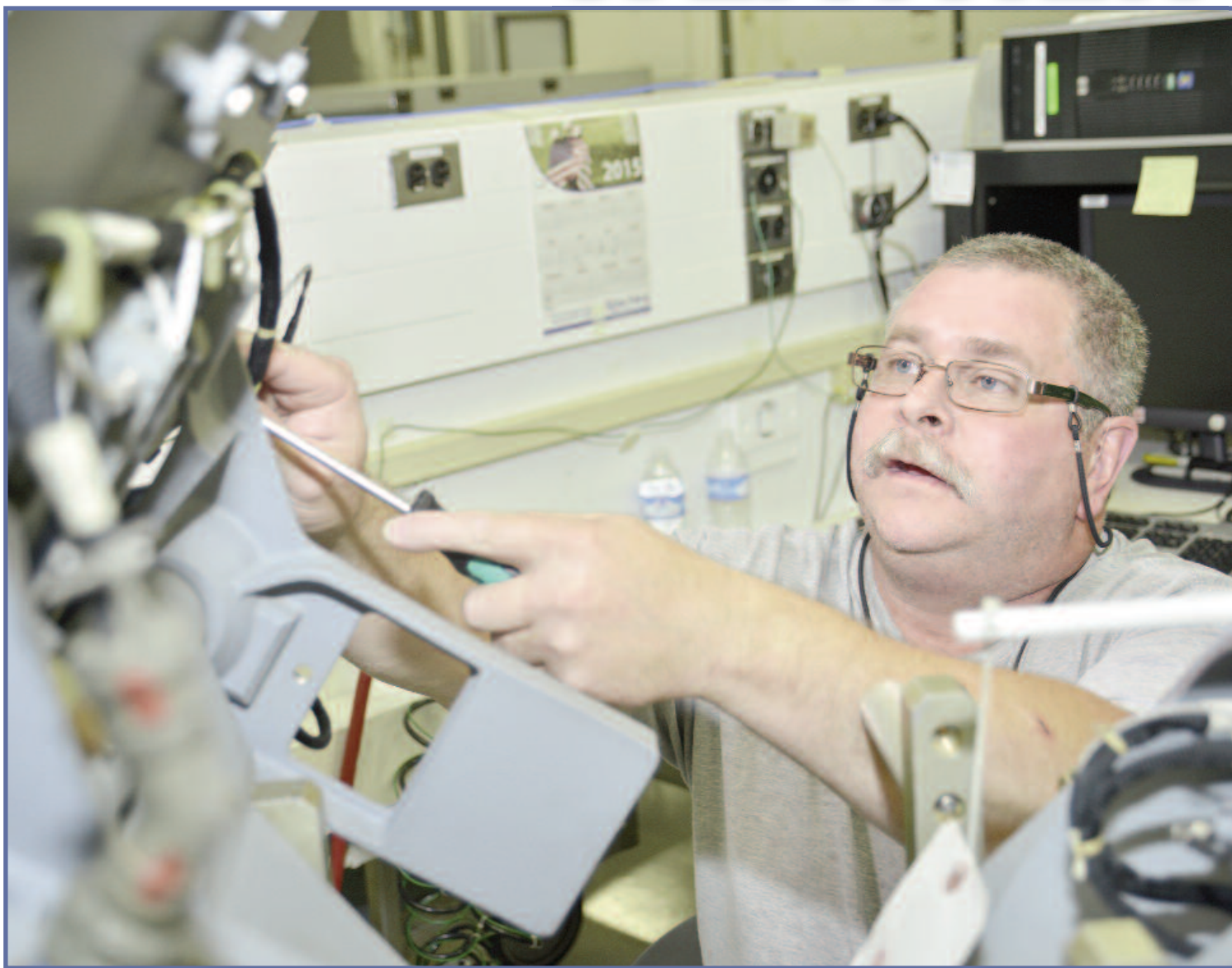
Jack Hancock, 567th Electronics Maintenance Squadron technician, reassembles a radar antenna after he repaired it. Since 2009, the APN-241 Color Weather Radar Shop has been accident free.
