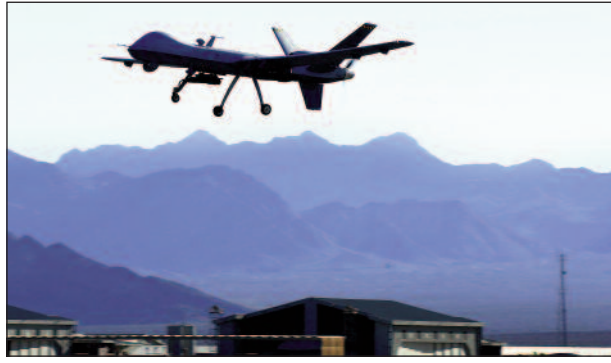
U.S. Air Force photo by SENIOR MASTER SGT. CECILIO RICARDO An MQ-9 Reaper performs touch-and-go flight patterns at Creech Air Force Base, Nev. The Reaper is an armed, multi-mission, medium-altitude, long-endurance remotely piloted aircraft that is employed primarily as an intelligence-collection asset and secondarily against dynamic execution targets.
