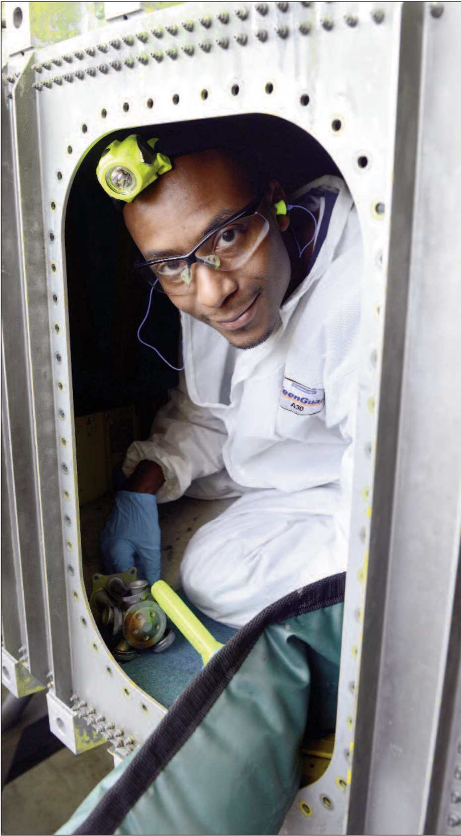
U.S. Air Force photo by TOMMIE HORTON Greg Vickers, 560th Aircraft Maintenance Squadron aircraft mechanic, conducts maintenance inside the confined space of a C-130 fuel tank as part of programmed depot maintenance at the Warner Robins Air Logistics Complex.
