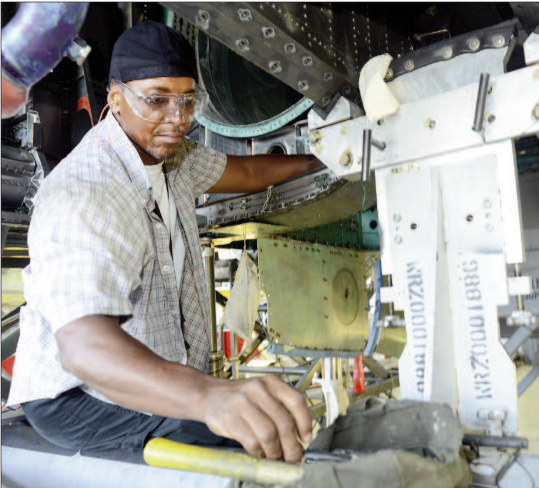
Dennis Pickett, 561st Aircraft Maintenance Squadron aircraft structural repair technician, installs fasteners into the newly replaced 626 bulkhead of an F-15C. During programmed depot maintenance, a crack was discovered in the original bulkhead leaving the organization with the option to replace the part or scrap the entire aircraft.
