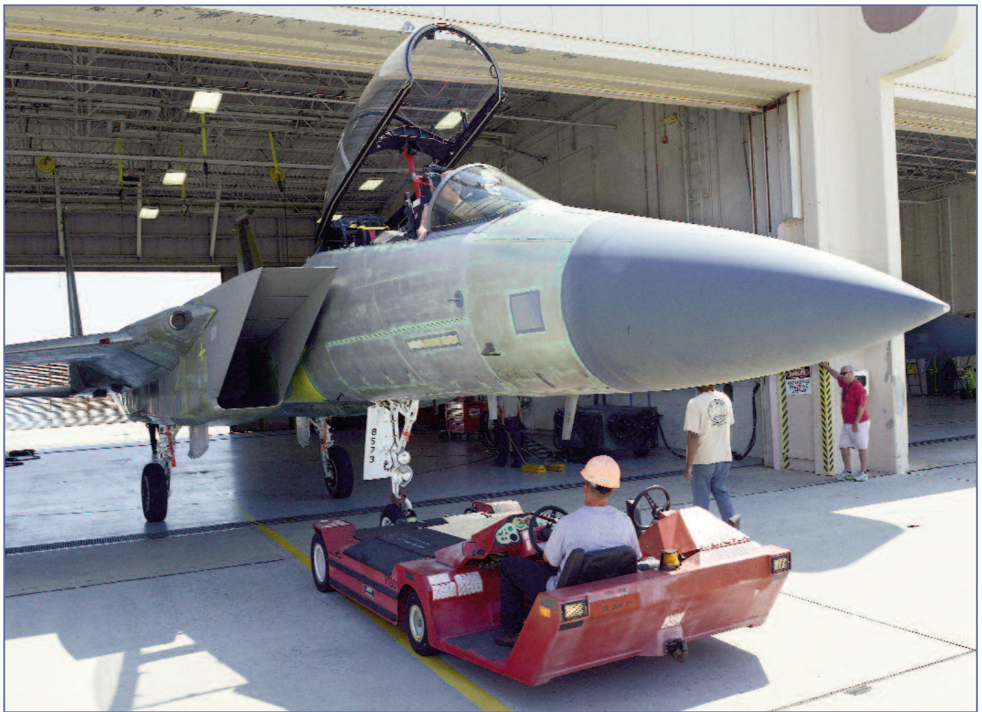
An F-15 is towed to a hangar upon its return from a test flight. During these flights, aircraft are put through extensive testing and engine run-up to find any possible performance problems.
