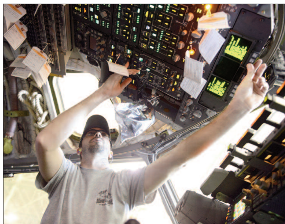
Rob Haymons, 562nd Aircraft Maintenance Group aircraft electrician, performs operational checks of C-17 interior light panels.
