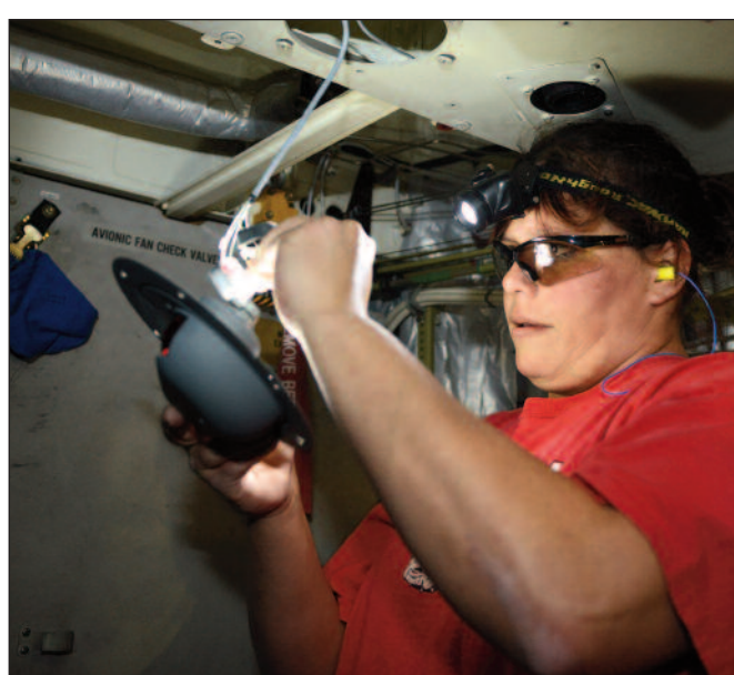
Susan Floyd, 402nd Electronics Maintenance Group electronics mechanic, installs a C-17 forward loadmaster light panel.
