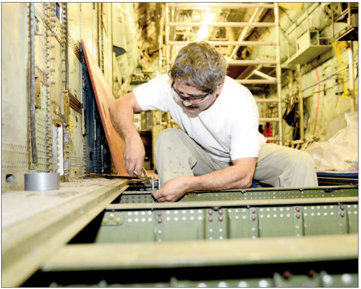
Right, Carlos Melendez, 560th Aircraft Maintenance Squadron sheet metal mechanic, replaces floor boards in the cargo area of a C-130H.
