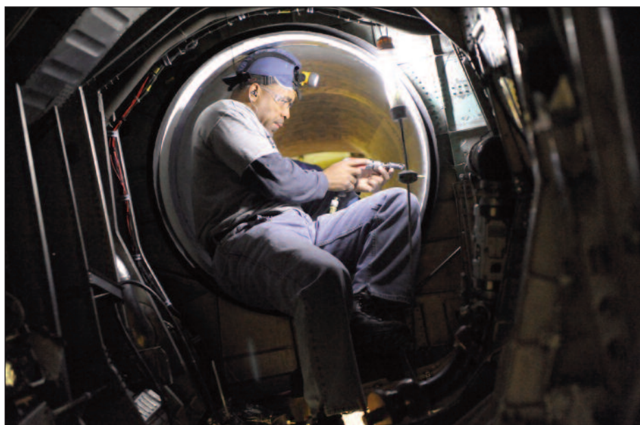
U.S. Air Force photo by RAY CRAYTON Anthony Farrow, 561st Aircraft Maintenance Squadron Production Support, changes intake fasteners on an F-15.
