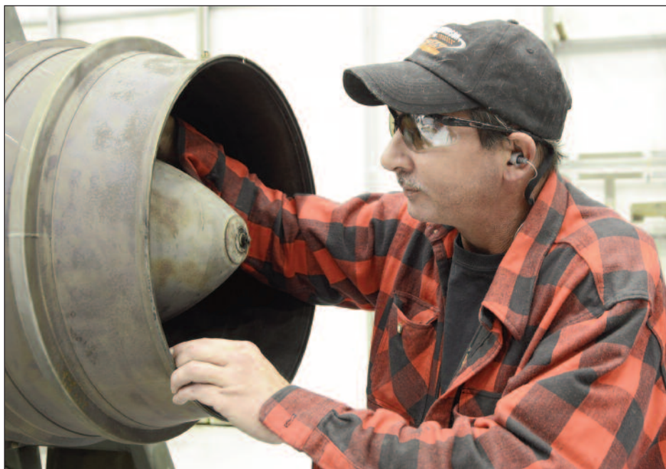
U.S. Air Force photo by ED ASPERA James Skipper, C-130 Engine Shop mechanic, shows a rear bearing support crack on a C-130 engine.
