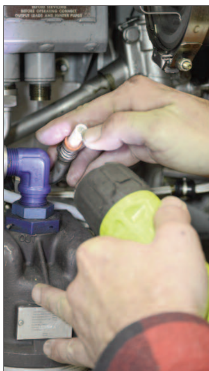
James Skipper, C-130 Engine Shop mechanic, removes an igniter which provides power to a C-130 engine.
