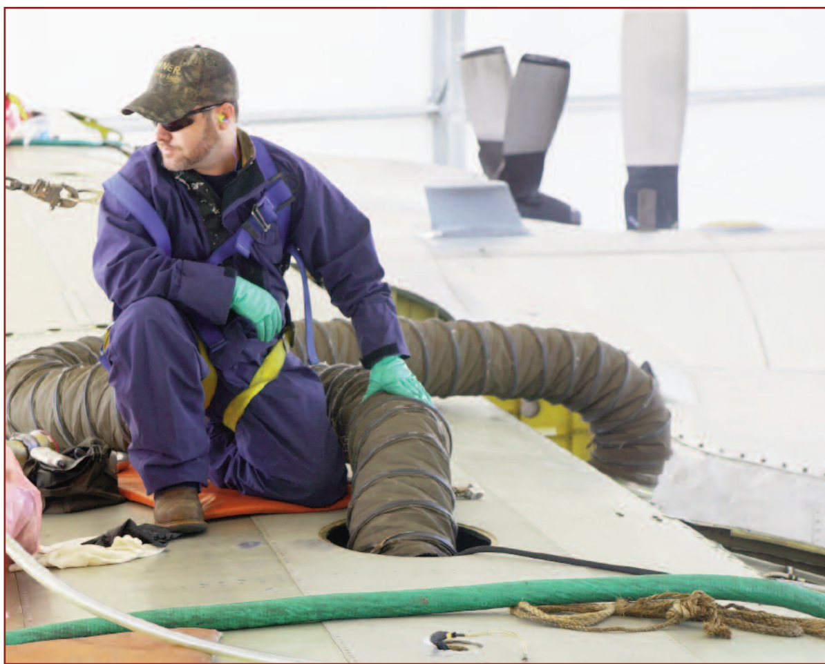
Robert Noles, part of the C-130 strip crew, removes fuel foam from the inside of a right wing cavity. On some areas of the wing, workers are able to open a lid and effortlessly extract the material. But, there are other areas where crews must crawl inside the wing to get the job done.
