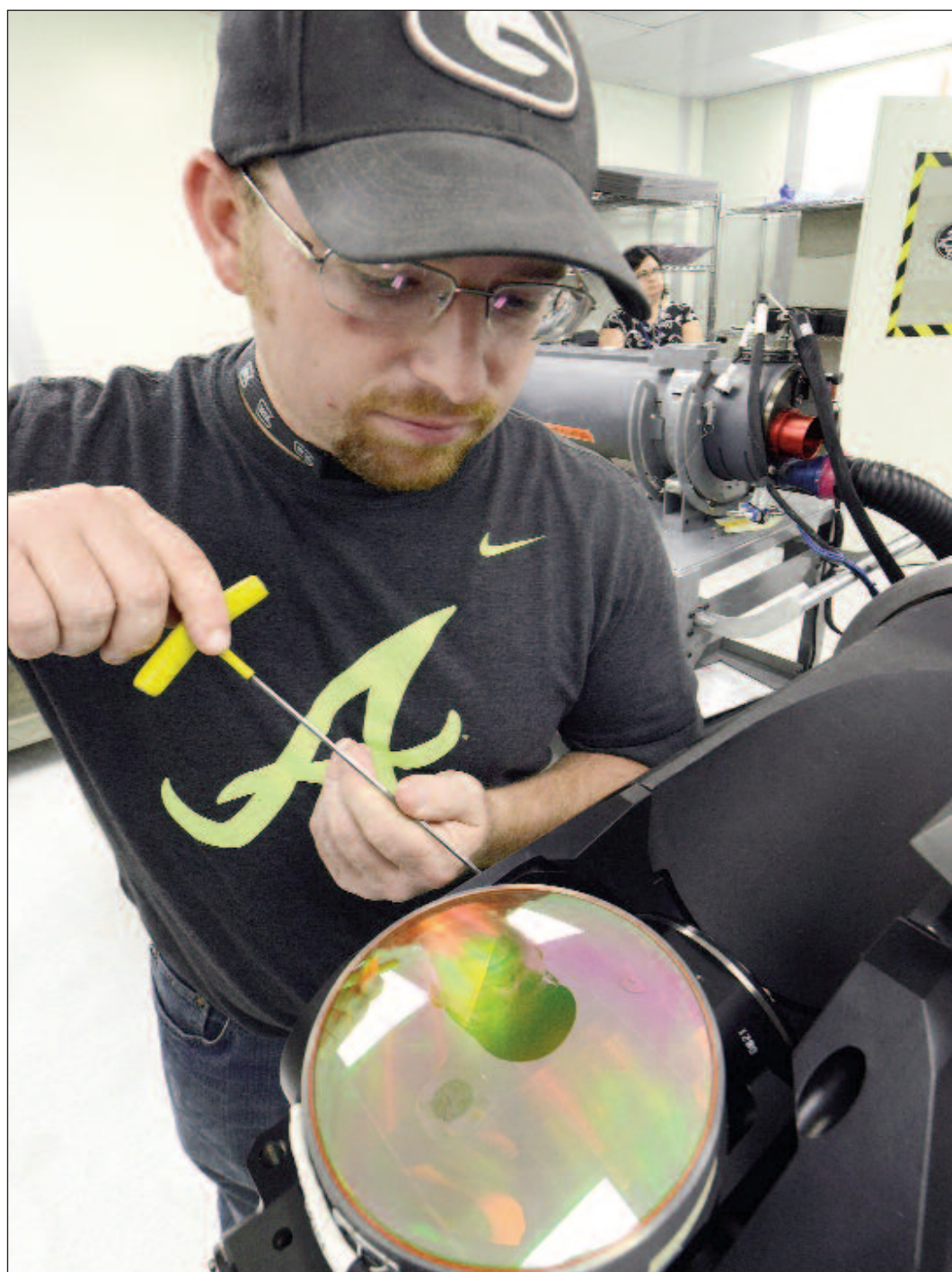
Jeffrey Nauss, 402nd Electronics Maintenance Group electronics technician, performs optic alignment and adjustment procedures on the rotating gimble assembly of a Sniper XR Advanced Targeting Pod.
