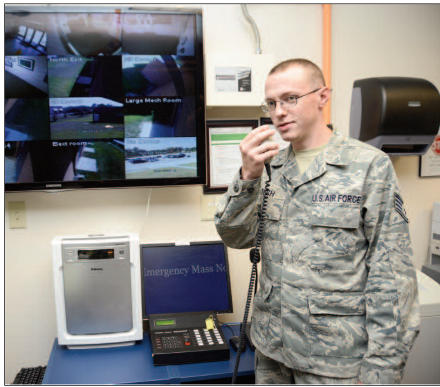
U.S. Air Force photo by ED ASPERA Staff Sgt. Tyler Bush, senior emergency action controller, demonstrates the Giant Voice System. It is a part of the Installation Notification Warning System, which allows controllers to inform the base populace of emergency situations that require immediate action such as alarm conditions, FPCON/INFOCON changes and natural disaster warnings.
