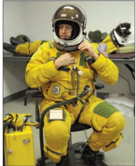
U.S. Air Force photo by RAY CRAYTON Stuart Droce, ER-2 pilot, dons a space pressure suit. These suits can save a pilot's life in case of a loss of cabin pressurization at the aircraft's flying altitude of 65,000 feet.
