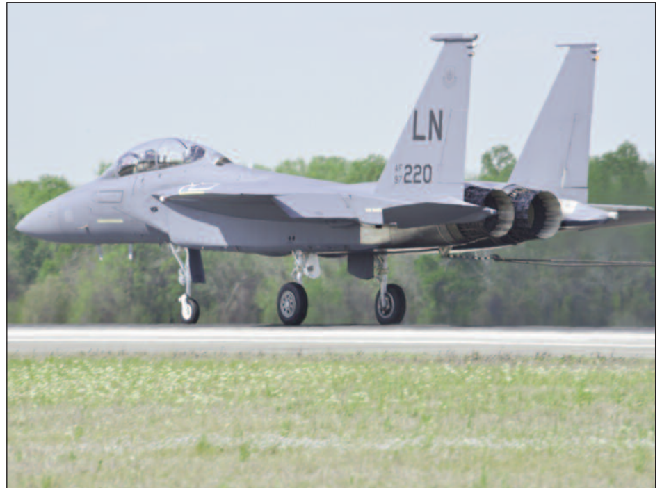
Top, pilots Lt. Col. Stephen D'Amico, F-15 flight commander, and Maj. John Grady, C-5 flight commander, inspect the F-15E following the use of Robins' aircraft barrier arresting system April 8. Above, The F-15E uses a tailhook to catch a cable which runs across the flight line. The F-15E is a two-seat, all-weather, long-range strike and ground attack aircraft.
