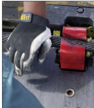
U.S. Air Force photos by ED ASPERA Base firefighters prepare the cable system prior to the F-15 landing at Robins. The use of the system was for a scheduled annual certification engagement April 8.
