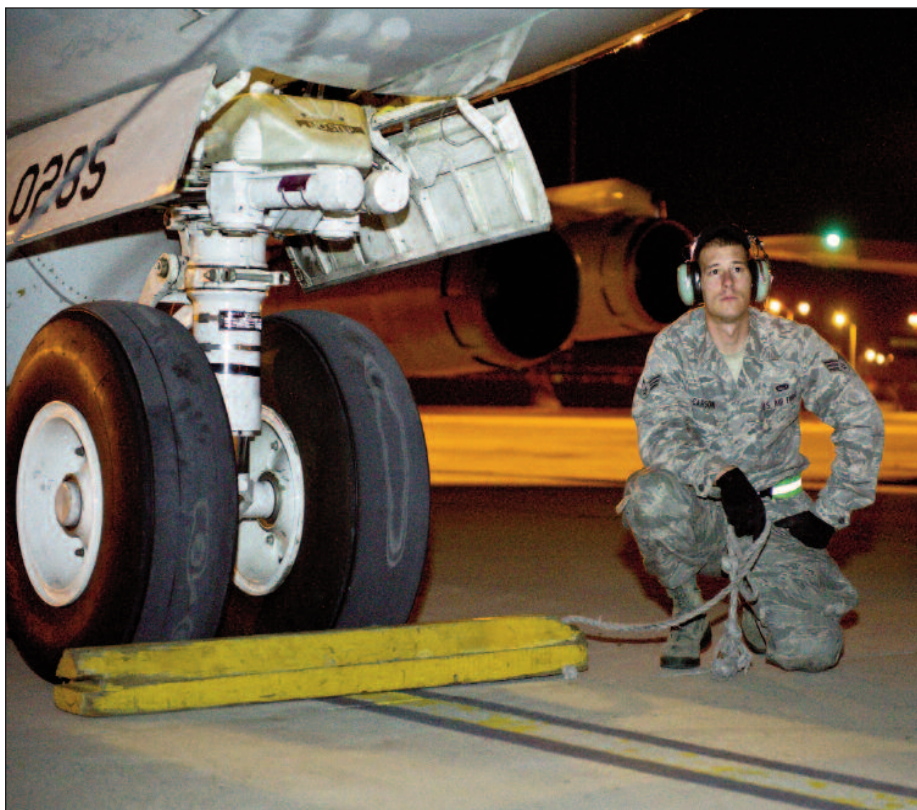
U.S. Air Force file photo by MASTER SGT. ROGER PARSONS Senior Airman Stephen Carson, 461st Air Control Wing, waits for the signal to pull the chocks from the nose gear on an E-8 Joint STARS prior to launch.
