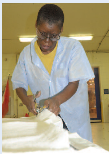
Sandra Armstrong, metal bond sheet metal mechanic, trims breather cloth which creates a vacuum seal bag for the autoclave bonding cycle.
