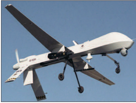
Courtesy photo An MQ-1 Predator armed with an AGM-114 Hellfire missile flies a training mission. The MQ-1's primary mission is interdiction and conducting armed reconnaissance against critical, perishable targets.
