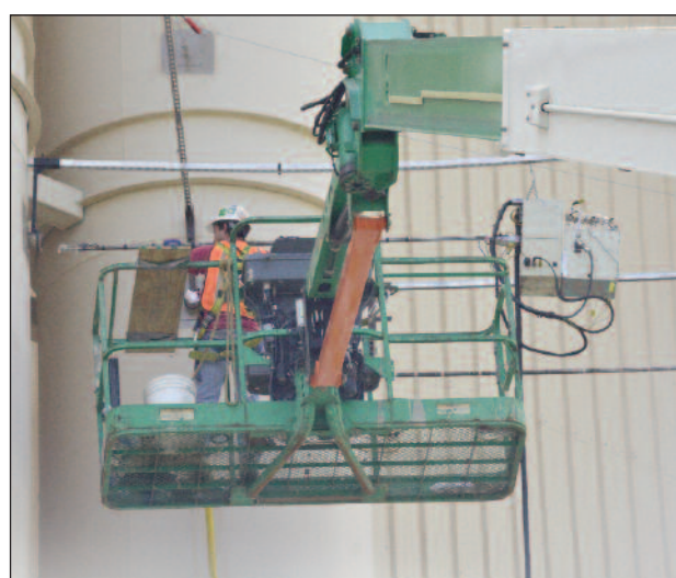
U.S. Air Force photo by ED ASPERA A 78th Civil Engineer Group consultant tests the stack exhaust from the aircraft coating hangar in Bldg. 59 as part of a residual risk and technology review by the Environmental Protection Agency.
