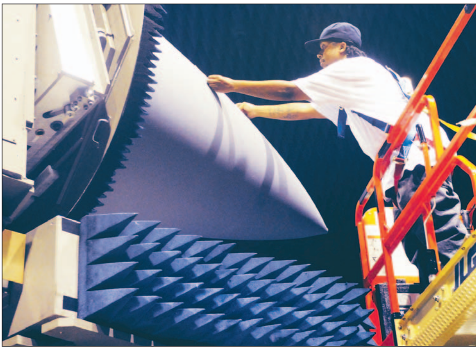
U.S. Air Force photo by SUE SAPP Clarence Thrower, a 566th Electronics Maintenance Squadron employee, makes corrections to a radome by adding tape.
