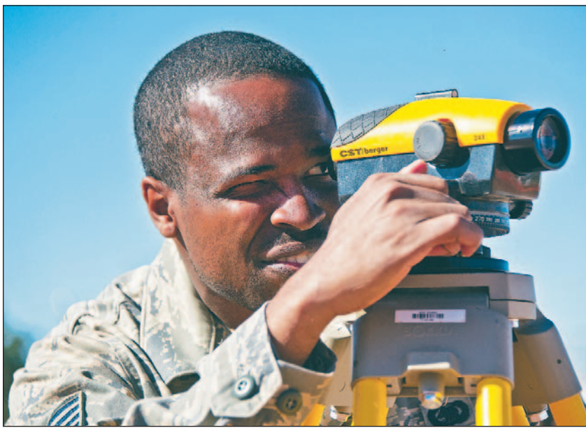
Tech. Sgt. Antonio Adolphues, 116th Civil Engineer Squadron, uses an auto level to take measurements during a construction project at St. Michaels Association for Special Education, Window Rock, Ariz., June 9.
